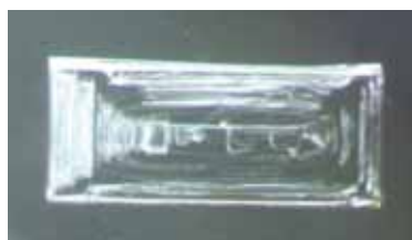
Figure 2-5 Acrylic acid crystal with cavities grown from a melt with 5 wt% water.
