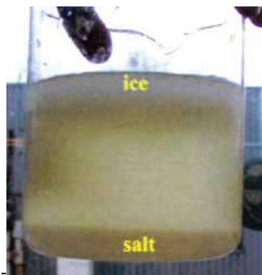
Figure 4-2 Gravitational separation of ice and salt crystals [5].
