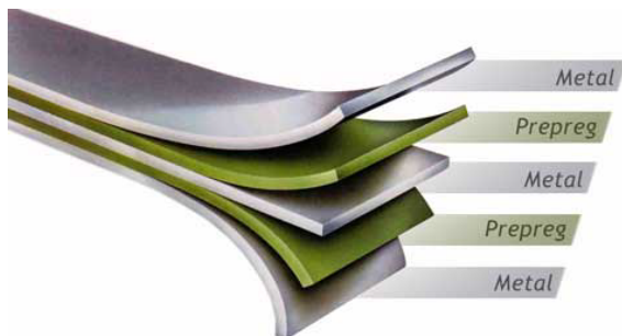
Figure 22.1: Illustration of GLARE lay-up.
