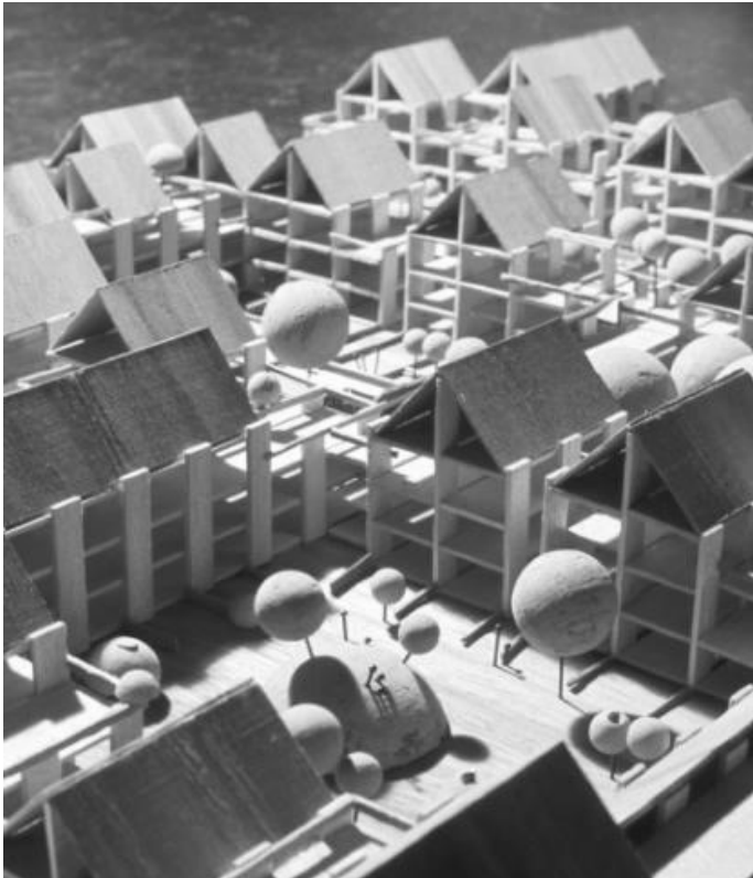
Fig. 3.4: Model photo showing the support structure of Molenvliet. From: The Molenvliet Project , by Frans van der Werf, 2017. https://thematicdesign.org/wp-content/uploads/2017/05/Molenvliet%20for%20Thematicdesign.org%20-new%20main%20text.pdf
