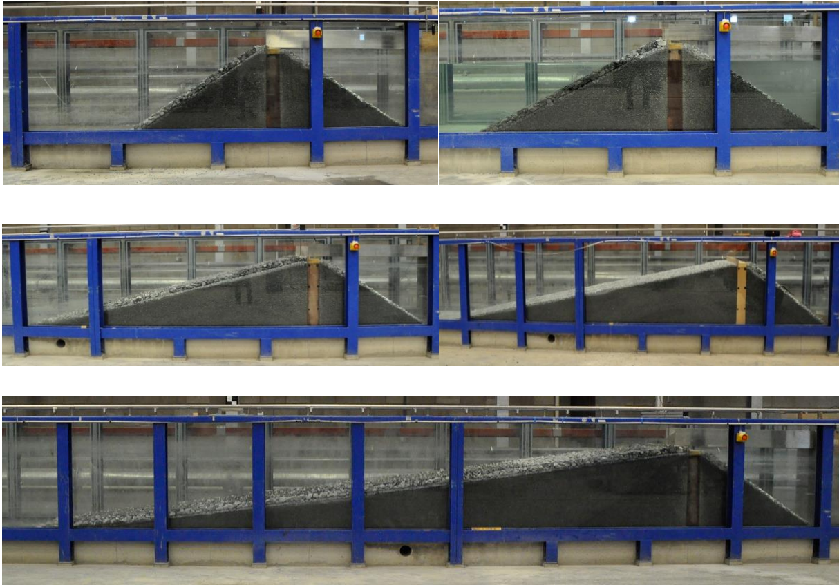
Figure 9 Construction of the different breakwater Configurations. Top left: slope 1:1.5, Top right: slope 1:2, Middle left: slope 1:4, Middle right: slope 1:6, bottom: slope 1:8.
