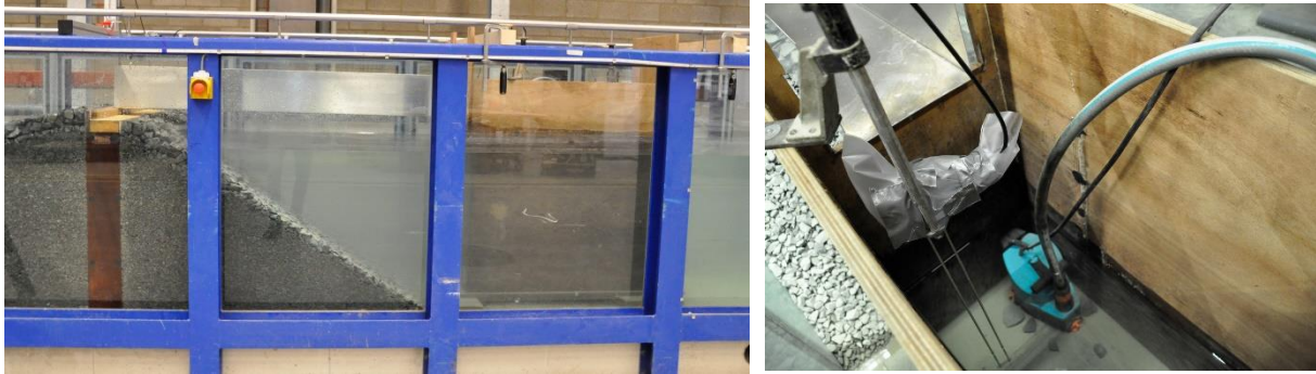
Figure 11 Chute connection between crest element and overtopping box (left) and pump inside overtopping box (right).
