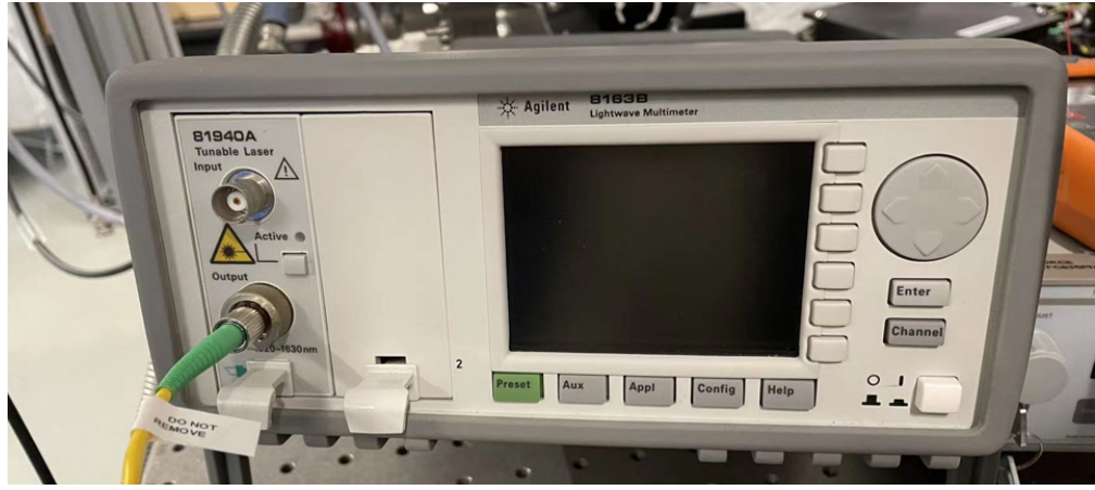
Figure 25: Tunable input laser source with a tunable range of 1530nm to 1620nm.
