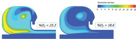
Figure 3 – Damköhler number contours in the mid-plane of the combustor for two different oxidizer compositions. Simulations including radiation modelling.
