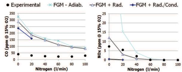
Figure 5 –CO and NO<sub>x</sub> emissions as function of nitrogen addition in the oxidizer stream.
