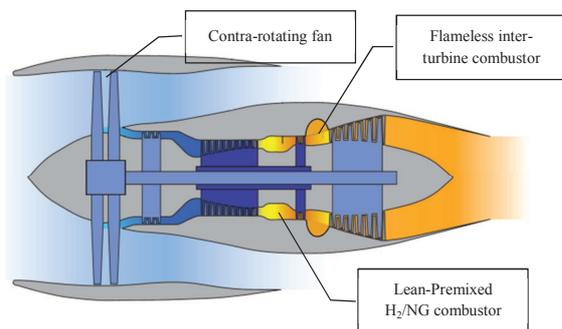
Figure 1 – Engine concept proposed along the AHEAD project<sup>1</sup>.
