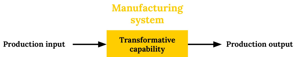
Figure 4.1: Input-output representation of a manufacturing system
