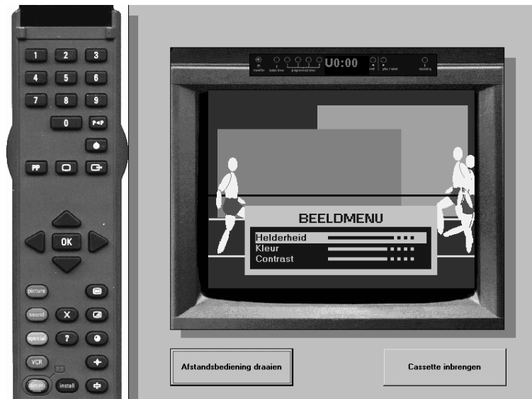
Figure 5 The software prototype (showing the picture menu). Both TV/video recorder and remote control are shown on the computer screen. The large buttons along the lower edge of the screen are named 'Turn over remote control' and 'Insert cassette'.
