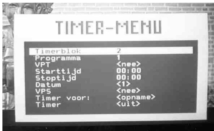
Figure 3 The timer menu. Listed items are: Timer block, Channel, VPT <no>, Start time, Stop time, Date, VPS <no>, Timer for <recording>, Timer <off>.
