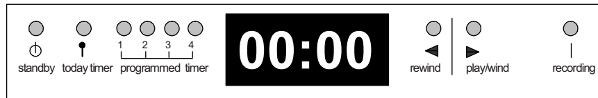
Figure 2 Schematic view of the LEDs and labels above the screen.
