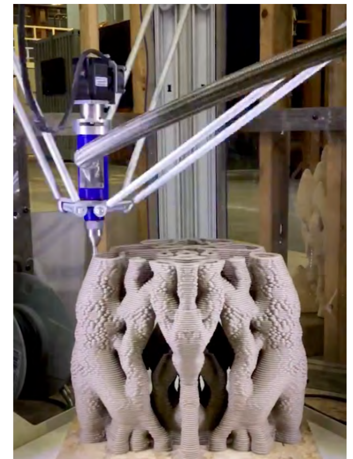
Figure 3. 3D Printing Process of Reef ( Urban Reef, 2023)
