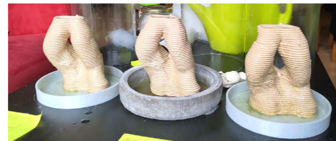
Figure 19. First Pilot test at home Reefs ( From left to right: Hydrogel, water, Agar)
