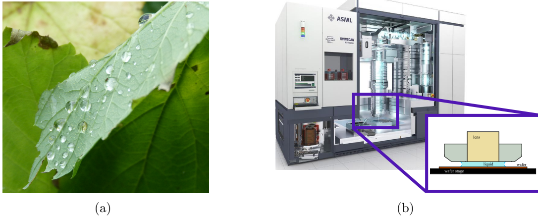
Figure 1.1: (a) Rain droplets on a leaf (photograph taken in Kiev, Ukraine), (b) state-of-the-art ASML immersion lithography equipment: TWINSCAN NXT:1950i ( www.asml.com ). The inset shows a schematic of the immersion lens of the lithography system.
