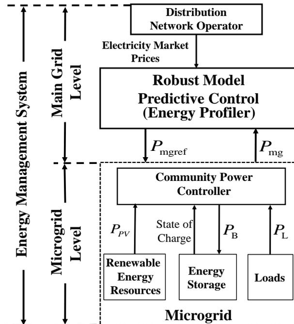
**Figure 1.** Hierarchical energy management system (EMS) Structure.
