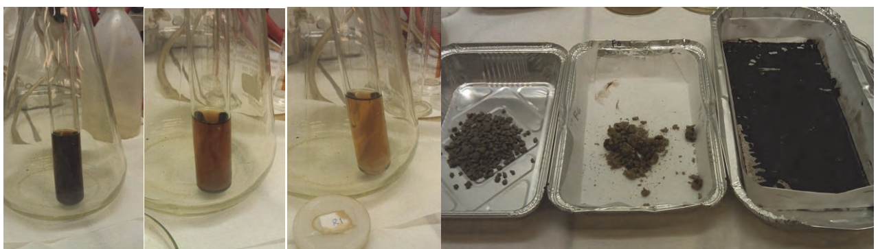
(a) (b) Figure 5.3. (a) From left to the right are the dichloromethane+dissolved bitumen after 1 st , 4 th and 7 th process (b) From left to the right are the granular Retona in original form, the extracted filler, and the extracted bitumen.
