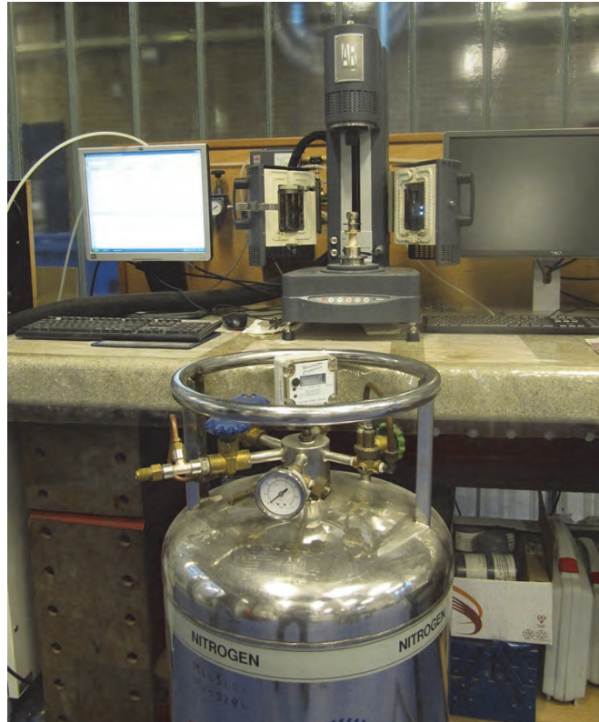
Figure 4.1. Dynamic shear rheometer machine and liquid nitrogen vessel
