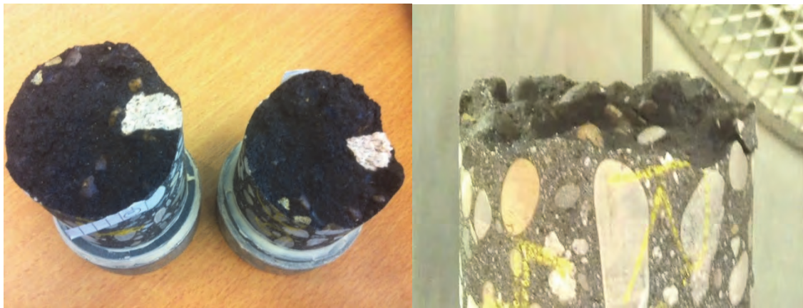
Figure 5.18. Typical failure at 5°C around the aggregate -adhesive- (right: test at 5°C and 1%/s) and at 20°C through an aggregate particle (left: test at 20°C and 0.01%/s);
