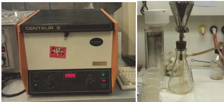
Figure 5.2. The Centaur 2 centrifuge (left) and the Erlenmeyer (right), connected to the vacuum pump, with the microfiber filter paper
