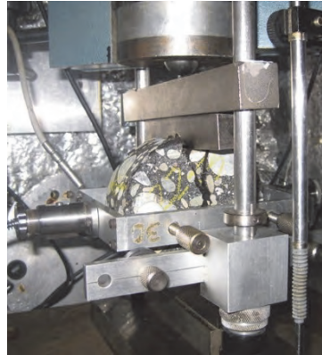
Figure 3.10. Indirect tension test set-up
