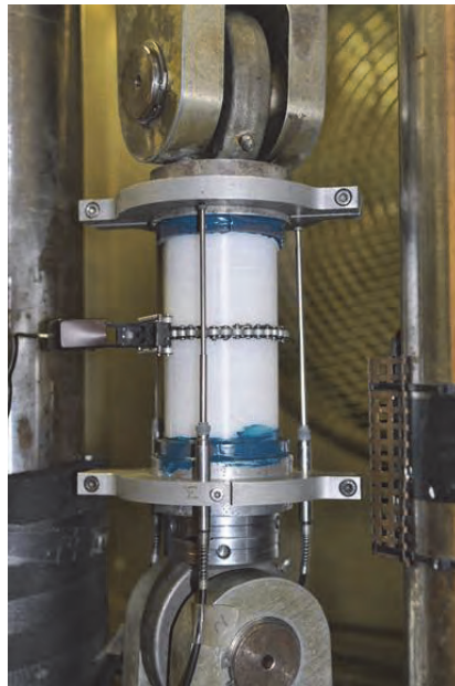
Figure 4.28. Delrin specimen in the set-up to validate the test method
