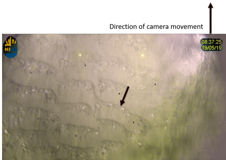
Figure 4.10: Still frame from video data. The black arrow in the frame indicates the direction of the sand ripples. The arrow above the frame indicates the direction of camera movement. Yellow lines were drawn in ImageJ to determine ripple orientation and length.
