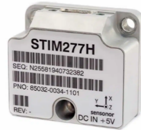
Figure 2.15: Safran STIM277H MEMS gyroscope [15]
