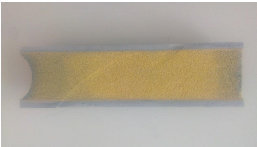
Figure 76: Carbonate (chalk) core after nanoparticle experiment
