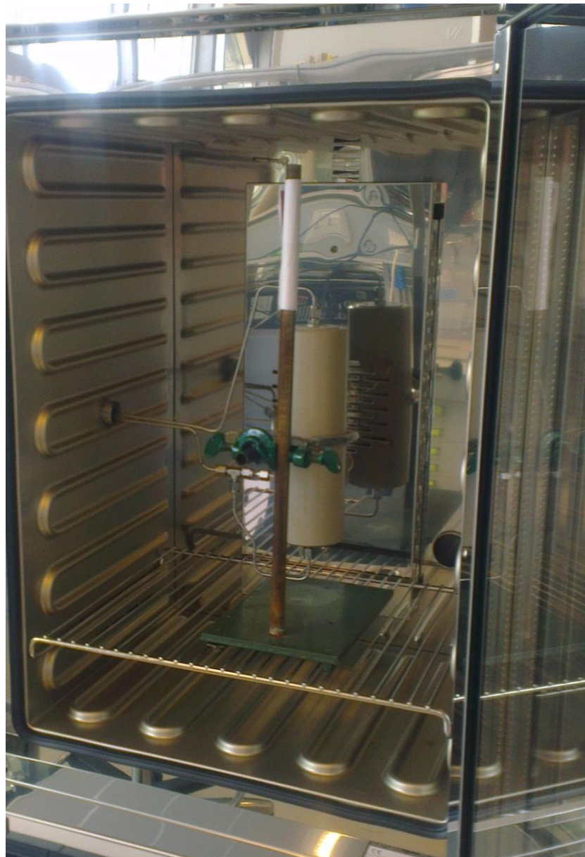
Figure 22: Picture of core holder inside oven
