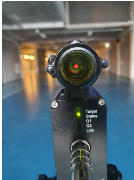
Figure 4.6: The laser used for measuring athlete velocity
