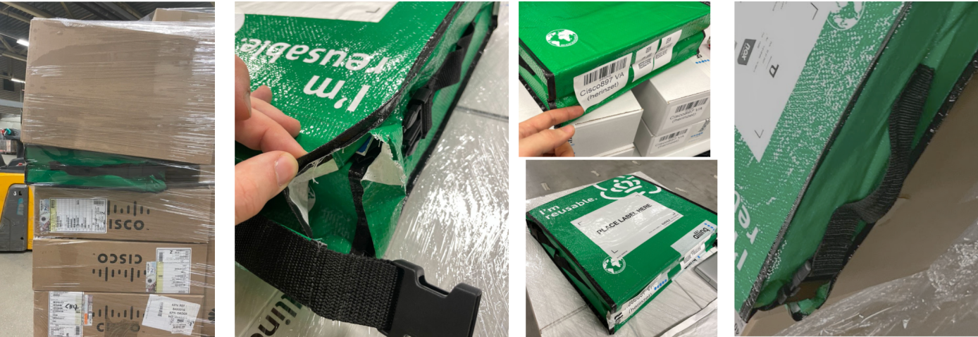
Figuur 52 F.I.t.r. the flaws with protection, stackability, stickers coming off and the risk of getting stuck behind something.
