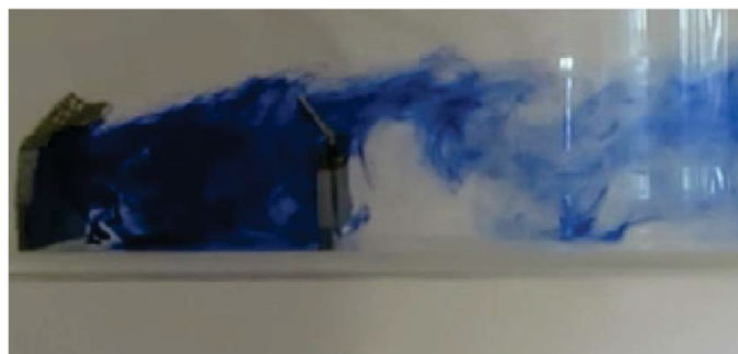
Figure 3.5: Flow visualization investigating the effect of overhanging ESPs installed on top of the sound barriers. Figure reproduced from Alfonsi et al. [11].
