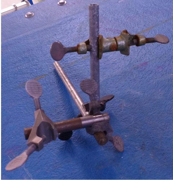
(a) The first pitot tube traverse structure composed of cylindrical rods and mechanical traverses.
