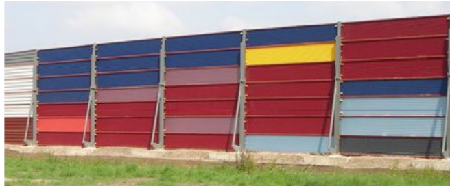
Figure 1.3: A 7 m tall sound barrier being tested at Strandnulle. Photo reproduced from Hooghwerff et al. [8].
