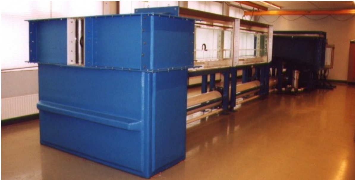
Figure 4.1: The water tunnel facility. Image reproduced from the website of Engineering Laboratory Design Inc [73].
