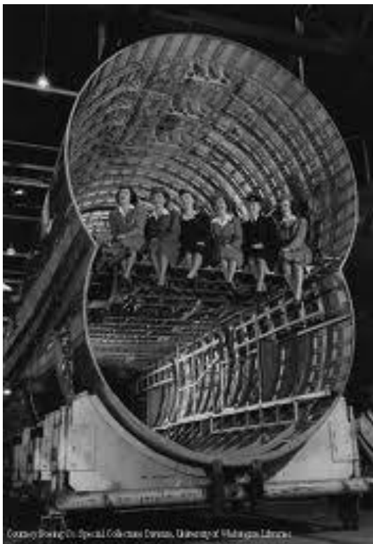
Fig. 1.3: Cross-section of the fuselage of the Boeing 377
