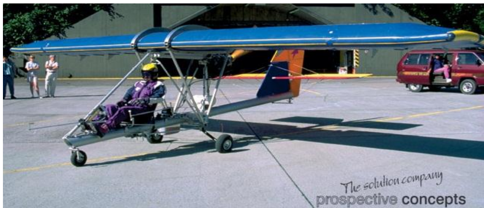
Fig. 1.2: The inflatable wing of the pumpolino, made by prospective concepts
