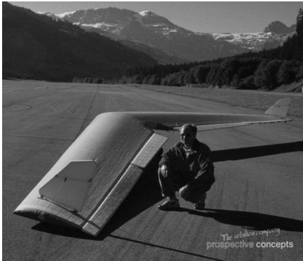
Fig. 6.5: Inflatable aircraft from [Prospective Concepts]
