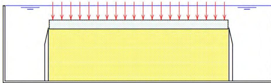
Figure 5.2: The one-dimensional case of flow and deformation in the vertical direction only. Reprinted from Verruijt (2010).
