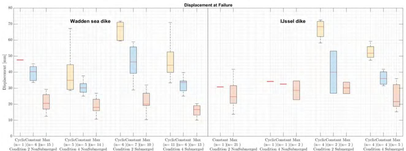
Figure 4.8: Comparison of the displacement at failure of the grass cover sample for the different test variables.
