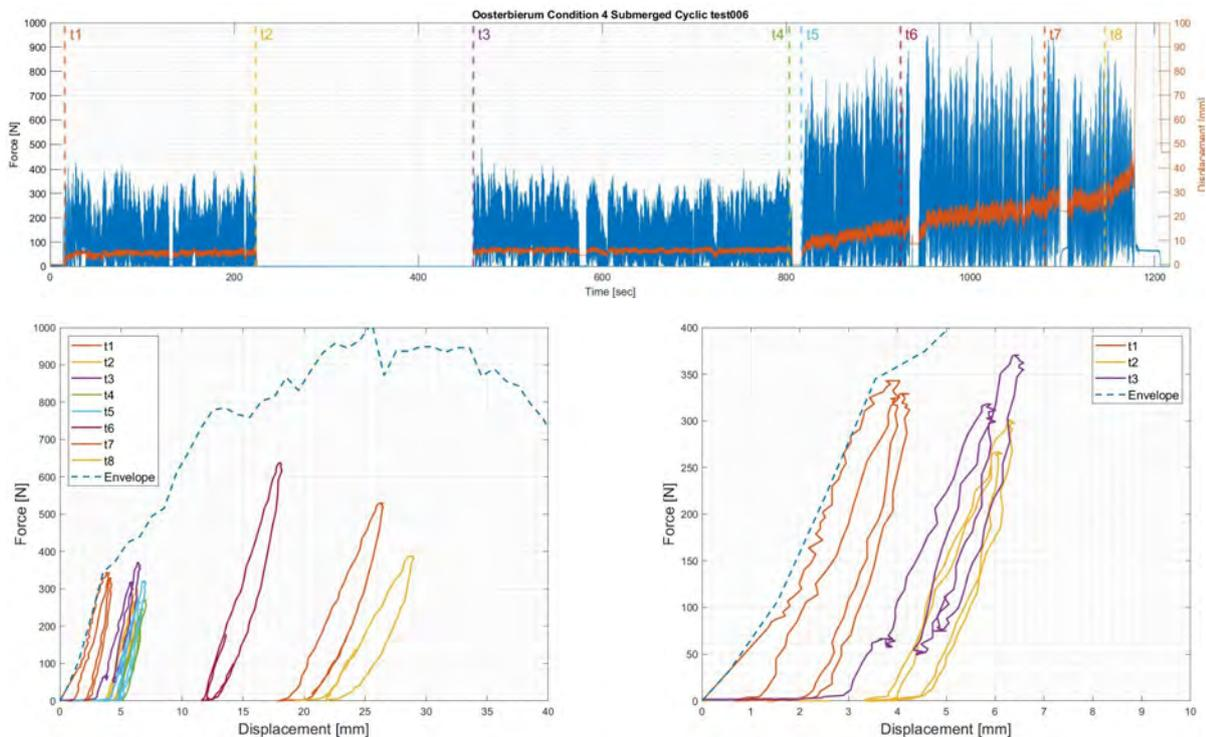
Figure 4.17: Development of Load - Displacement relation over successive loading cycles. The graphs in the lower panels show the Load - Displacement relation at points in time as indicated in the top panel. The envelope of the total the Load - Displacement relation is depicted as well. The lower right panel shows a close-up of the t1 until t3 and points out the effect of an increased time between successive loading cycles.
