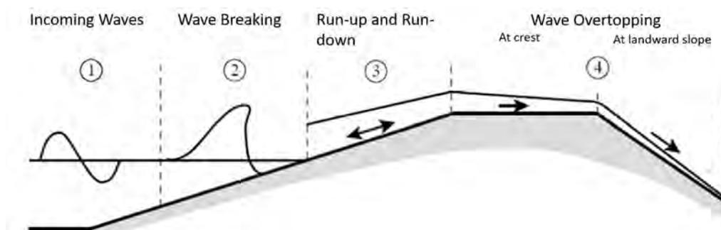
Figure 1.1: Hydraulic processes of breaking, run-up and run-down and overtopping of waves. Reprinted from Schüttrumpf and Oumeraci (2005).
