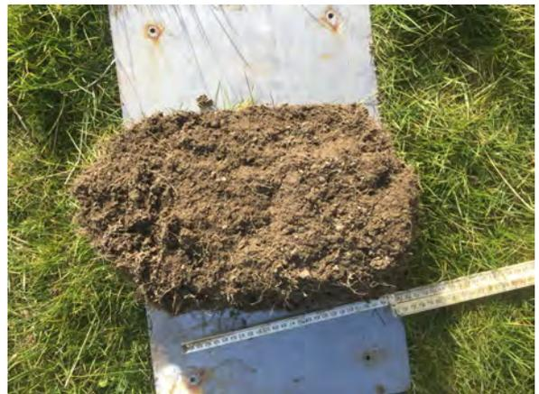
Figure 4.12: Picture of grass sod specimen after it was lifted out of the grass cover. The typical shape of the grass sod shows widths of circa 20 cm at the edges increasing towards the centre of the grass cover sample.
