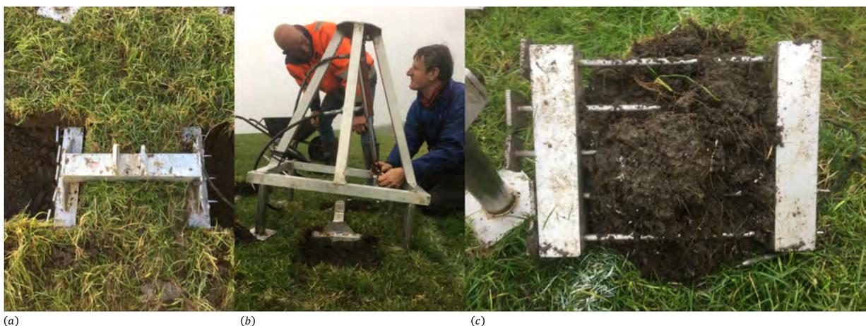
Figure B.1: The test set-up of the sod pulling test with pull frame and supporting frame Source :Own pictures November 2018.
