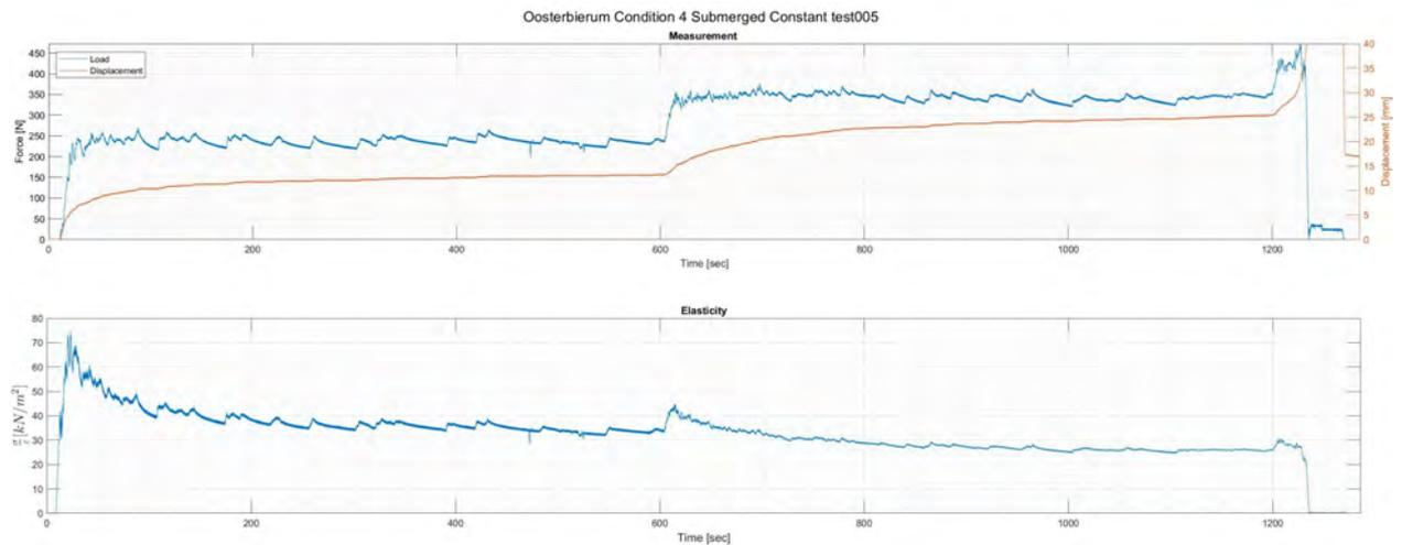
Figure 4.1: An example of typical development deformation and elasticity of the grass cover due to stepwise increased constant load. In the top panel the raw measurement of load and displacement is depicted. The lower panel depicted the resulting elasticity of the grass cover.
