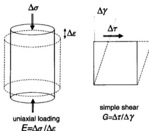
Figure 2.4: Elastic moduli. Reprinted from Winterwerp and Van Kesteren (2004).
