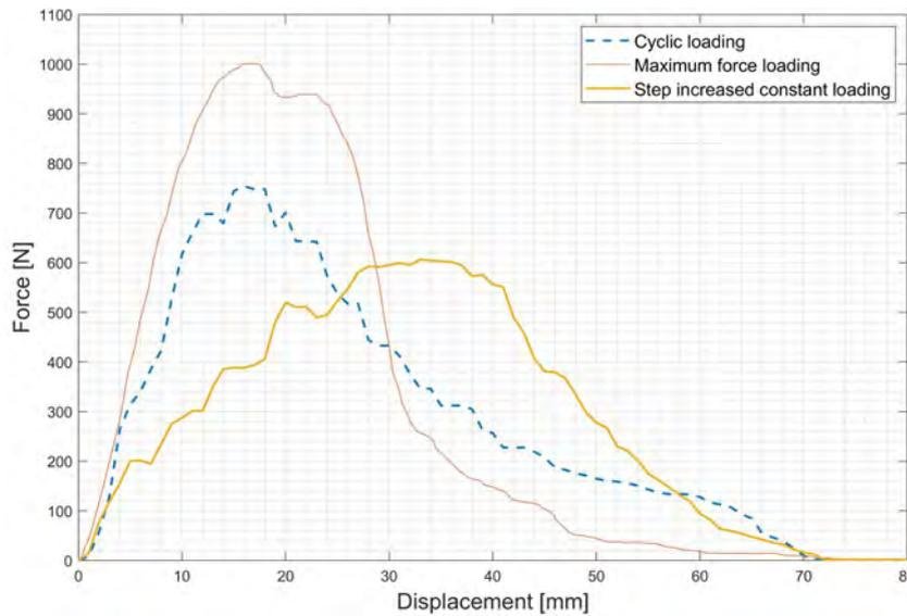
Figure 4.7: Typical Force - Displacement curve for the three different load regimes. The stepwise increased constant load and the cyclic load were force controlled and the maximum force load was displacement - controlled.
