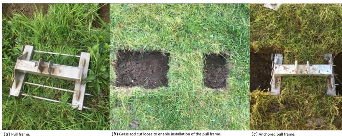
Figure 3.1: The test set-up of the sod pulling test, pull frame.
