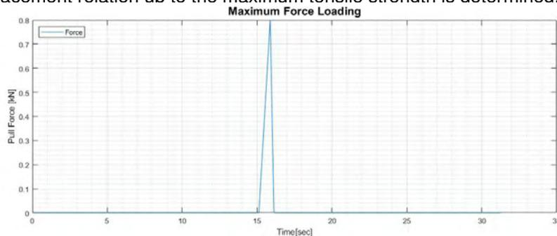
Figure 3.6: Variable: Load Regime. During maximum force loading, the grass sod is loaded with a constant pull rate until failure occurs.
