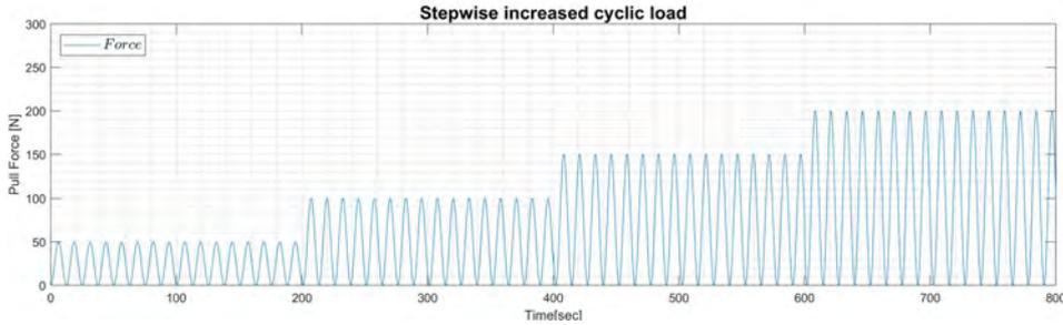
Figure 5.1: During cyclic loading, the grass sod is repetitively loaded with a constant period of  $0.5 \text{ Hz}$  and a stepwise increased amplitude. The amplitude of the load increases every 100 cycles with  $50 \text{ N}$ , starting with a load of  $50 \text{ N}$ . This process proceeds until failure occurs.
