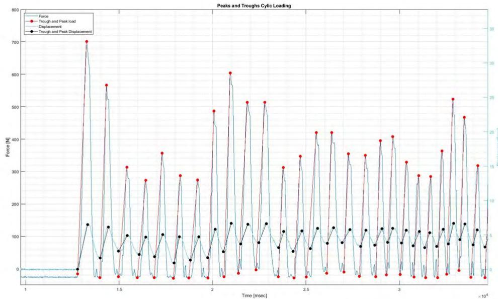
Figure 3.12: The local minima and maxima are determined with standard functions based on spline interpolation available in MATLAB R2019a.
