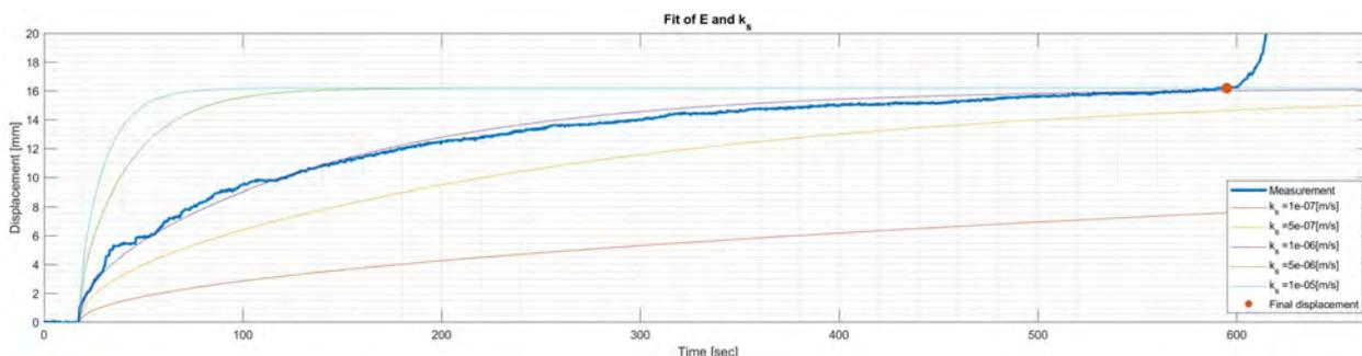
Figure 5.3: Example of method to determine  $E$  and  $k_s$ , applying the expression for degree of consolidation as described by Verruijt (2010). For this example the results of the submerged stepwise increased load regime, as described in Section 3.2, were used as input. Please note that the induced load is not in agreement with the load as proposed.
