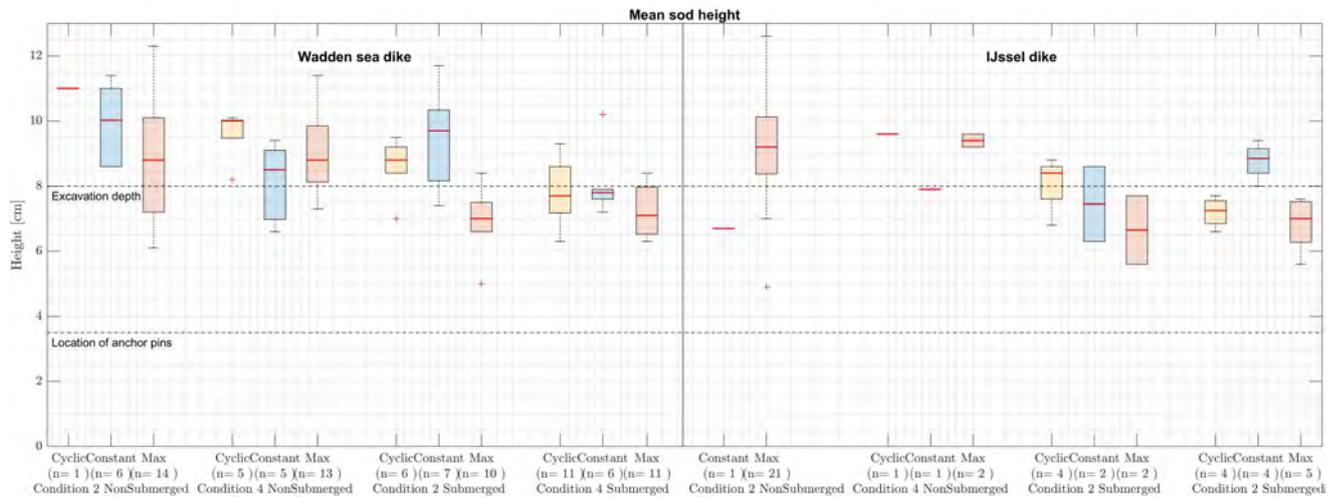
Figure 4.4: Comparison of the height of the grass sod after the sod was lifted out the grass cover.
