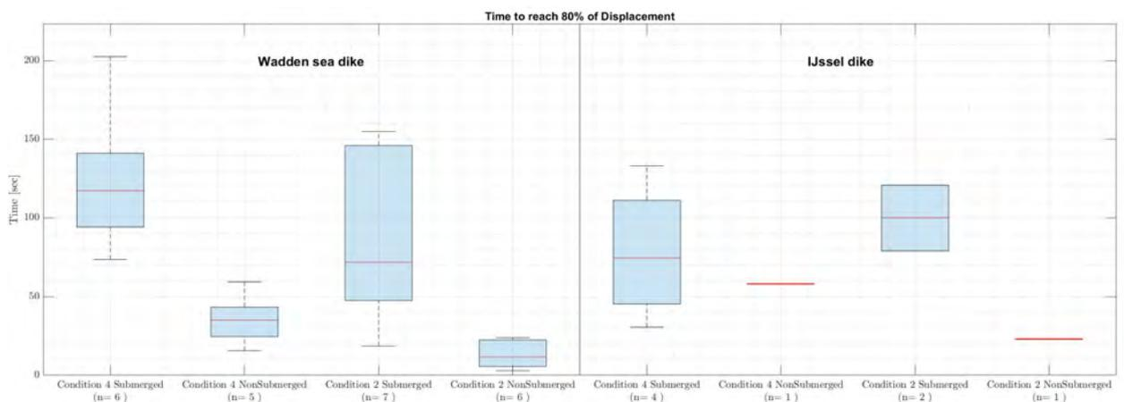
Figure 4.2: Comparison of time to reach 80% of final displacement between submerged and non submerged conditions under constant loading.
