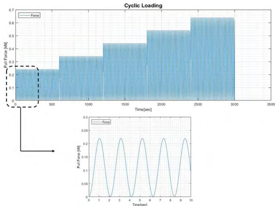
Figure 3.5: Variable: Load Regime. During a stepwise increased cyclic load, the grass sod is repetitively loaded with a relative constant amplitude, mean load and period. The amplitude of the load increases every 10 minutes with circa  $0.2\text{ kN}$ , starting with a load of circa  $0.2\text{ kN}$ . This process proceeds until failure occurs.
