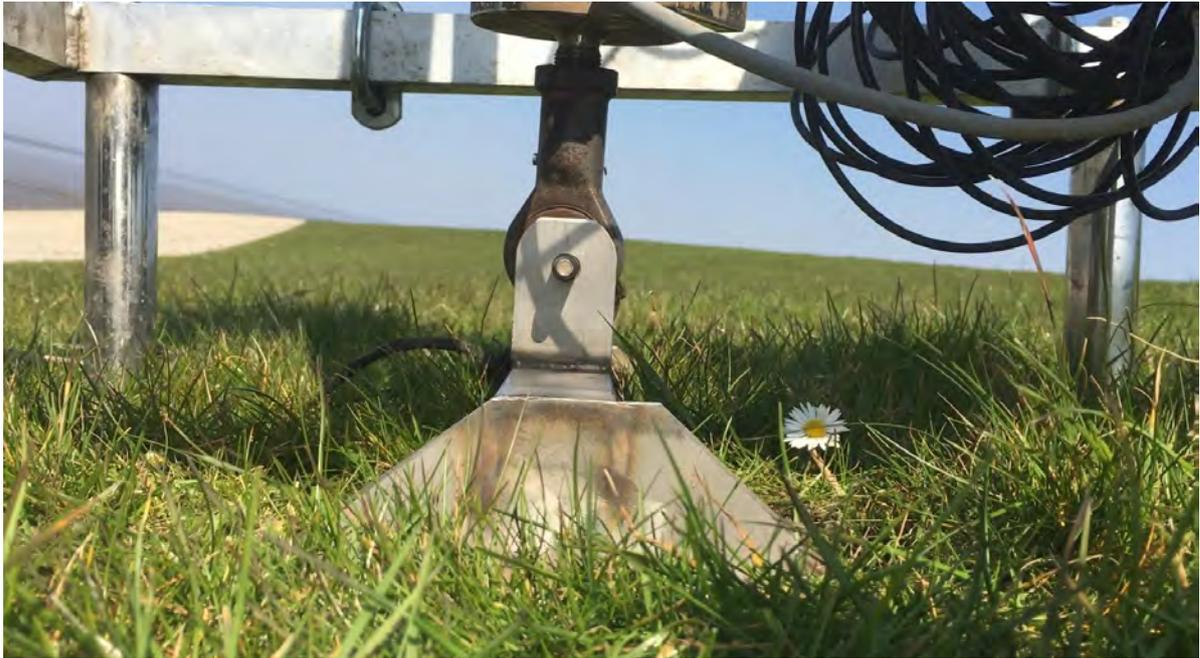
Execution of a cyclic load test under non submerged conditions. The video shows the last part of the test up to failure of the grass cover. Scan QR code to start video.
