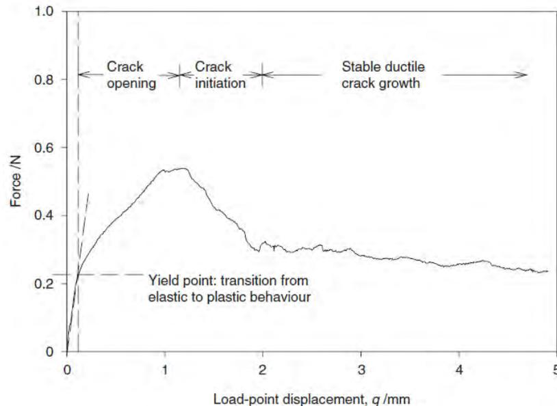
Figure 2.5: Force - Displacement diagram with the stages of crack growth in wet soil. Reprinted from Hallett and Newson (2005).
