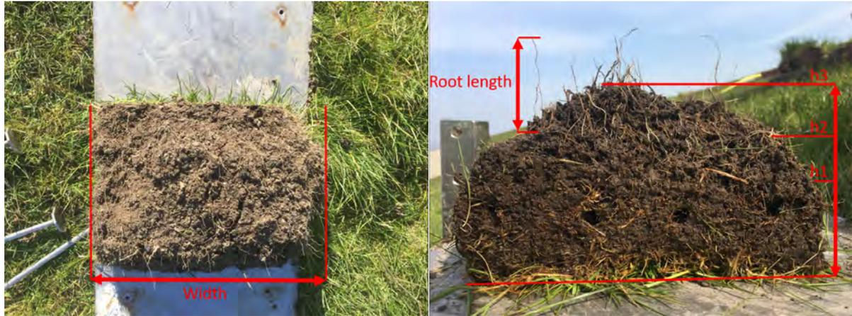
Figure 3.11: The measured dimensions are indicated by the red arrows.
