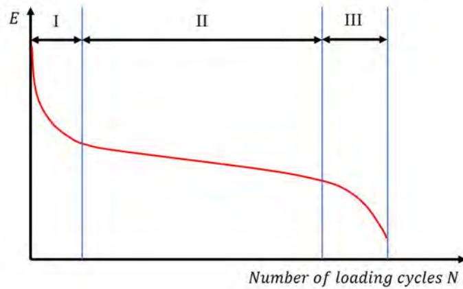
Figure 2.8: The successive phases of stiffness decrease due to fatigue. Reprinted from Li (2013).
