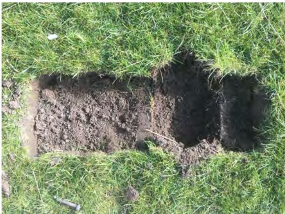
Figure 4.11: Picture of grass cover after the specimen was lifted out of the grass cover. The print of the grass sod in the subsoil shows that the failure plane attaches to the adjacent grass cover at the location of the edge of the grass cover sample.
