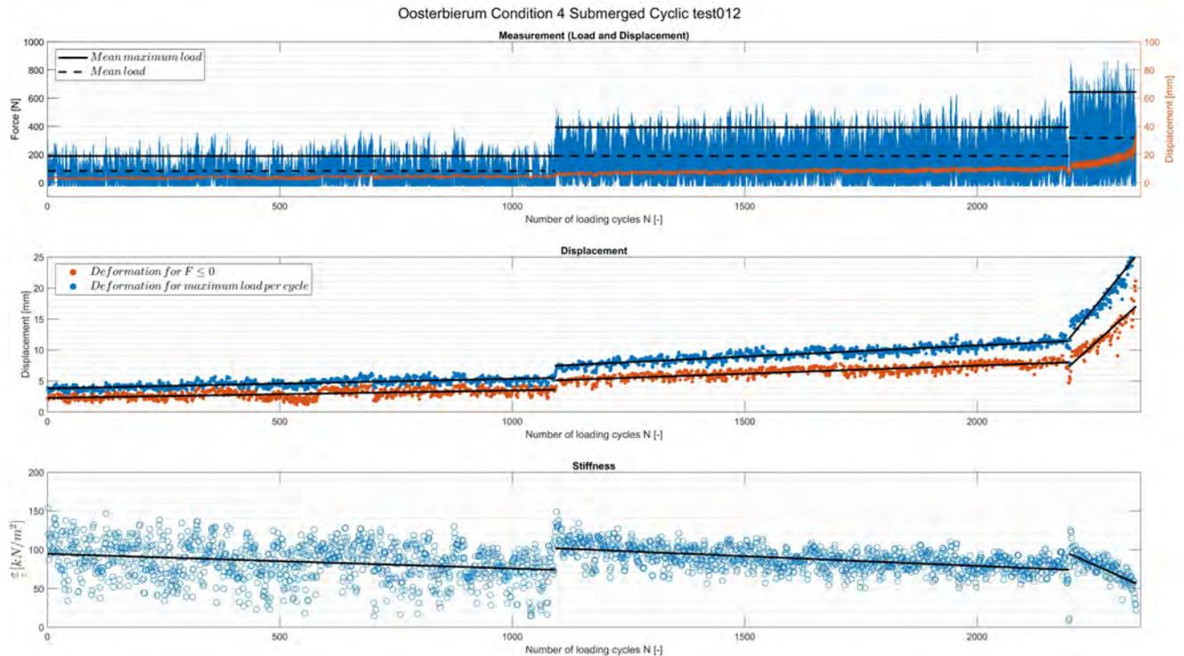
Figure 4.15: Example of typical behaviour under repetitive tension loading. The figure shows a change in inclination of the trend line in displacement and stiffness due to increase of the load. Linear line was fit to the data with standard linear regression functions available in *MATLAB R2019a*.
