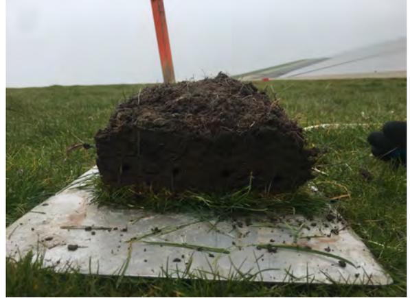
Figure 4.10: Picture of grass sod specimen after it was lifted out of the grass cover. The typical shape of the grass sod shows small heights at the edges increasing towards the middle of the grass sod.
