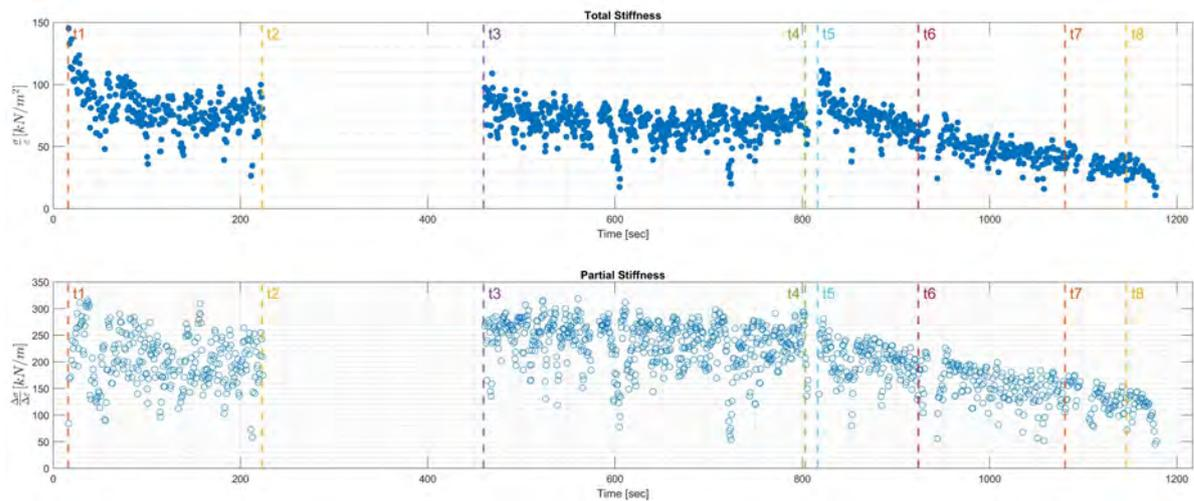
Figure 4.18: Development of total and partial stiffness as defined in section 3.3.
