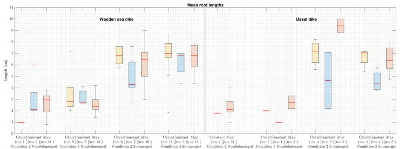
Figure 4.5: Comparison of the mean root length of the grass sod after the sod was lifted out the grass cover.
