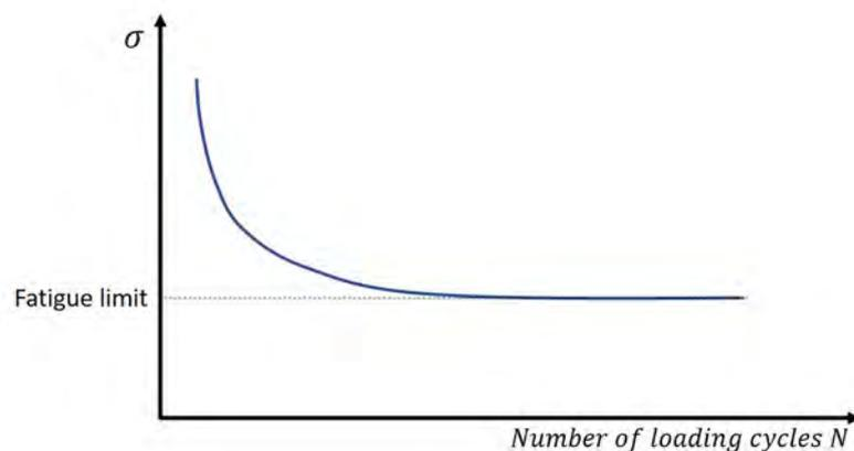
Figure 2.9: S-N curve depict the number of loading cycles until a specimen fails for different stress amplitudes. Adapted from Yang and Den Uijl (2019).
