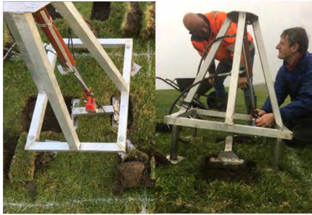
Figure 3.2: The test set-up of the sod pulling test, pulling mechanism.
