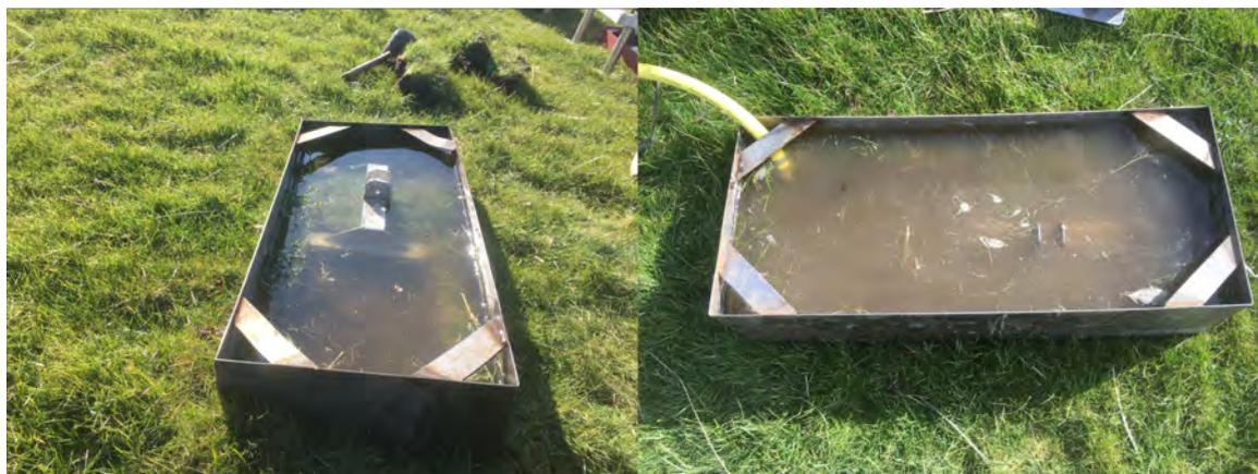
Figure 3.7: Variable: Degree of saturation. Box used to perform grass pulling test in submerged conditions.
