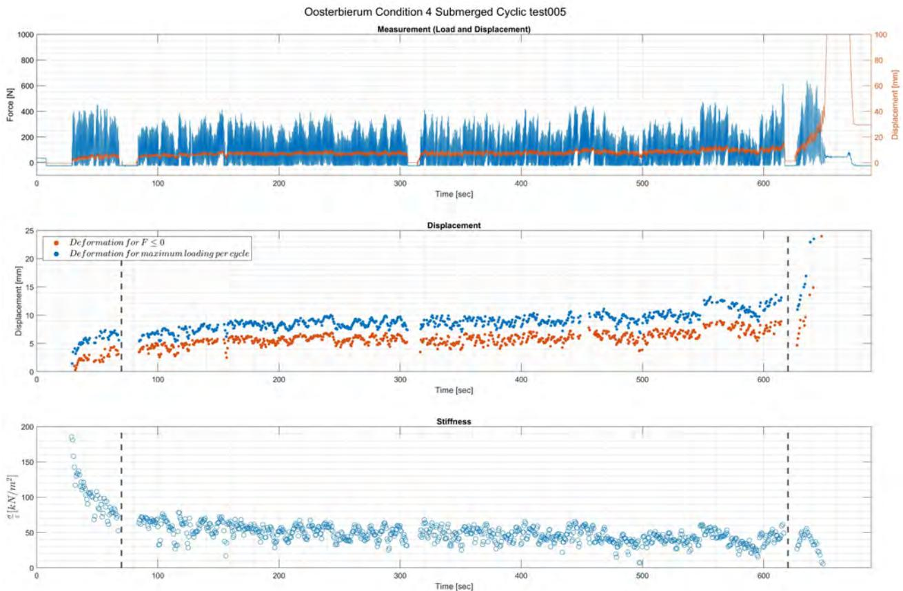
Figure 4.14: Example of typical behaviour under repetitive tension loading. The figure shows the results of cyclic loading during submerged conditions and with four sides cut loose. The top panel shows the raw measurement of force and displacement. The center panel shows the maxima and minima of the measured displacement per cycle. The lower panel depicts the elasticity for each load cycle. The variables are shown as a function of time.
