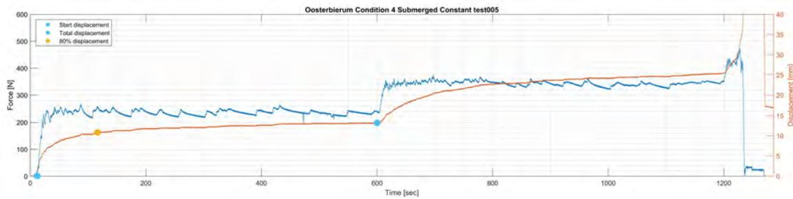
Figure 3.10: Displacement rate induced by a stepwise increased constant load. The blue dots indicate the total or final displacement as result of the induced load during the first 600 seconds of loading. The yellow dot indicates 80% of the final displacement.
