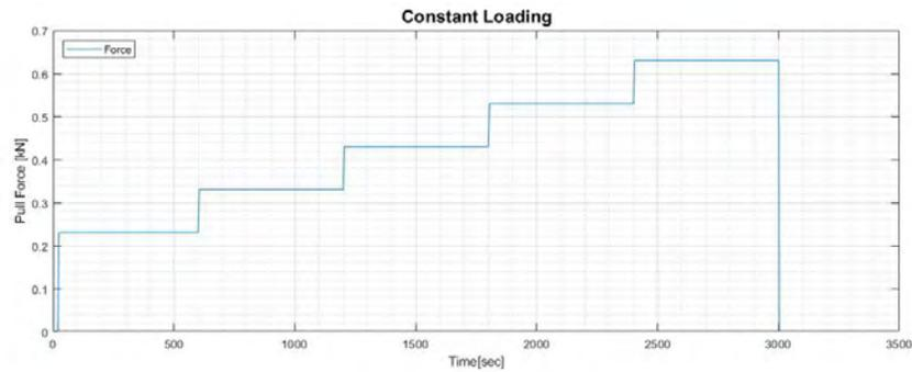
Figure 3.4: Variable: Load Regime. During constant loading, the grass sod is loaded with a constant load. The load increases every 10 minutes with circa  $0.1\text{ kN}$ , starting with a load of circa  $0.2\text{ kN}$ . This process proceeds until failure occurs.
