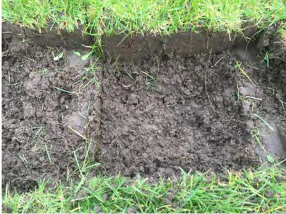
Figure 4.9: Picture of grass cover after the specimen was lifted out of the grass cover. The print of the grass sod in the subsoil show that the failure plane attaches to the maximum excavation depth necessary to anchor the pull frame.
