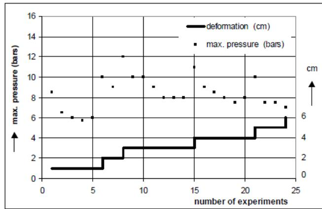
Figure 2.6: Fatigue of the grass cover. The effect of fatigue is shown by imposing a constantly increasing displacement. Every imposed displacement is repeated several times, after which the displacement is increased. A clear reduction of the required pull force can be seen. Source: Pijpers(2013).
