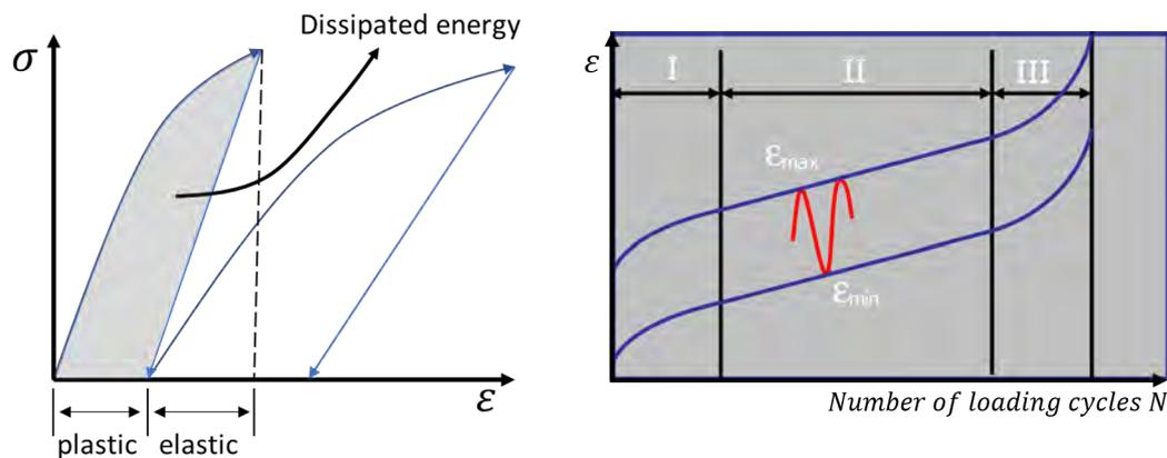
Figure 2.7: Plastic deformation is irrecoverable and is accumulated during successive loading cycles. The left panel shows typical plastic and elastic behaviour as found for concrete under cyclic loading. The right panel show the strain ( $\varepsilon$ ) development during cyclic loading of a specimen. Adapted from Yang and Den Uijl (2019).
