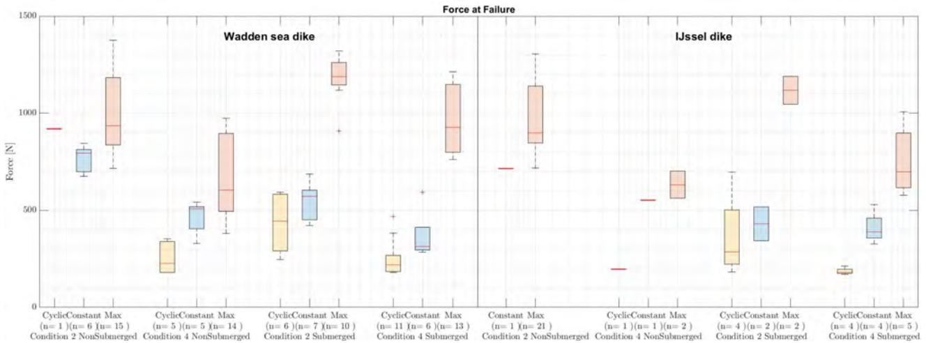
Figure 4.13: Comparison of the load that causes failure of the grass cover between Cyclic loading, Constant loading and Maximum force loading.
