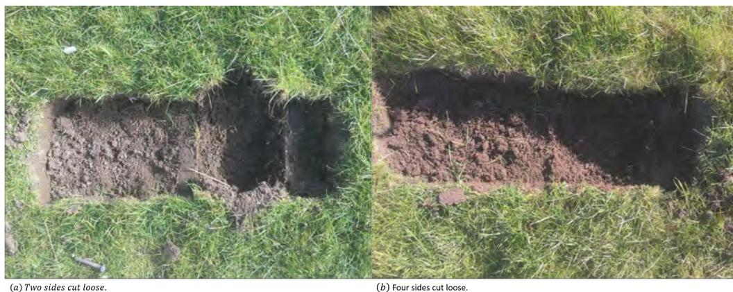
Figure 3.9: Variable: Number of cuts. Difference of failure plane between two and four cuts.
