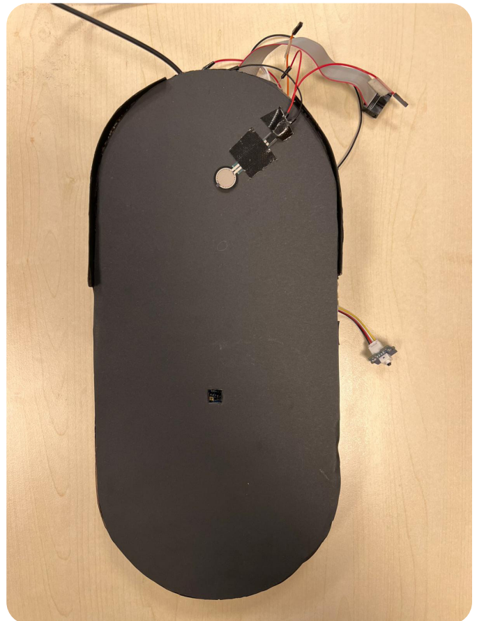
Figure 60. New locations pressure and light sensors
