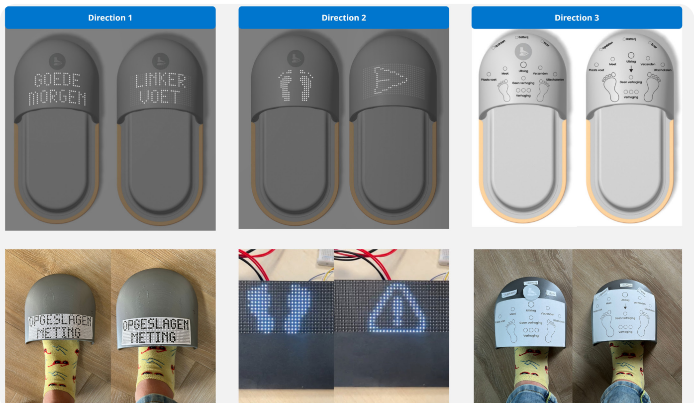
Figure 48. Low-fi prototyping of the three directions
