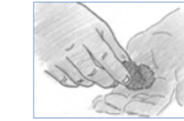
Fig. 2.7. Ribbon Test: Forming a ribbon by pressing wet soil between the thumb and forefinger helps assess clay content. Longer ribbons indicate higher clay percentages, which enhance block strength. Source: NSW Department of Primary Industries (2014).
