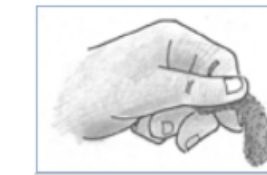
Fig. 2.7. Ribbon Test: Forming a ribbon by pressing wet soil between the thumb and forefinger helps assess clay content. Longer ribbons indicate higher clay percentages, which enhance block strength. Source: NSW Department of Primary Industries (2014).
