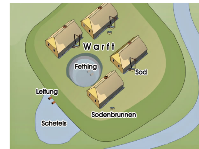
Figure 2.9. Freshwater supply system on a Warft (artificial dwelling mound) in the Hallig region of northern Germany. The diagram shows a tiered water management strategy: Fething is a central livestock watering pit; Schetels are shallow peripheral basins for additional storage; and Sod is narrow, sealed cisterns collecting rainwater from rooftops for human consumption. This layered approach illustrates how freshwater was secured in salt-marsh environments, comparable to practices in terp settlements in the northern Netherlands. Source: Waddenacademie (2017), adapted from the Pitt Rivers Museum, University of Oxford.
