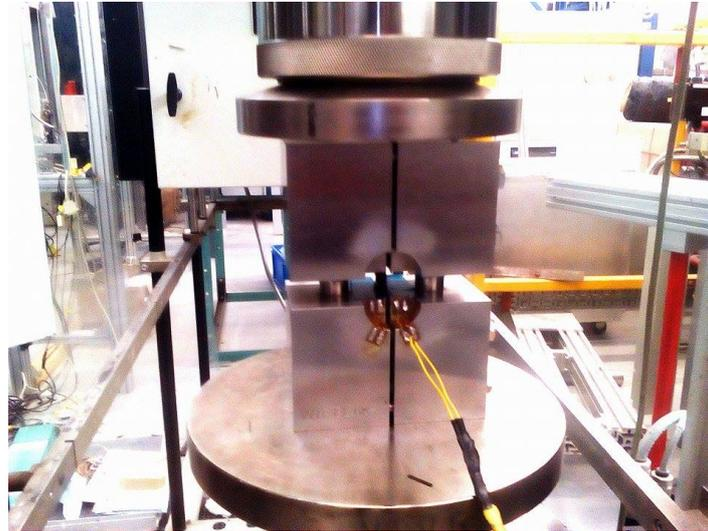
**Figure G.6:** CLC fixture for the compression test
