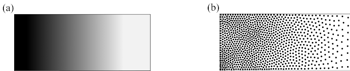
Figure 5.2: Feature of the sampling density transformation: (a) a horizontal gradient map is transformed to, (b) a set of sampling points whose spatial density distribution is proportional to the input gradient map.
