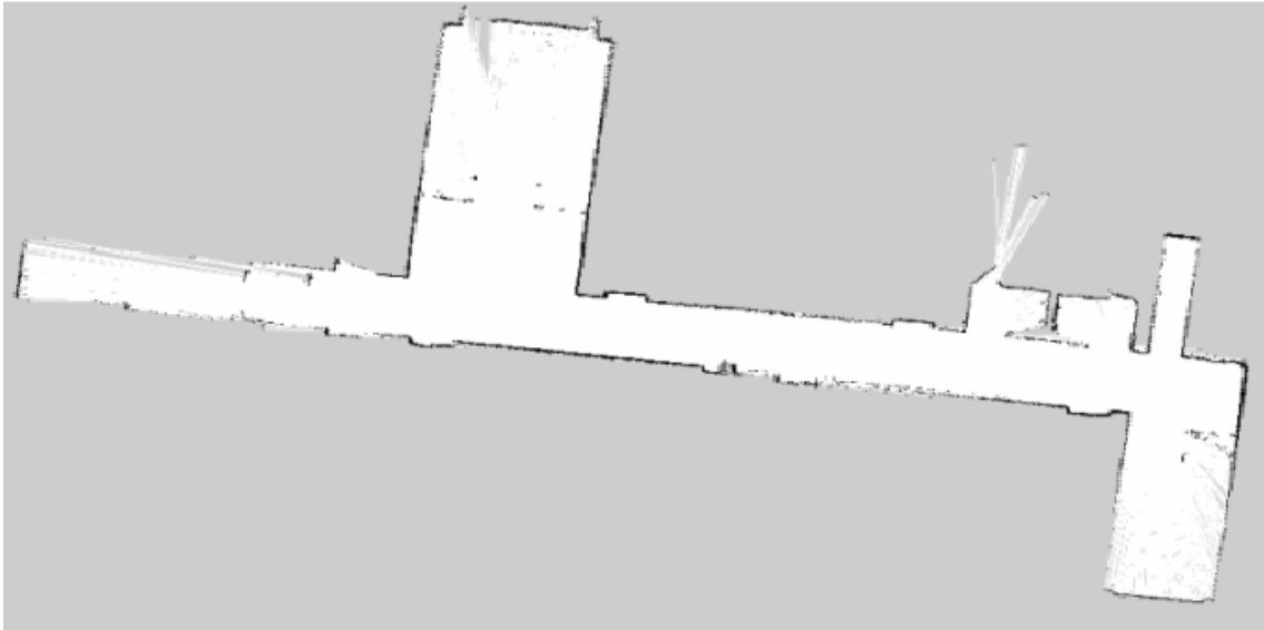
Figure 1.1: An example of an occupancy grid-map, the black cells indicate occupied cells such as walls. Grey denotes unknown space and white denotes the free spaces with no obstacles. Such maps are commonly used for navigation or localization tasks. Image adopted from [7].
