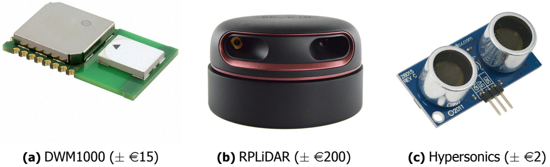
Figure 2.8: Three different range sensors, from left to right based on: radio ( UWB ), optics (laser) and acoustic (hypersonic).
