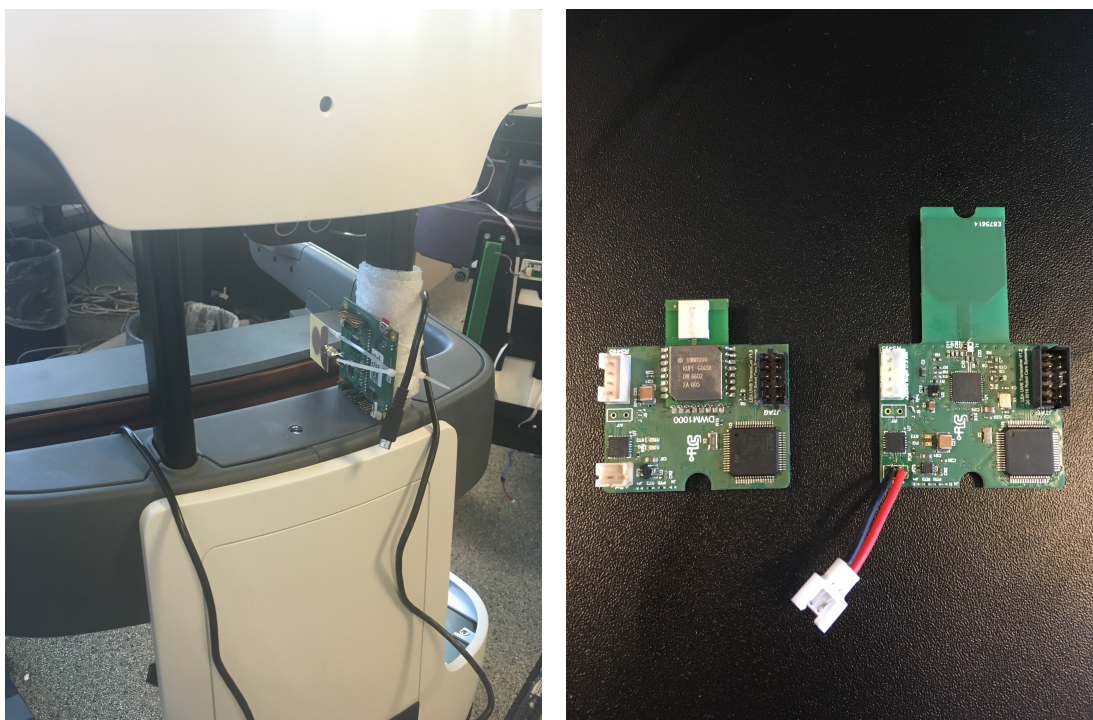
Figure C.2: On the left: Decawave demo-module attached to LEA in a rather primitive matter. On the right: two versions of the ultra-wideband module designed at Robot Care Systems. The left one uses the DWM1000-module with an active antenna, the module on the right is the DW1000 with a passive antenna.
