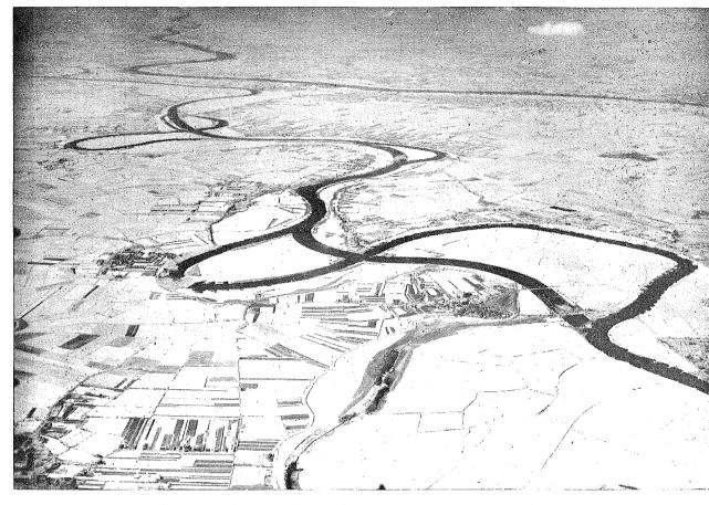
THE MEANDERING MAAS, which so often inundated large areas, has now been shortened and harnassed. The old loops are still there. The second river in the background is the Waal, the main branch of the Rhine. At one point they come close together. The Maas is now navigable for 2000-ton ships, the Waal for ships of more than 4000 tons. (Photo K.L.M.)
