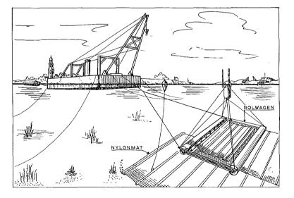
Complete new way of covering a shifty sand bottom with nylon sheets.
