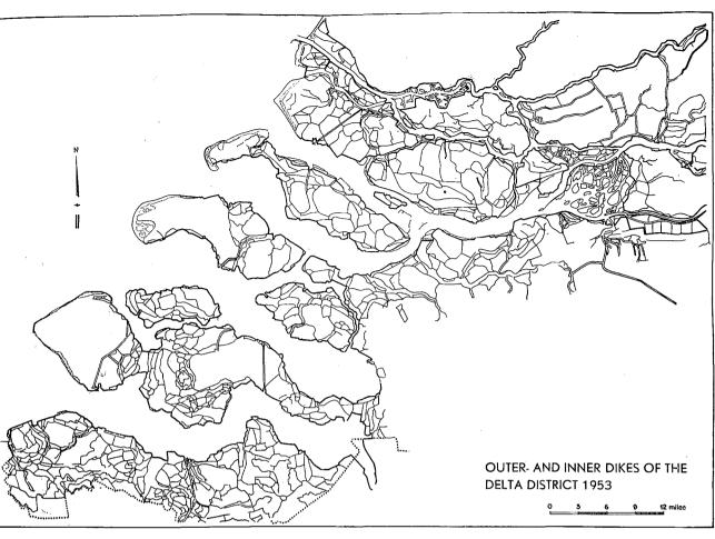
Zeeland's struggle to rise above the water has been hard indeed. Its ancient device 'Luctor et Emergo' and its enormous amount of inner dikes prove it. Each dike, still existent, was made to extend the islands bit by bit. Outer as well as inner dikes were broken by the 1953 flood.
