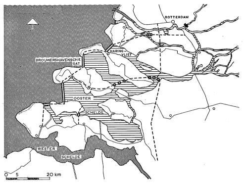
The Delta scheme for closing four southwestern estuaries. A fresh-water lake will be created here. The work will take about 25 years. Total length of dams 25 miles, maximum depth about 100 ft, bottoms consist of loose sand.
