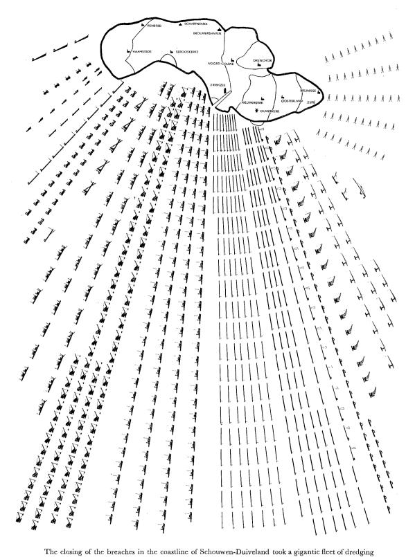
The closing of the breaches in the coastline of Schouwen-Duiveland took a gigantic fleet of dredging and construction material; 126 tugboats, 283 barges of 300 to 700 tons, 38 dredges, 49 cranes, 105 draglines, 43 launches, 53 locomotives, dukw's, bulldozers, and so on. About 5000 workers have been employed here during several months.
