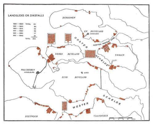
The above map shows the constant threat of landslides. Zeeland's tidal waters scour its shores in such a way that landslides occur, even though these shores are defended against scour. Viewed over centuries large areas have been lost in Zeeland by landslides, and still new ones are to be feared.
