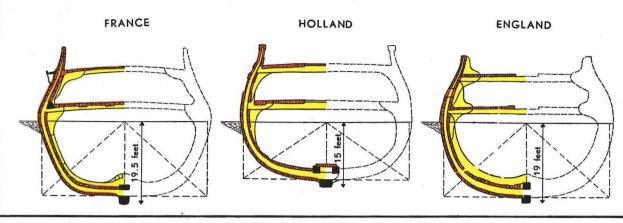
Main frames of ships in 1750, showing how the Dutch ships could not compete any longer because of lack of draught, owing to lack of depth in their harbours and inlets (after E. van Konijnenburg). (Depths in Amsterdam feet.)
