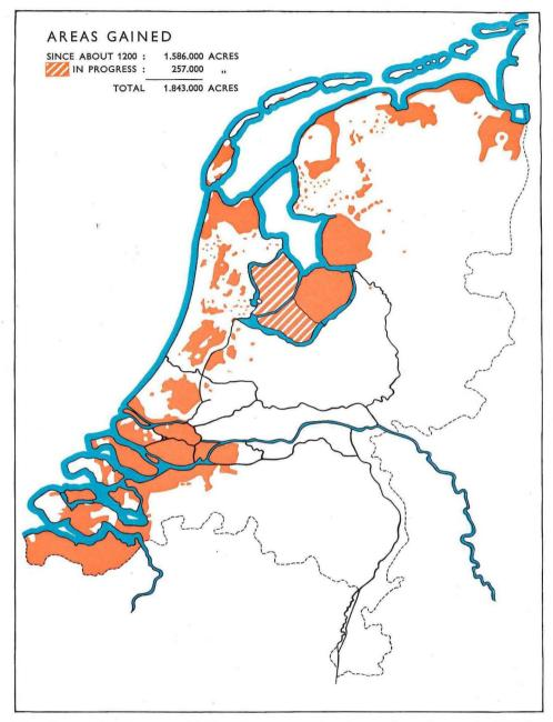
The red spots indicate the areas which have been obtained either by accretion, or by pumping lakes dry.
