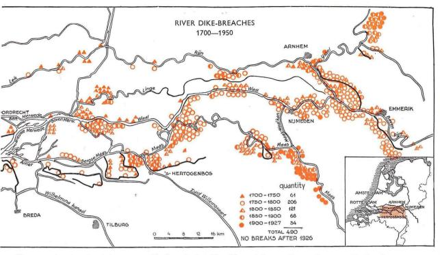
Since 1700 almost 500 breaks have occurred in the main river dikes. The period 1750–1800 was the worst with 4 breaks a year. In February 1953 the breaks in the dikes of the down stream polders were not due to the overflowing rivers, but to the water being driven in from the seaside through the simultaneous action of spring tide and a heavy northwestern storm.
