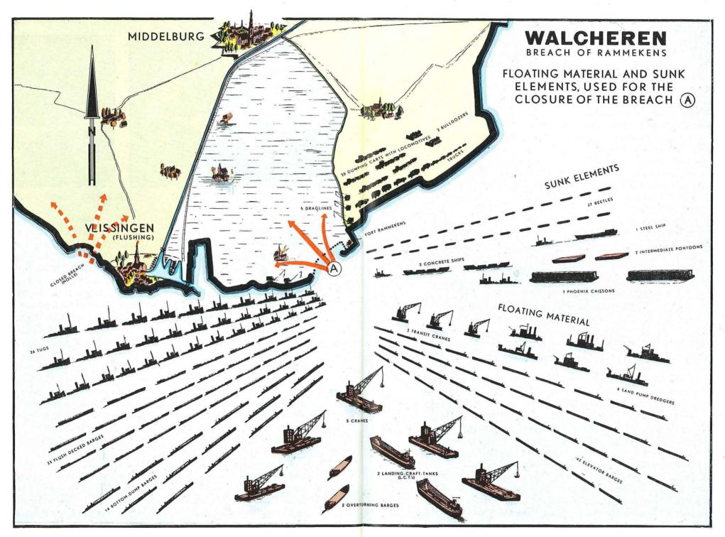
The breach of Rammekens, one of the four gaps the Allies had to make in order to drive the Germans out of the isle of Walcheren, was closed with great difficulty by using a large fleet of
