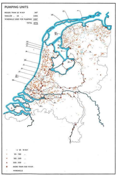
Holland is kept dry by continuous pumping with more than 4500 units.
