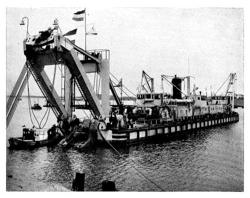
Modern cutter and suction dredger of high capacity.
