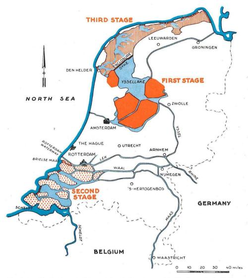
The closing of the Dutch coast will be carried out in three stages mainly. The first work, the Zuiderzee reclamation (1925–1980), the second work or Delta scheme (1954–1978), the third work or Wadden reclamation (not yet dated). The mouths of the Rotterdam and Antwerp Waterways remain open, according to the latest plans.
