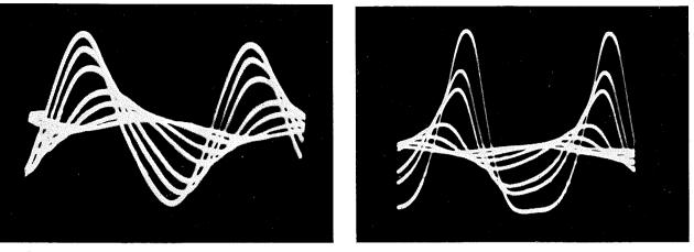
ELECTRICAL IMITATION OF TIDES The first tidal calculation (of the Zuiderzee enclosure) took 8 years. New schemes led Waterstaat to the use of the analogy between tides and alternating currents. The tidal rise and fall (left) is analogous to voltage, the tidal currents (right) to amperage.
