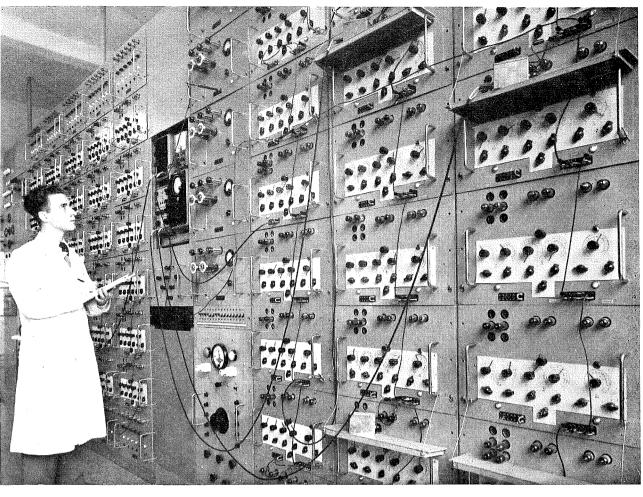
Electronic computer based on the analogy of tides and alternating currents. Every 'tide' takes one thousandth of a second.
