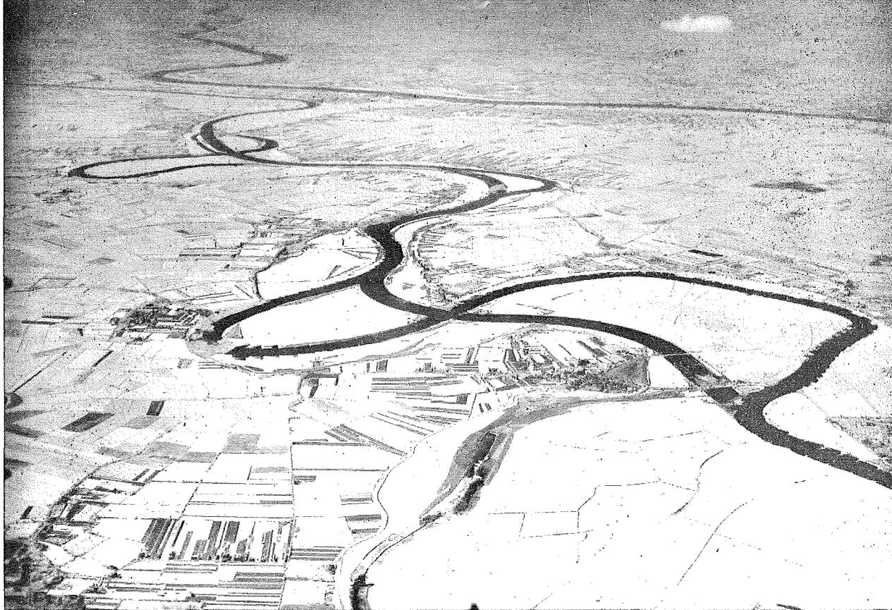
THE MEANDERING MAAS, which so often inundated large areas, has now been shortened and harnessed. The old loops are still there. The second river in the background is the Waal, the main branch of the Rhine. At one point they come close together. The Maas is now navigable for 2000-ton ships, the Waal for ships of more than 4000 tons. *(Photo K.L.M.)*
