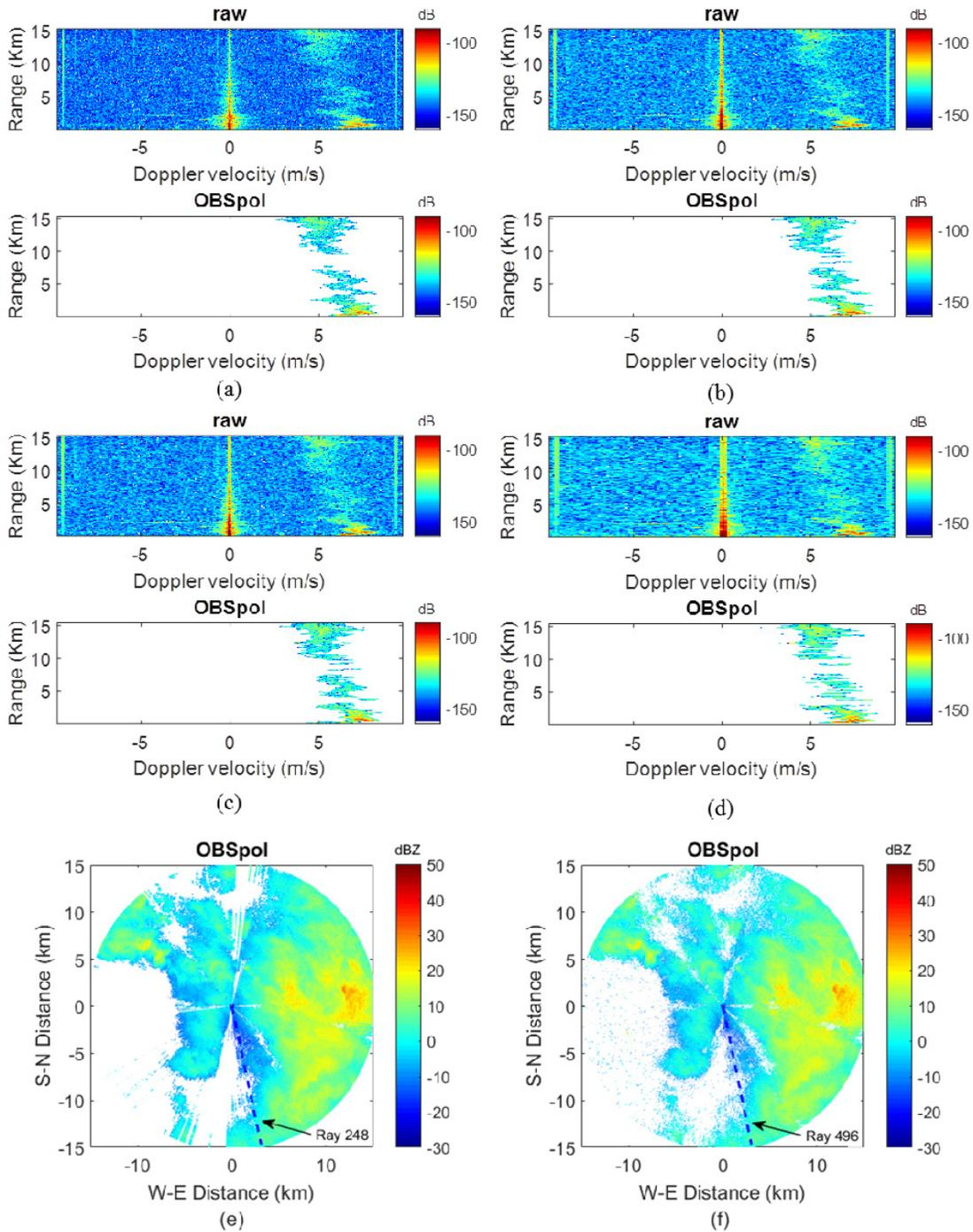
Fig. 13. OBSpol filter applied to radar data with different Doppler velocity resolutions. Data measured at 13:00 UTC on August 22, 2016. (a)  $sP_{hh}$  spectrogram with sweep number 512. (b)  $sP_{hh}$  spectrogram with sweep number 256. (c)  $sP_{hh}$  spectrogram with sweep number 128. (d)  $sP_{hh}$  spectrogram with sweep number 64. (e) PPI with sweep number 128. (f) PPI with sweep number 64.
