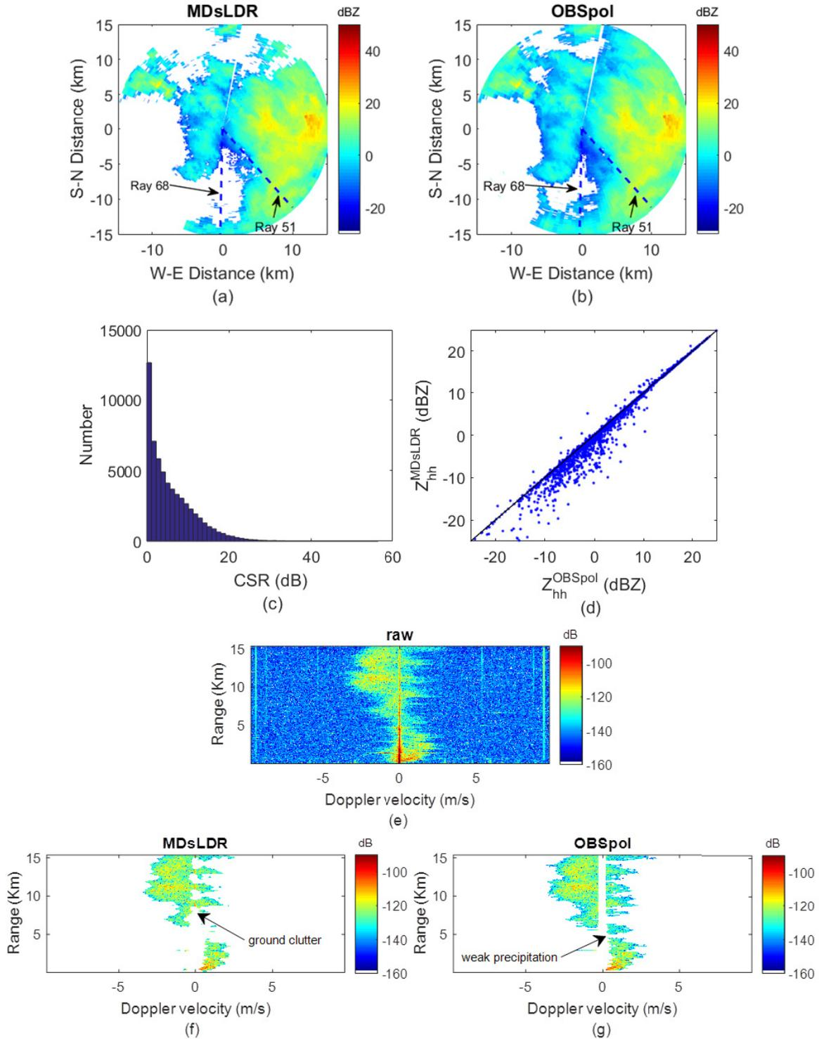
Fig. 11. Performance comparison between MDsLDR and OBSpol filters. Data measured at 13:00 UTC on August 22, 2014. (a)  $Z_{hh}$  after the MDsLDR filter. (b)  $Z_{hh}$  after the OBSpol filter. (c) CSR distribution of the OBSpol filter. (d) Scatter plot of the MDsLDR-filtered  $Z_{hh}$  and the OBSpol-filtered  $Z_{hh}$ . (e) Raw  $sP_{hh}$  spectrogram of Ray 51. (f) MDsLDR-filtered  $sP_{hh}$  spectrogram. (g) OBSpol-filtered  $sP_{hh}$  spectrogram.
