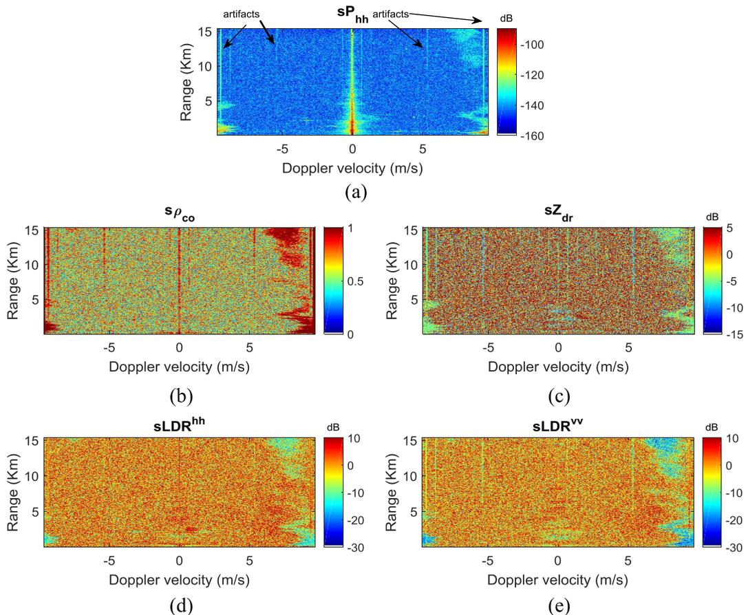
Fig. 3. Spectral polarimetric observables of IDRA. Data are related to Ray 68 of the measurements at 13:00 UTC on August 22, 2014. (a) Spectral power  $sP_{hh}$ . (b) Spectral copolar correlation coefficient  $s\rho_{co}$ . (c) Spectral differential reflectivity  $sZ_{dr}$ . (d)  $sLDR^{hh}$ . (e)  $sLDR^{vv}$ .
