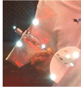
(b) Retro-reflective markers placed on the robot, with wings closed.
