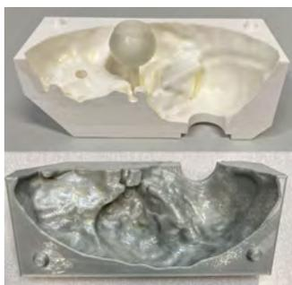
**Figure 3.8:** The two top parts of the brain mould with the tumor insert
