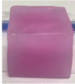
**Figure 3.2:** A PVA sample with the dimensions  $3,3 \times 3,3 \times 3,3$  cm
