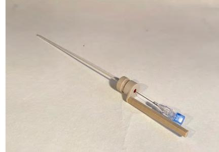
**Figure 4.7:** Cannula needle with pre-bend stylet
