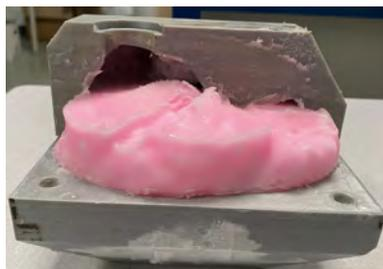
**Figure 3.17:** Brain phantom in the mould
