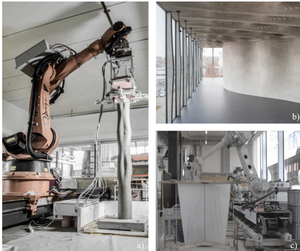
Fig. 21. a) Smart Dynamic Casting: Robotic Slipforming with flexible formwork [78], b) DFAB House, image Gramazio Kohler Research [80], c) ACDC Supported Thin Formwork [69].
