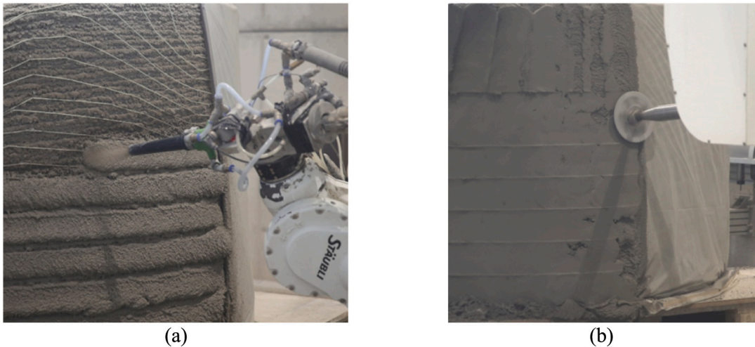
Fig. 24. Printing vertically onto a horizontally printed core: a) embedding the robotically fabricated fibre reinforcement; b) robotically trowelling the fresh concrete in a subsequent formative process, [101].
