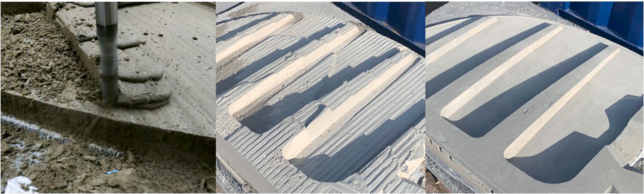
Fig. 25. Milling a 3DCP panel to create accurate and precise feature details while the printed material is in its green state (left); and the resulting impact on the aesthetics of the hardened component, partially milled (centre), and fully milled (right). (For interpretation of the references to colour in this figure legend, the reader is referred to the web version of this article.)
