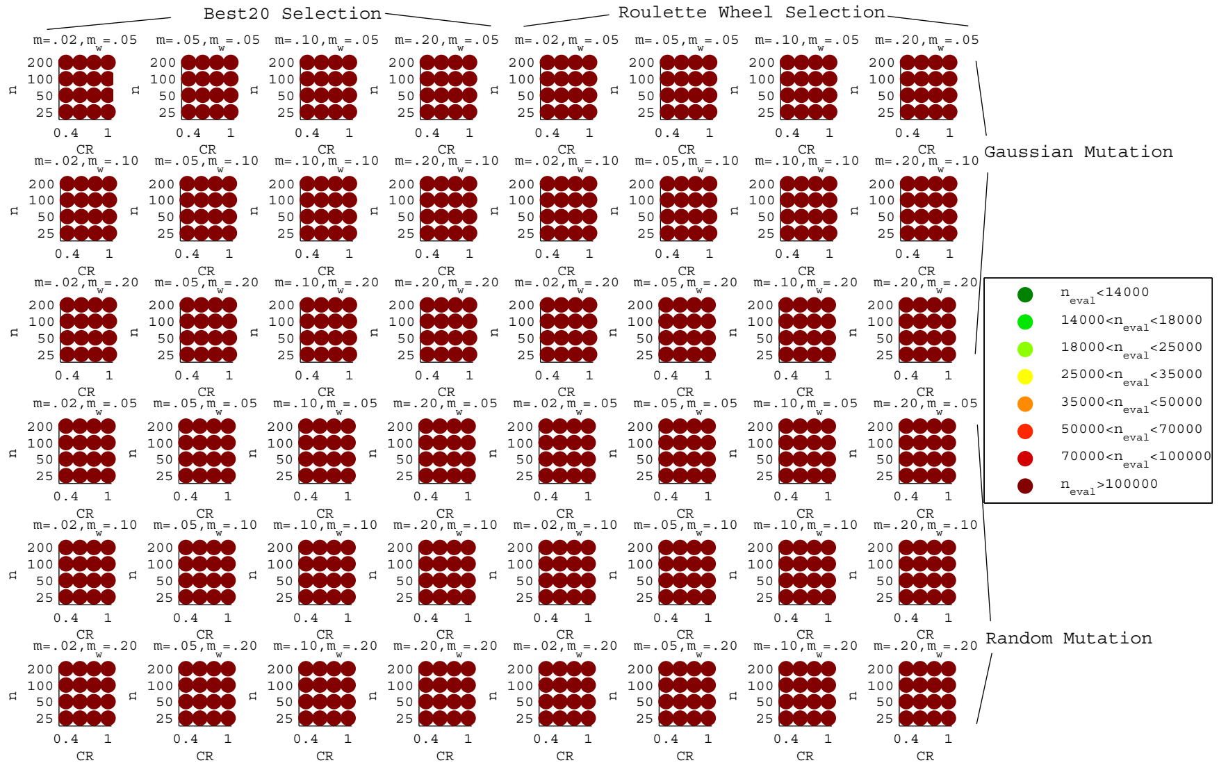
Figure B.5: The results of the first phase tuning process of GA on the Cassini2 First Leg VF problem. The results show the number of function evaluations that are required to obtain a 95% chance on finding a solution within 50 m/s of the best putative minimum. The results are categorized based on the color scheme visible on the right. The categorization is similar to that of the DE tuning, to allow for comparison. It is emphasized here that the categorization above 20000 evaluations is not necessarily correct: only 20000 evaluations were performed in each run, and algorithms that reliably converge after 20000 evaluations are underestimated in this plot. Note that n_{eval} in the legend is identical to n_{95\%} .
