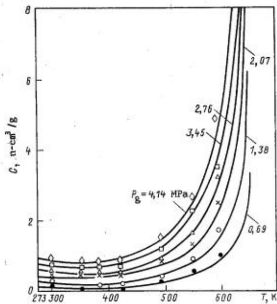
Figure 13 – Experimental concentration of hydrogen in water at varying  $p$  and  $T$ .
