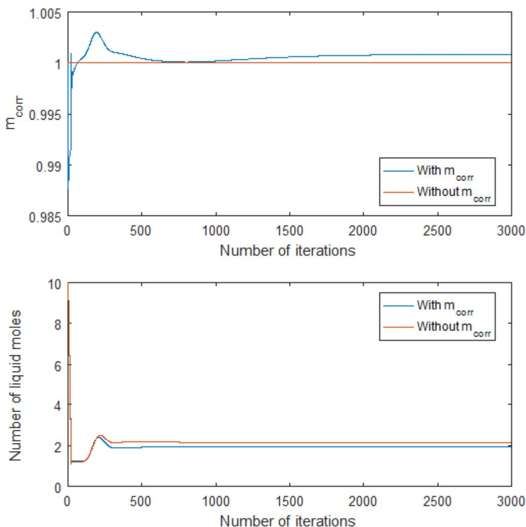
Figure 10 – Mass correction factor and number of liquid moles
