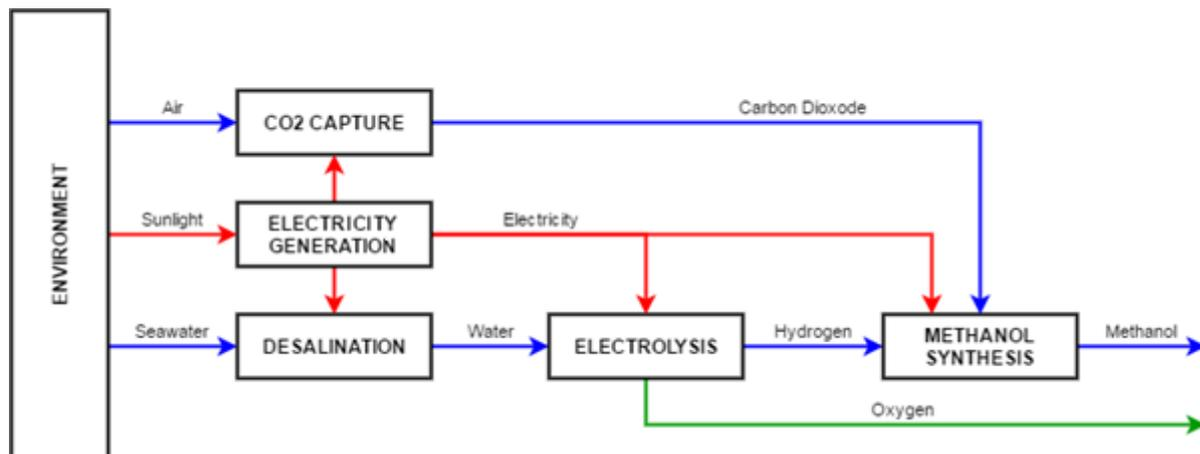
Figure 3 – Flowchart representation of the process in the DOS
