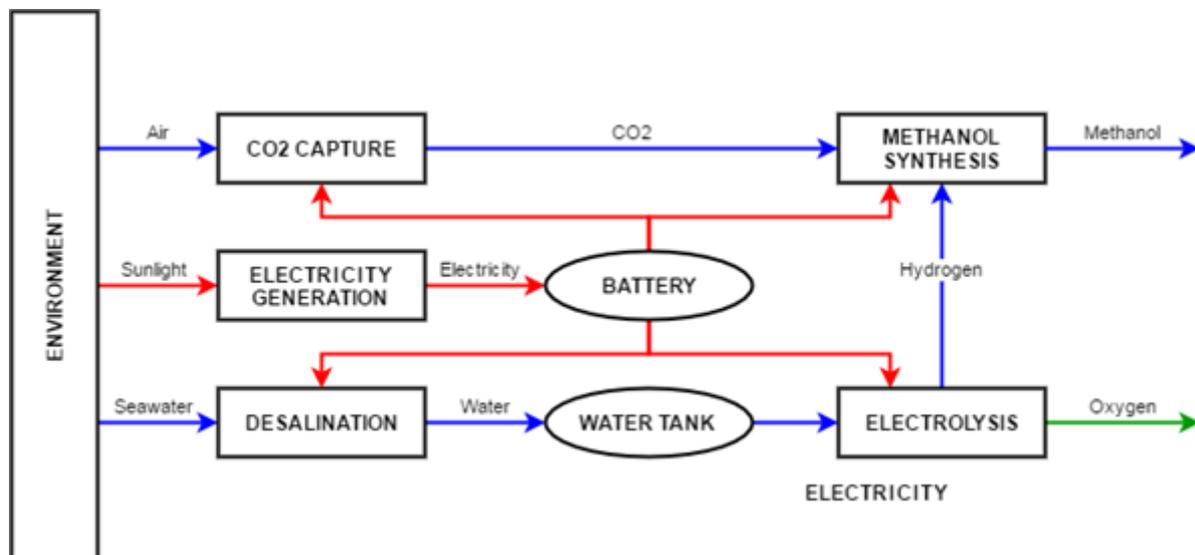
Figure 5 – Flowchart representation of the process of the DS
