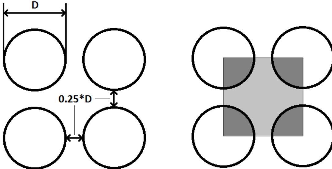
Figure 14 – Reactor tube configuration
