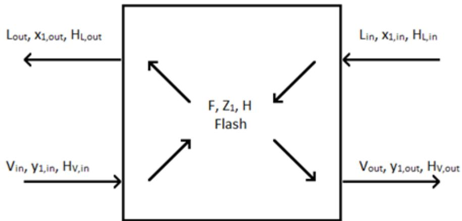
Figure 7 – Single cell material and energy balance
