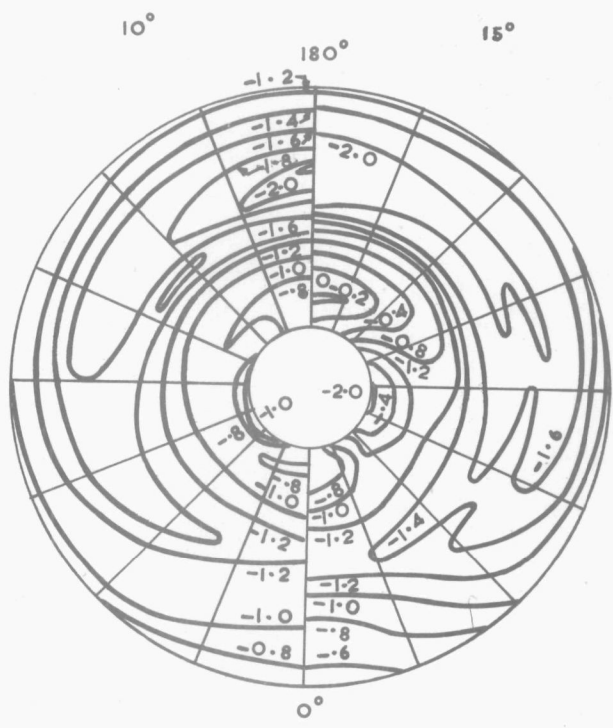
FIG. 2h. BASE PRESSURE DISTRIBUTION C_J = 40
