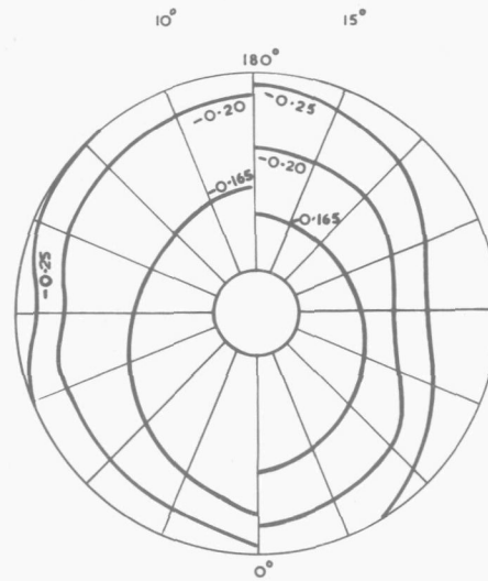
BASE PRESSURE DISTRIBUTION C_j=0
