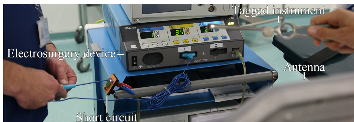
Figure 3.2: Evaluating the occurrence of reciprocal interference between the electrosurgery device and the antenna. The antenna is facing towards the electrosurgery device and a tagged instrument is located within the detection range of the antenna while the use of electrosurgery was being imitated.
