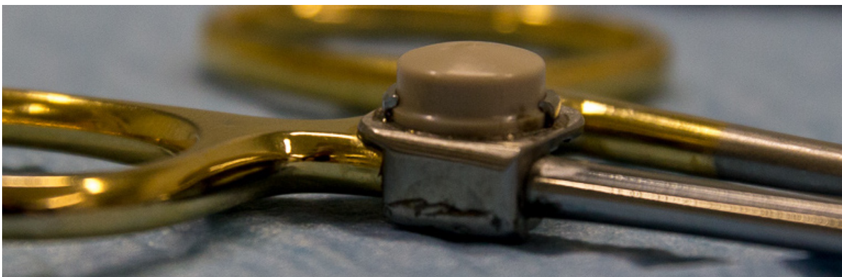
Figure 5.1: Original attachment of a tag to an instrument, showing two stainless steel counterparts welded together. The tag is encapsulated by epoxy to prevent damaging.
