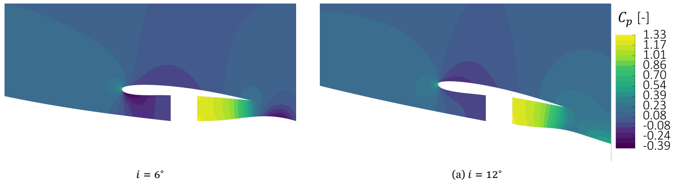
Figure 5.5: Static pressure contours for two levels of conicity. Both designs have the same fan mass flow rate
