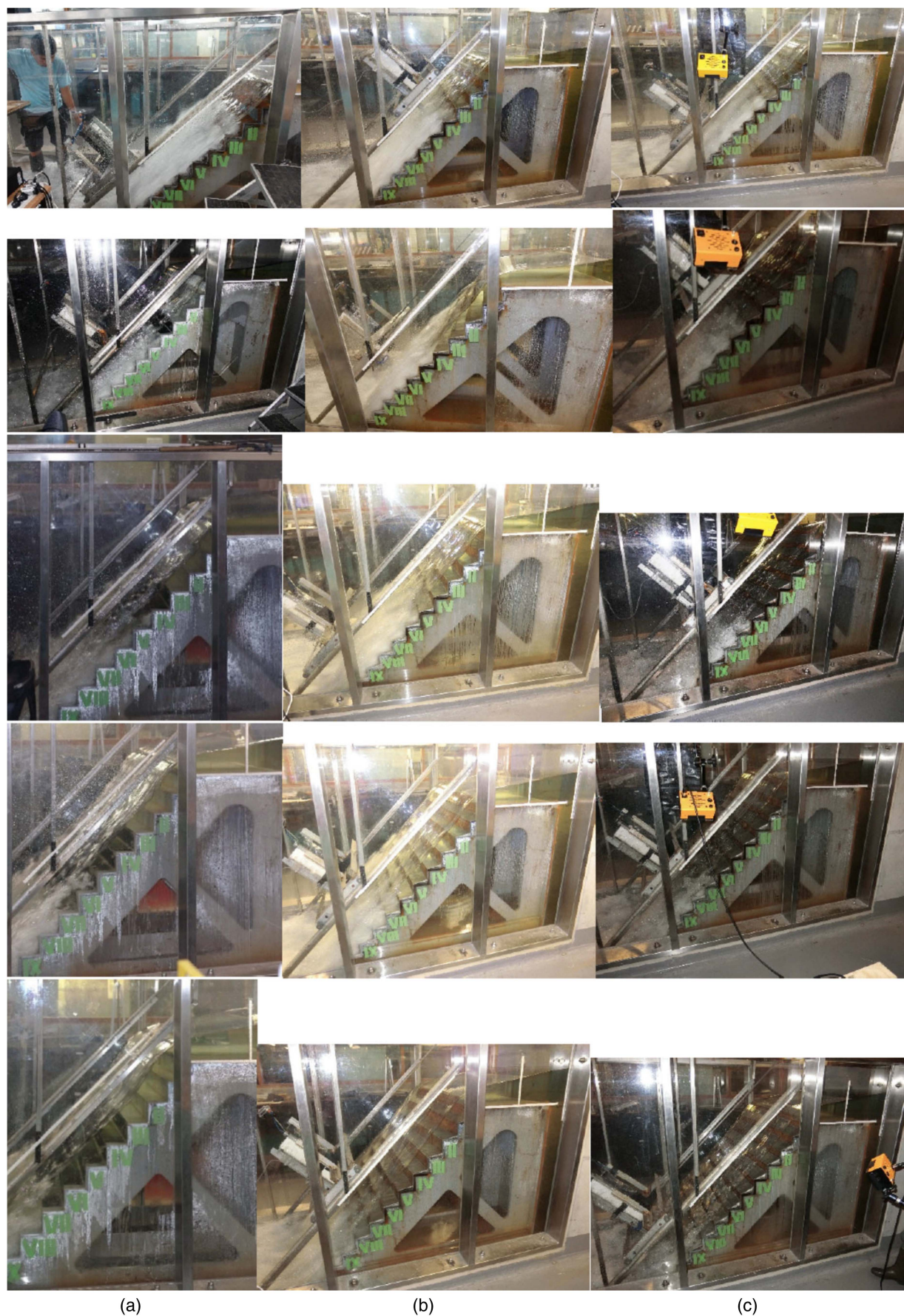
Fig. 4. Effects of the dimensionless discharge on 45° stepped chute with horizontal and inclined steps. From top to bottom: d_c/h = 0.8, 1.0, 1.2, 1.4 , and 1.6 ; (a) flat horizontal steps ( \delta = 0 and \lambda/k = 2.0 ); (b) 1V:5H inclined steps ( \delta = 11.3^\circ and \lambda/k = 2.5 ); and (c) 1V:2.3H inclined steps ( \delta = 23.3^\circ and \lambda/k = 3.0 ).
