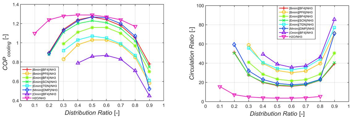
Fig. 5. Influence of  $DR$  on the  $COP$  for the selected  $NH_3/IL$  working pairs in a cooling application of DE-AHP
