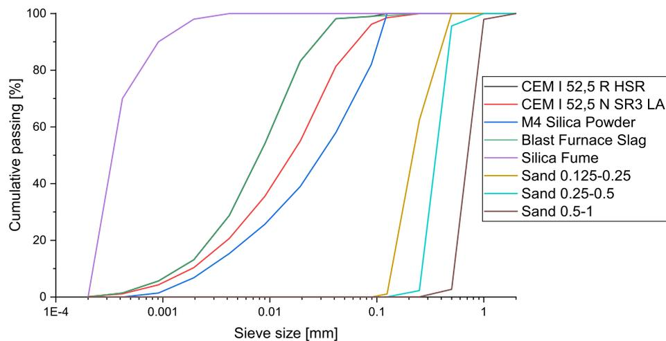
Figure 3.2: Particle size distribution curves of all granular materials used in research
