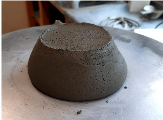
(a) Flow table specimen using CEM I 52.5 R right after lifting cone (M3)
