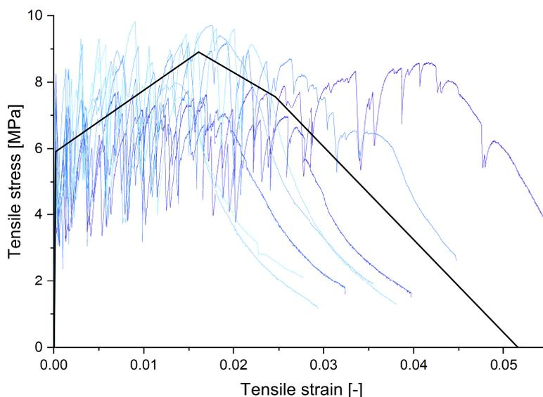
Figure 4.8: Material input for SH-UHPFRC based on experimental outcomes
