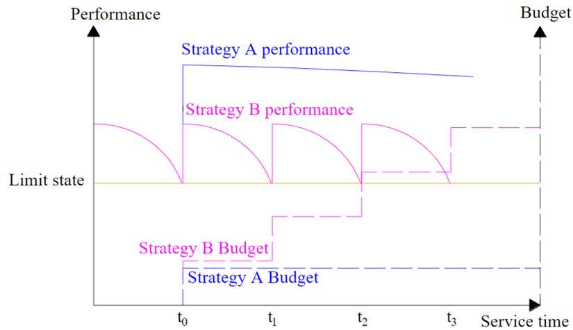
Figure 1.1: Comparison of different strengthening strategies: strengthening using UHPFRC (Strategy A) or using NC (Strategy B), based on performance and costs [6, 7]
