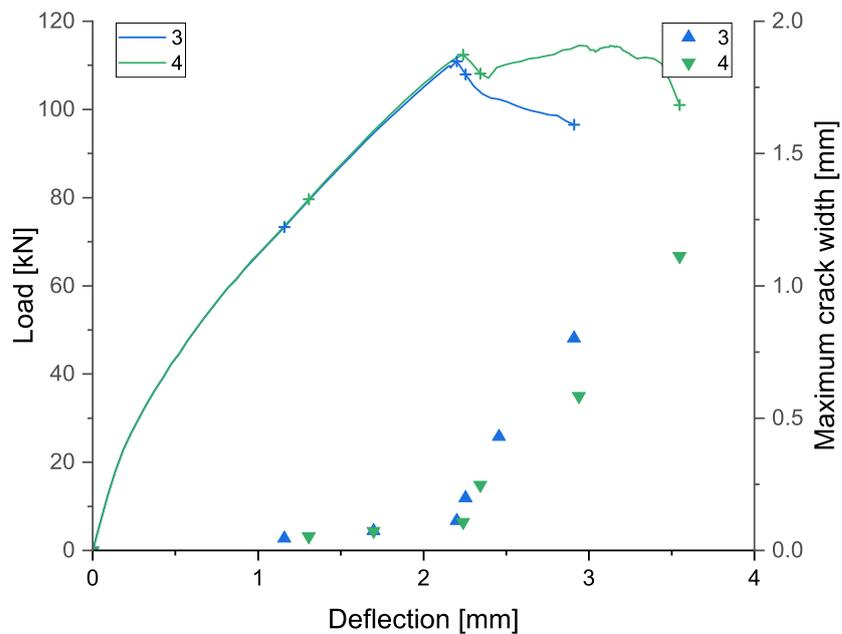
Figure 4.14: Load-deflection curve of Material Models 3 and 4 including crack width development. Characteristic points indicated by +
