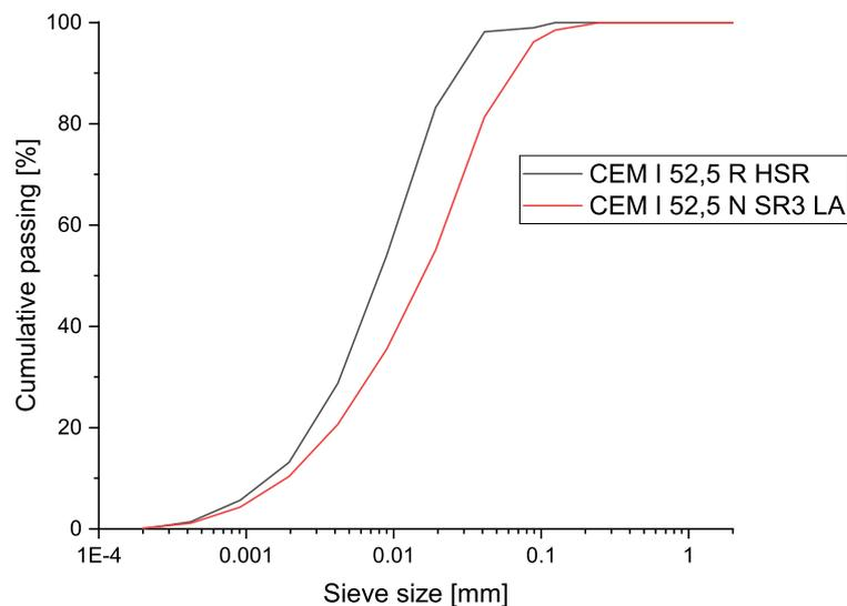
Figure 3.1: Particle Size Distribution curves of all dry materials used in research
