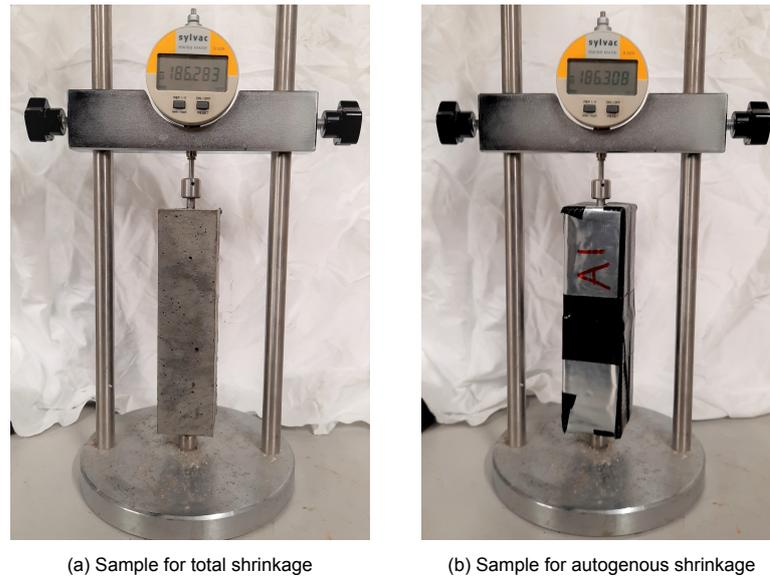
Figure 3.8: Setup for length measurement for shrinkage
