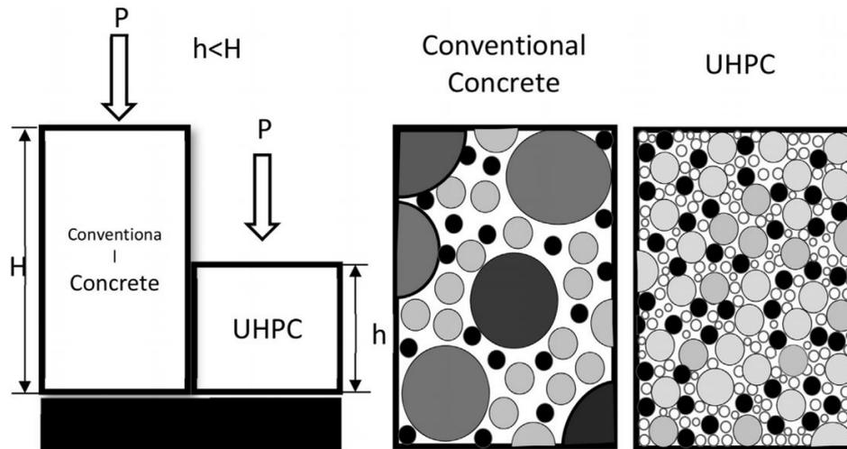
Figure 2.1: Conventional concrete (NC) versus UHPC [14]
