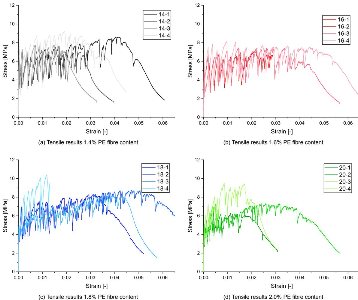
Figure 3.20: Tensile stress-strain results of direct tensile testing using different fibre contents
