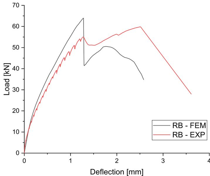
Figure 4.6: Load-deflection curves of the experimental and numerical RB for three point bending test
