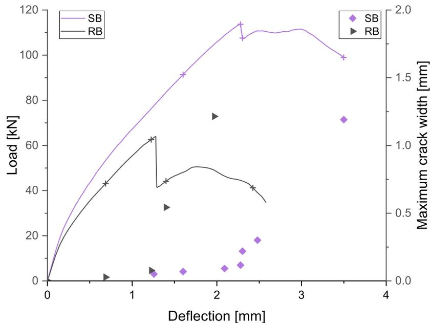
Figure 4.9: Load-deflection curve of the reference beam (RB) versus the strengthened beam (SB) including crack width development. Characteristic points indicated by +
