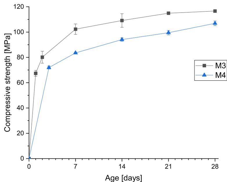
Figure 3.14: Compressive strength development over time of mixtures using different cement types
