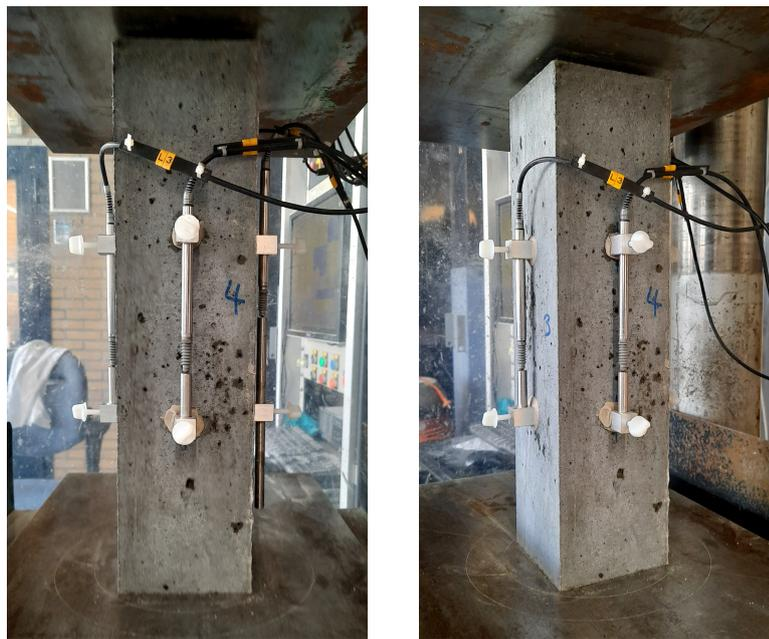
Figure 3.7: Setup for E-modulus measurement using TONI bank
