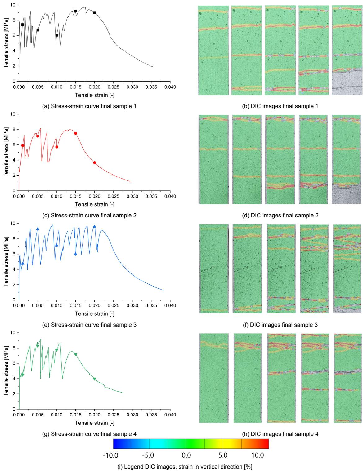
Figure 3.24: Stress-strain curves of samples using the final mixtures, accompanied by DIC images corresponding to the load situations as indicated by the symbols in the stress-strain curves.
