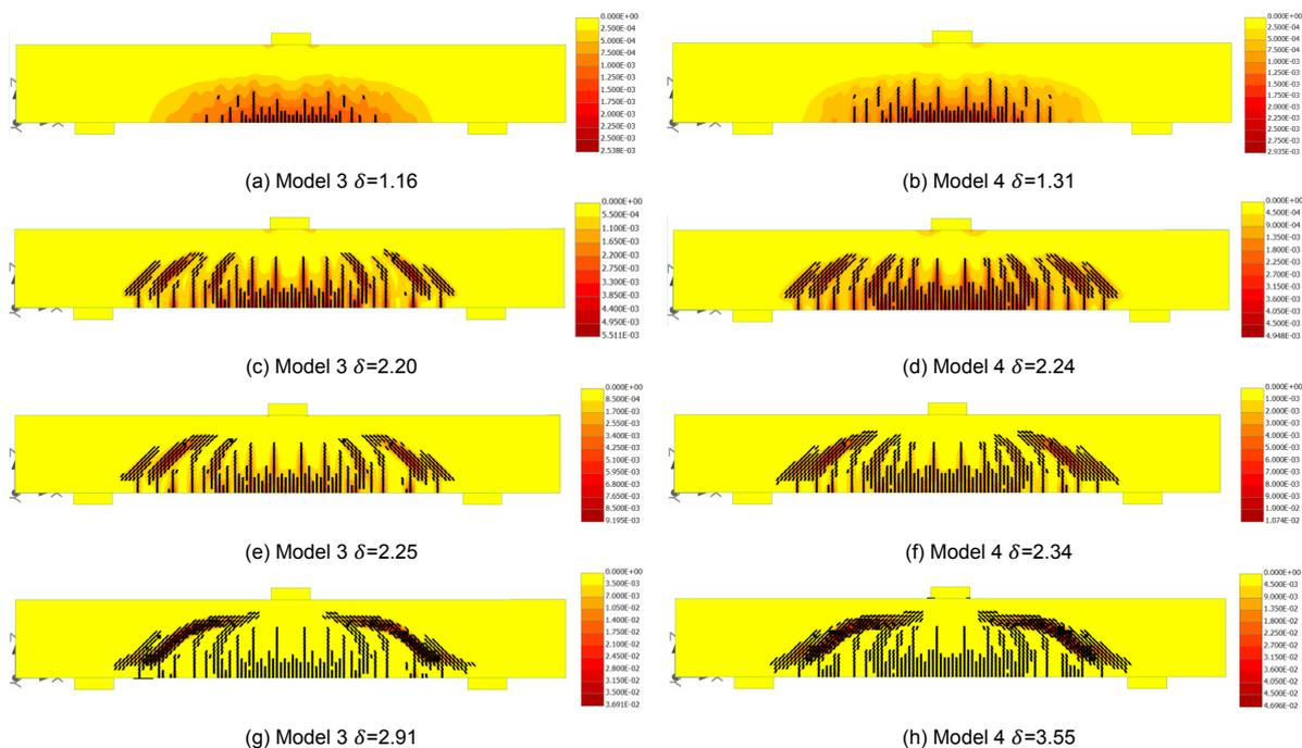
Figure 4.15: Crack pattern development of beam strengthened with materials using Material Models 3 and 4, with principal strain in ISO areas. Deflection  $\delta$  in mm, minimum visible crack width 0.01 mm.
