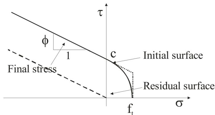
Figure 2.6: Failure surface for interface elements [105]
