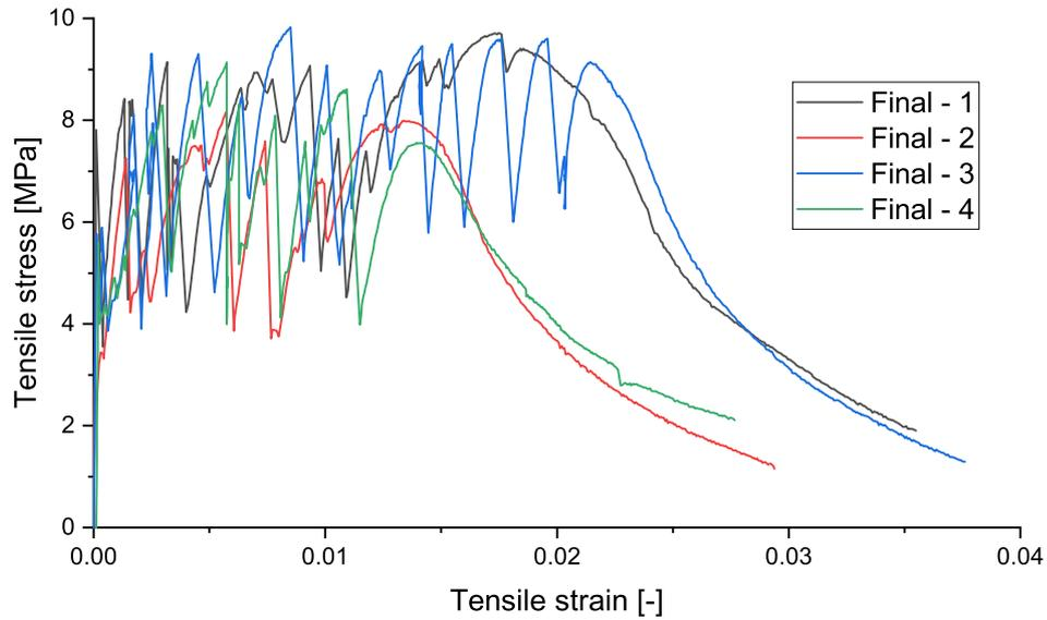
Figure 3.23: Tensile response of samples using the final mixture
