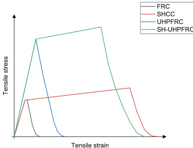
Figure 1.3: Schematic tensile constitutive behaviour of different concrete types
