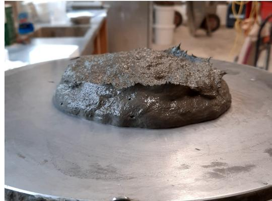
(b) Flow table specimen using CEM I 52.5 N right after lifting cone (M4)
