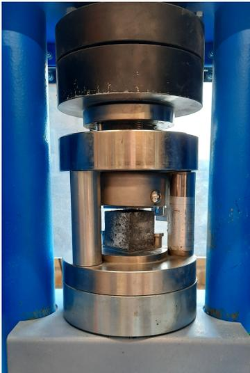
Figure 3.3: Setup compressive strength test 40 mm cubes
