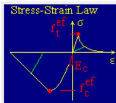
Figure 4.4: Modelled stress-strain relation NC
