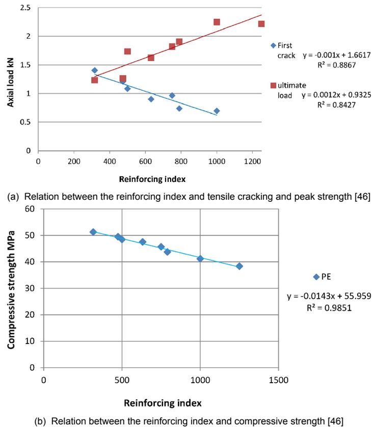
Figure 2.4: Relation between reinforcing index and mechanical properties as found by Said and Razak [46]
