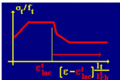
Figure 4.5: Input tensile stress-strain relation strengthening material
