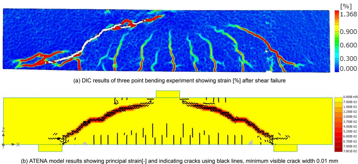
Figure 4.7: Comparison of the cracking pattern between experimental result (a) and numerical result (b)
