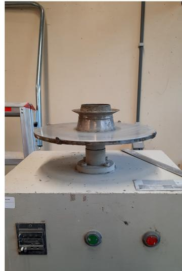
Figure 3.4: Setup flow table test
