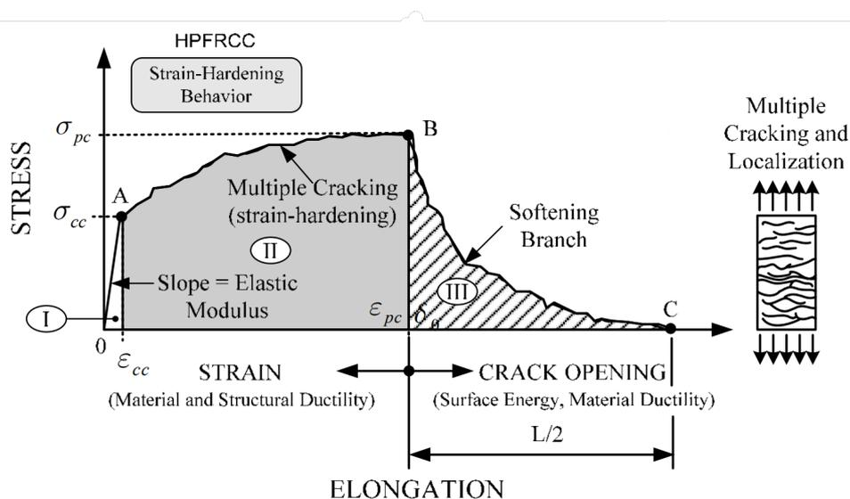
Figure 2.2: Typical stress-strain curve in tension up to complete separation of strain-hardening FRC or HPFRCC [9]
