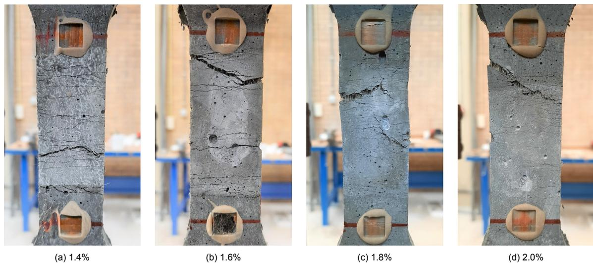
Figure 3.21: Final cracking patterns after direct tensile loading, using different fibre contents
