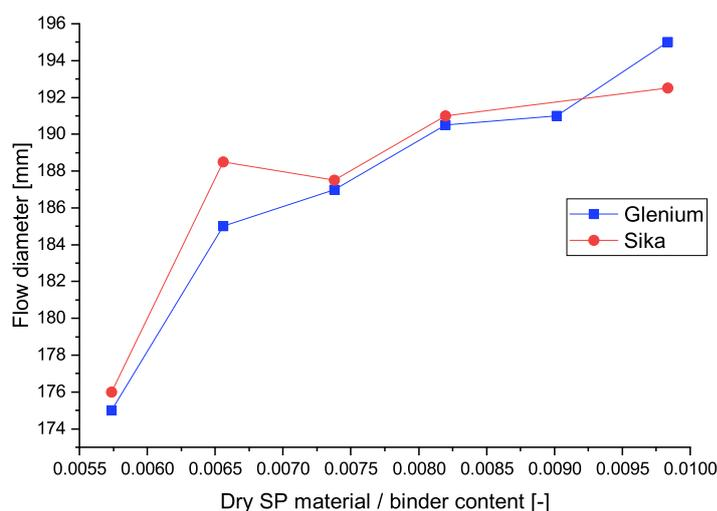
Figure 3.17: Effect of type and amount of SP on the flow diameter
