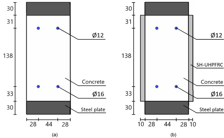
Figure 4.2: Transverse dimensions for reference beam (a) and strengthened beam (b). Dimensions in mm
