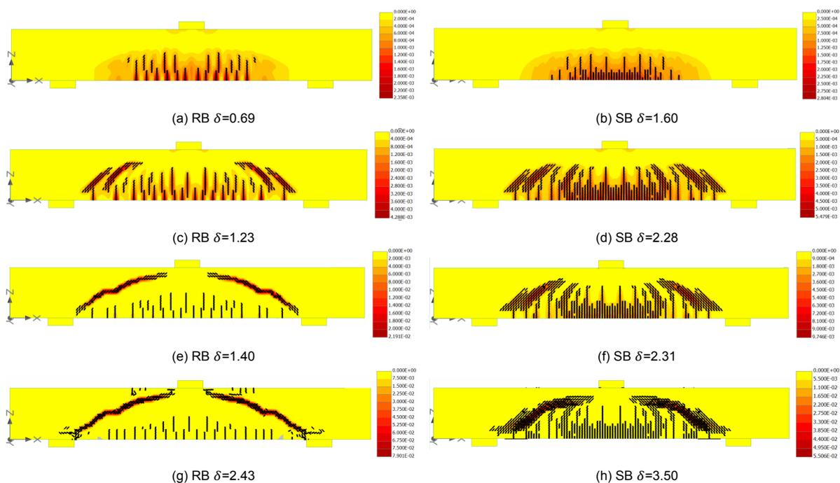
Figure 4.10: Crack pattern development reference beam versus strengthened beam with principal strain in ISO areas. Deflection  $\delta$  in mm, minimum visible crack width 0.01 mm.
