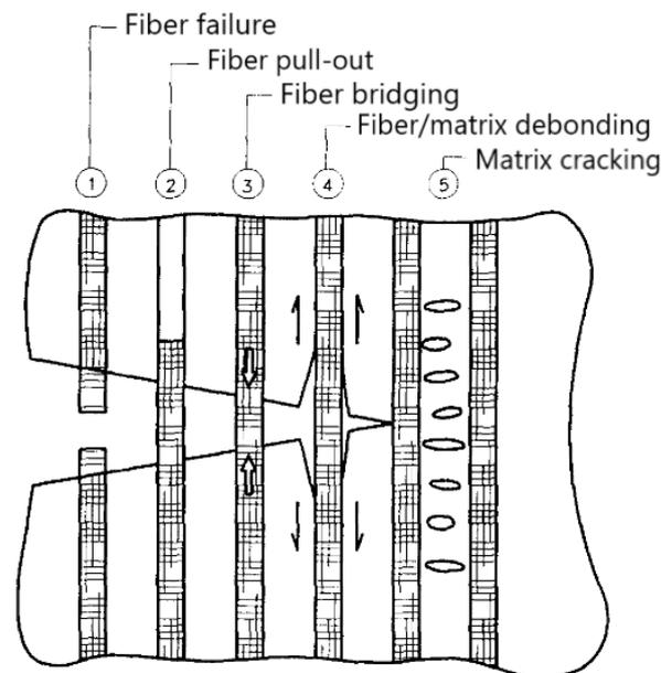
Figure 2.3: Fiber-matrix failure mechanisms [55]
