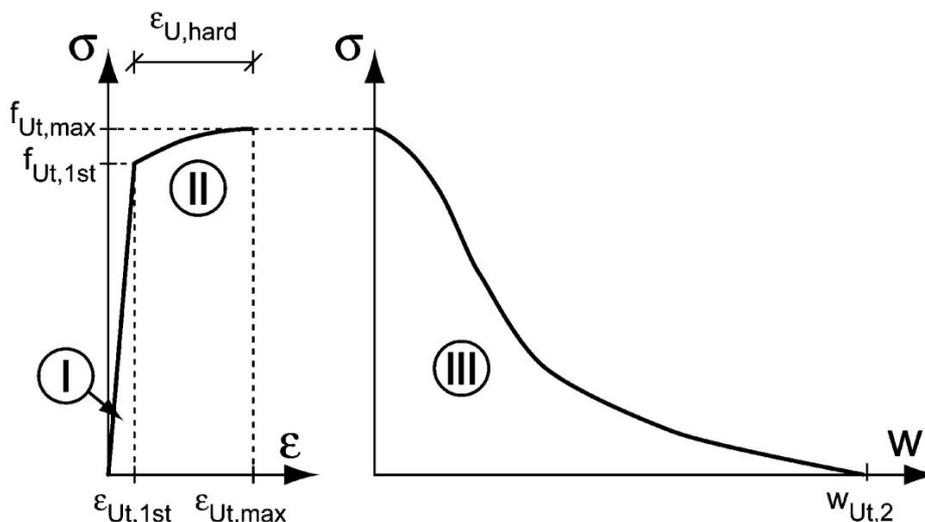
Figure 2.5: Schematic description of the tensile behaviour of UHPFRC: I) linear-elastic stress rise, II) domain of strain hardening and distributed macrocracking, III) softening behaviour and crack localization [83]
