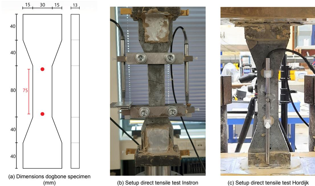
Figure 3.5: Direct tensile testing setup. Dimensions of dogbone specimen displayed in mm. The red dots indicate the location of attachment for strain gauges.
