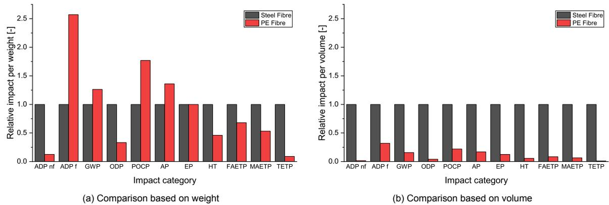
Figure 5.2: Relative environmental impact of PE fibres compared to steel fibres based on weight and volume
