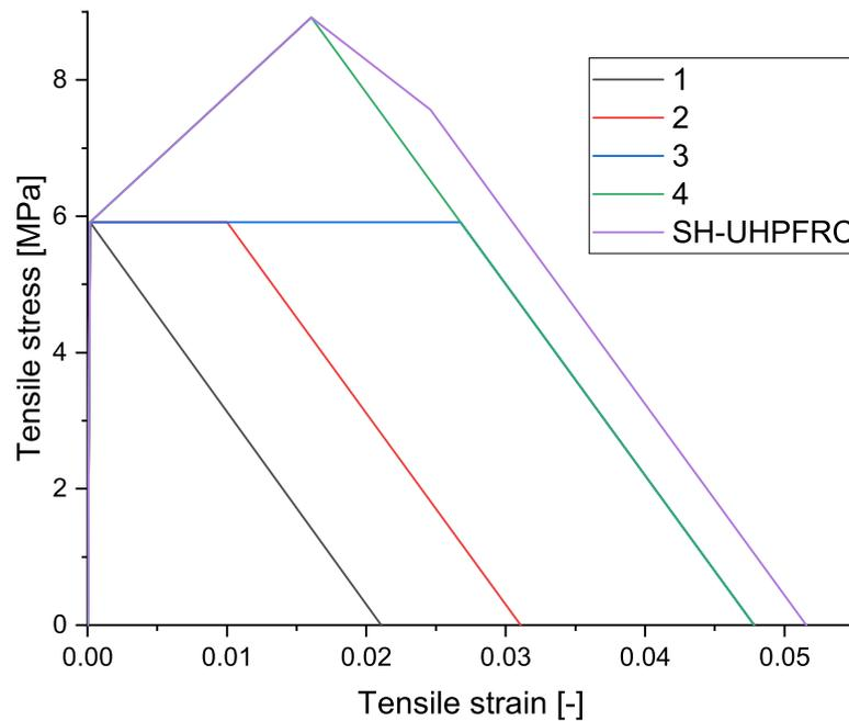
Figure 4.11: Tensile behaviour for different material models used in parametric study
