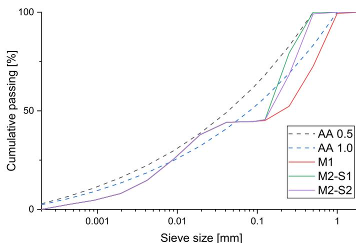
Figure 3.13: PSDs of mixtures for determination of the effect of different sand fractions on mechanical properties
