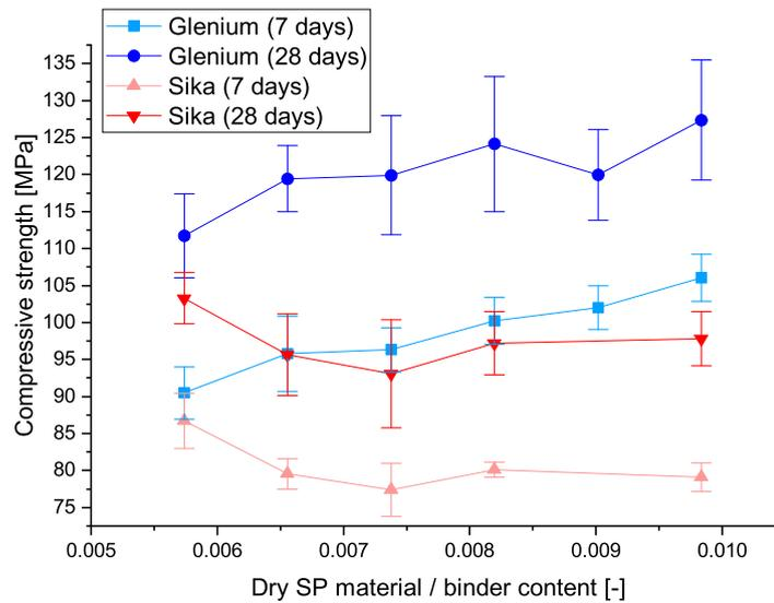
Figure 3.18: Effect of type and amount of SP on the compressive strength at 7 and 28 days
