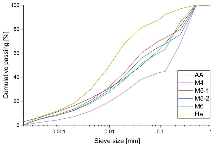
Figure 3.16: PSD curves of mixtures for packing and paste content comparison
