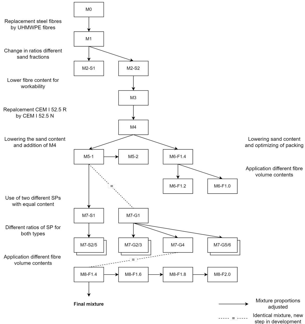
Figure 3.10: Flow scheme mixture development
