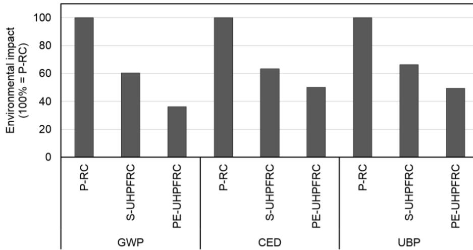
Figure 2.7: Normalized environmental impact over a life cycle of 100 years for different strengthening methods for a bridge deck. Calculated for three environmental impact factors: global warming potential (GWP), cumulative energy demand (CED) and ecological scarcity (UBP) [114]
