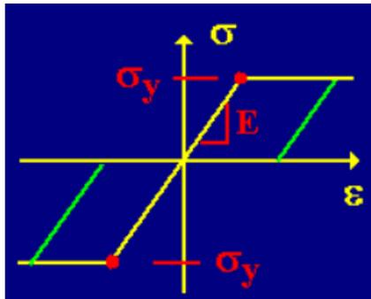
Figure 4.3: Modelled stress-strain relationship for steel reinforcement
