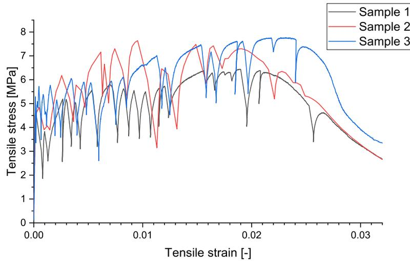
Figure 3.12: Direct tensile test results replicated mixture He et al. [80]
