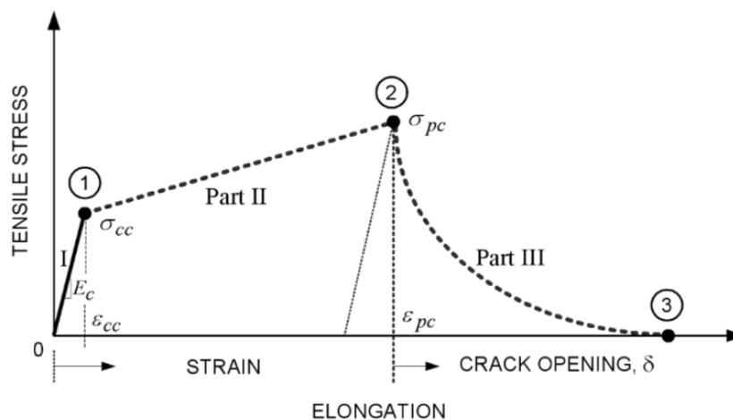
Figure 1.2: Idealized stress-elongation response in tension of a strain hardening FRC composite for modelling [11]
