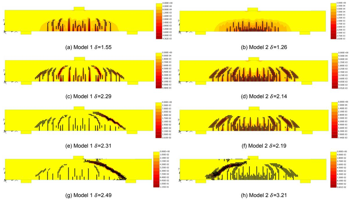
Figure 4.13: Crack pattern development of beam strengthened with materials using Material Models 1 and 2, with principal strain in ISO areas. Deflection  $\delta$  in mm, minimum visible crack width 0.01 mm.
