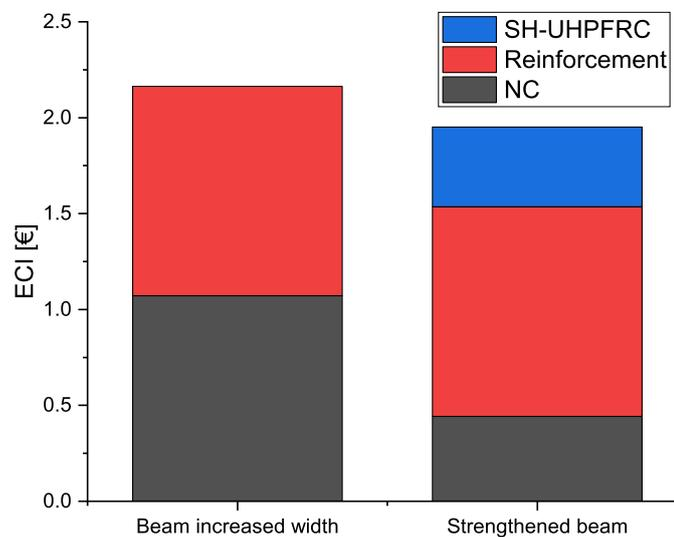
Figure 5.4: ECI for materials used in the widened beam and the strengthened beam
