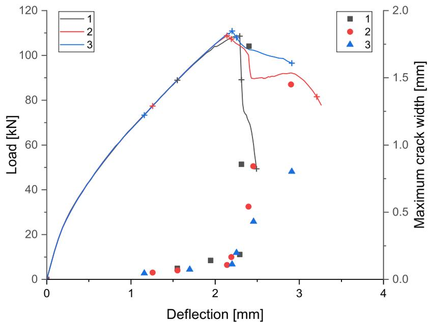
Figure 4.12: Load-deflection curve of Material Models 1-3 including crack width development. Characteristic points indicated by +
