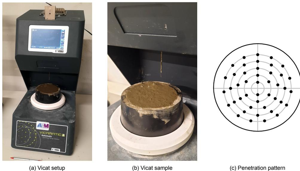
Figure 3.9: Vicat setup for setting time determination
