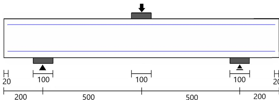
Figure 4.1: Longitudinal dimensions for the modelled beam. Dimensions in mm
