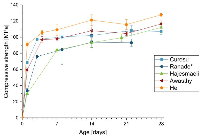
Figure 3.11: Compressive strength development of literature mixtures [39, 42, 80, 113, 115]. \*The mixture by Ranade does not include fibres.
