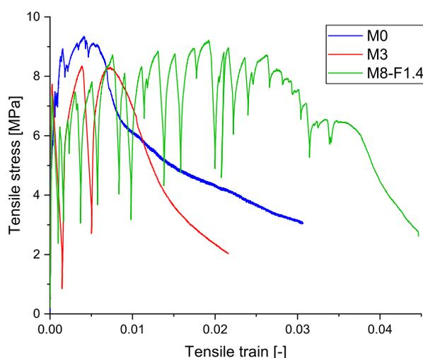
Figure 3.19: Direct tensile results of mixtures including steel or UHMWPE fibres
