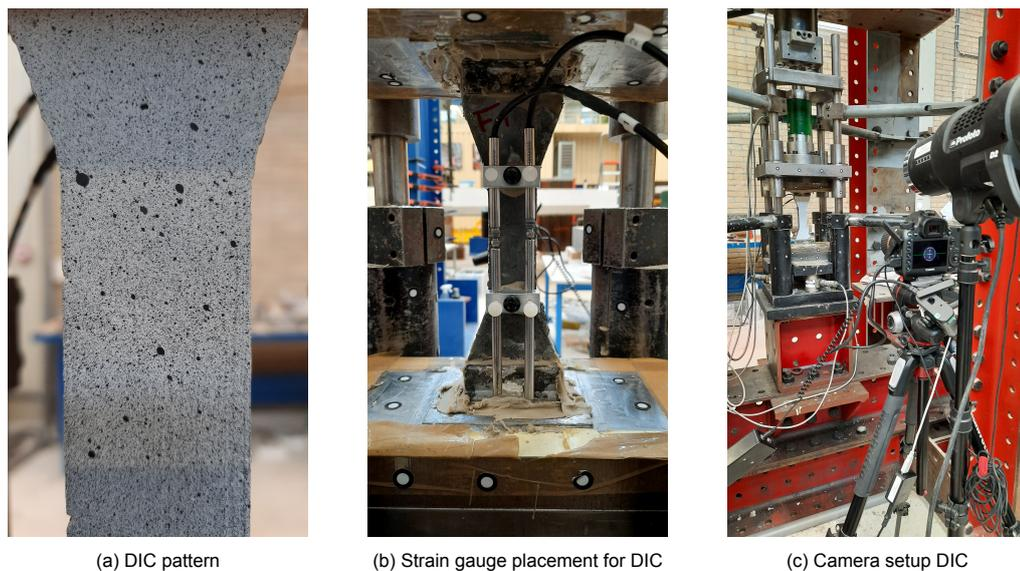
Figure 3.6: DIC direct tensile testing setup
