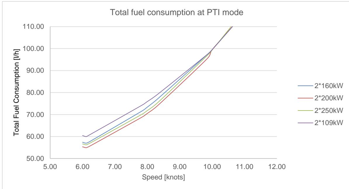
Figure 37: Total fuel consumption during PTI mode over the speed range for the four considered configurations
