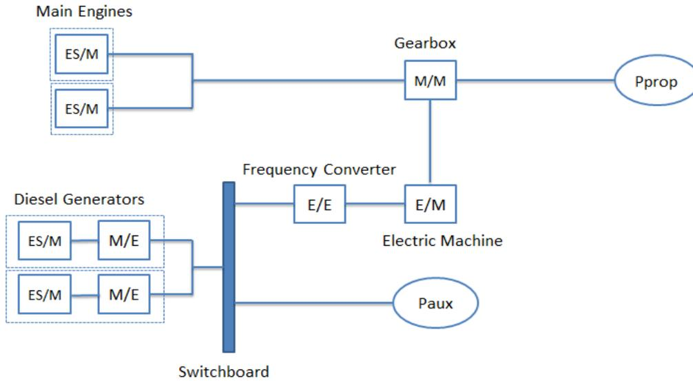
Figure 36: Energy Flow Diagram of the power plant of the new concept
