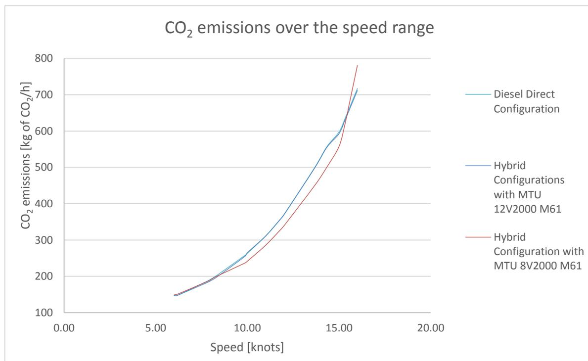
Figure 38: CO<sub>2</sub> emissions over the speed range for the three different configurations
