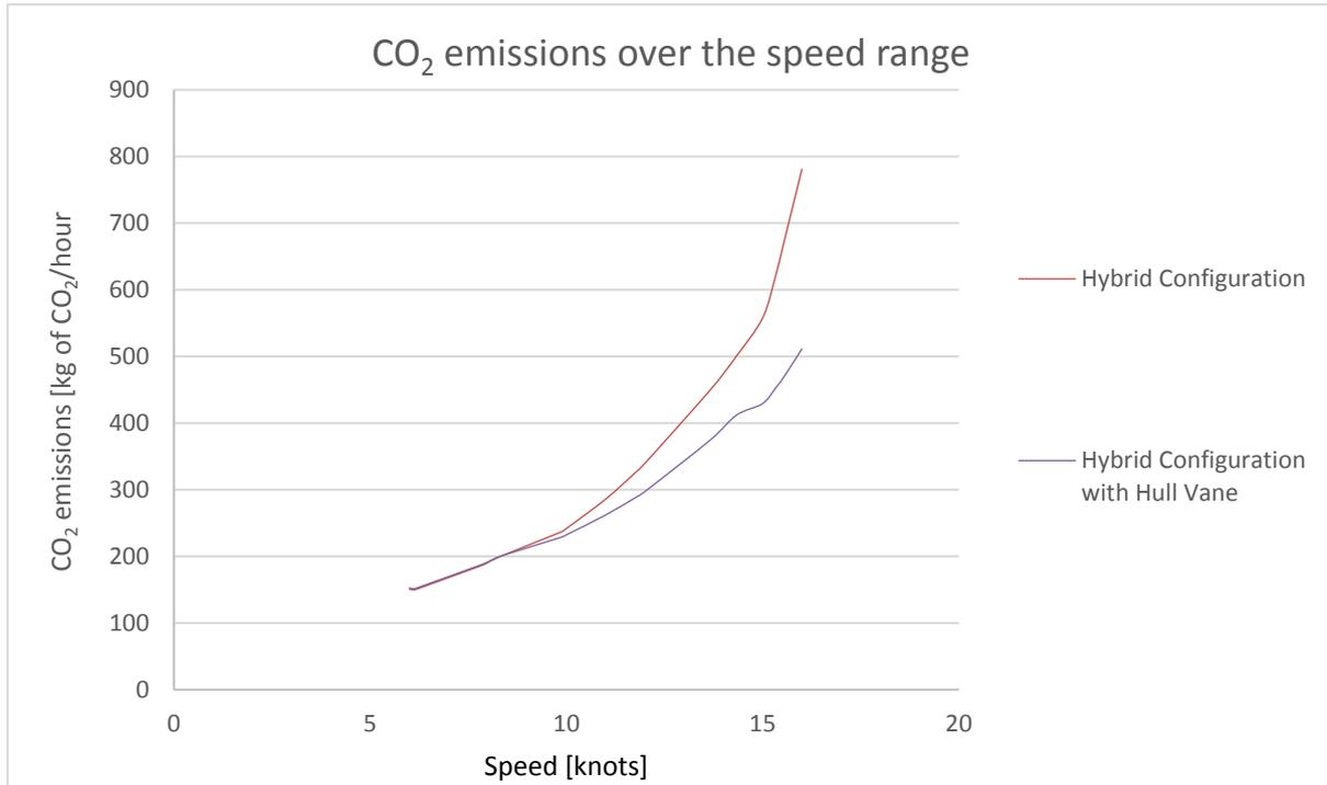
Figure 39: CO<sub>2</sub> emissions over the speed range of a hybrid configuration with and with Hull Vane®
