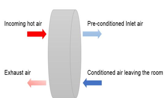
Figure 14: Scheme of a wheel heat exchanger
