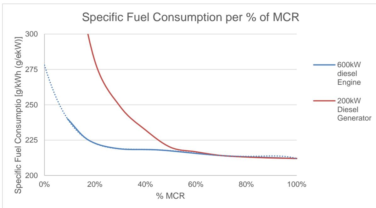
Figure 29: Specific fuel consumption comparison between medium size diesel engine and smaller diesel generator per percentage of maximum continuous rating
