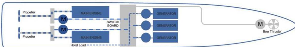
Figure 35: Hybrid propulsion arrangement in Boost PTI mode (8)
