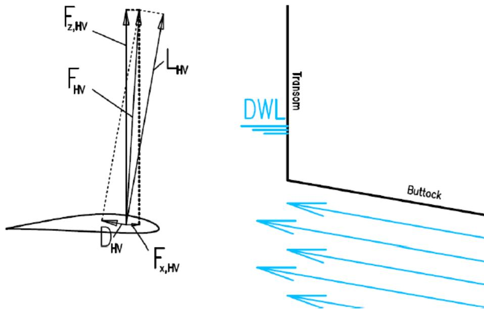
Figure 22: Schematic overview of the forces on the Hull Vane® in a section view of the aft ship
