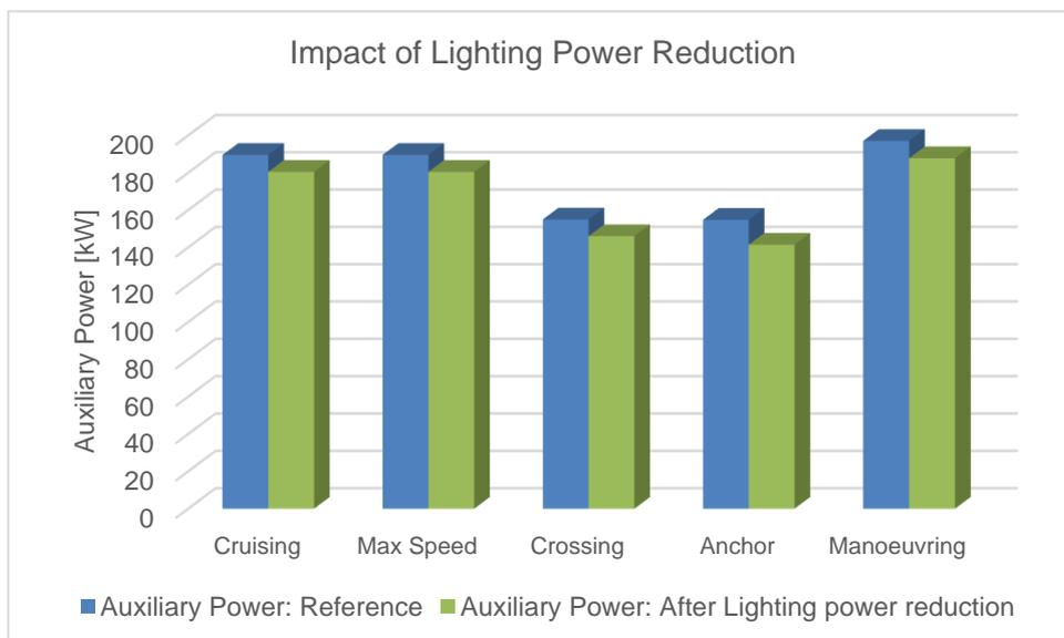
Figure 17: Comparison between auxiliary power of the reference design and of the new design after only Lighting power reduction
