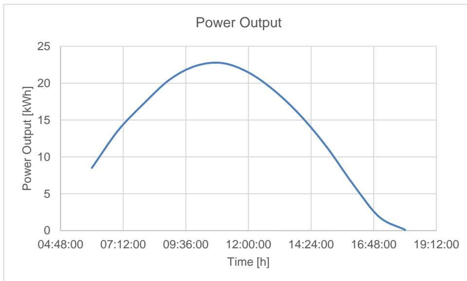
Figure 28: Power Output in optimal conditions of the total installed solar panel area
