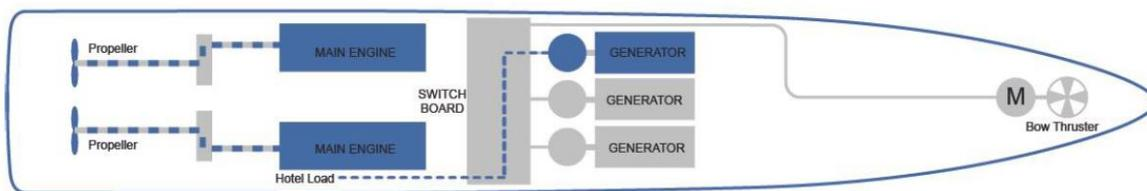
Figure 31: Diesel Direct typical configuration (8)
