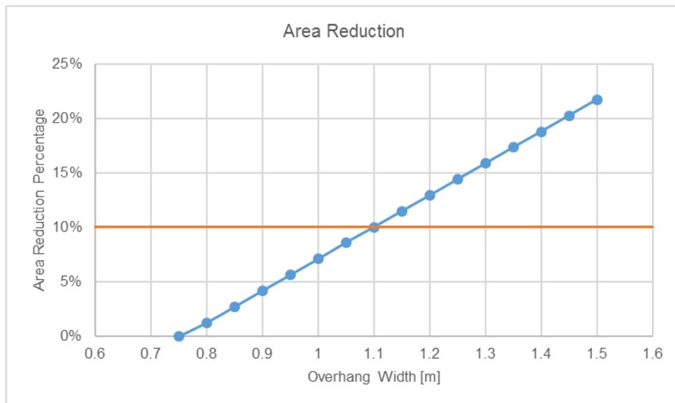
Figure 49: Area reduction percentage due to overhang width
