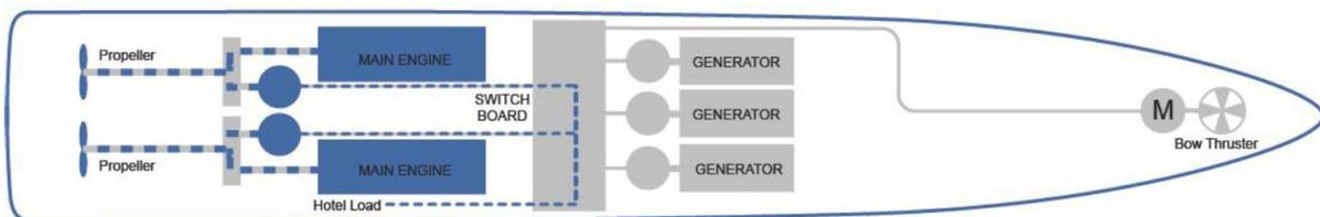
Figure 34: Hybrid propulsion arrangement in PTO mode (8)
