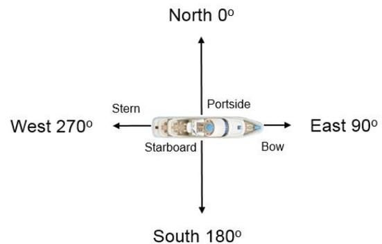
Figure 46: Yacht Orientation for Azimuth angle calculation
