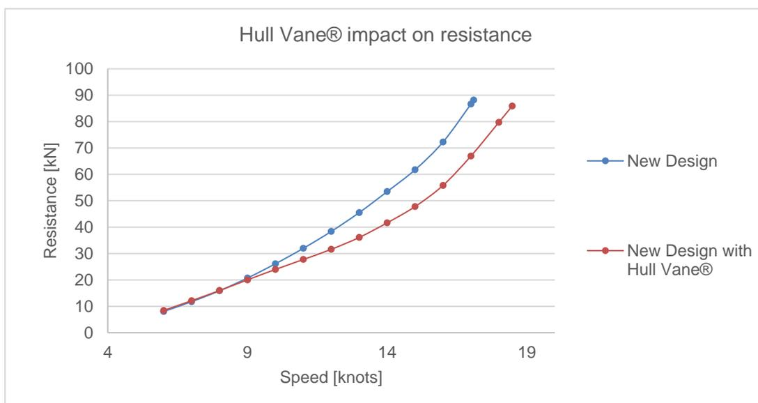
Figure 26: Resistance comparison between new design with and without Hull Vane®
