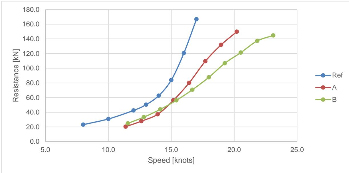
Figure 24: Performance comparison between reference design and aluminium fast displacement hull forms from database
