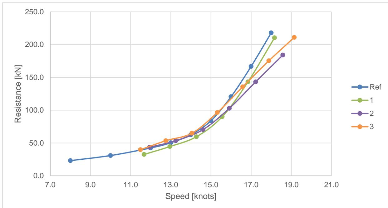
Figure 23: Performance comparison between reference design and steel fast displacement hull forms from database
