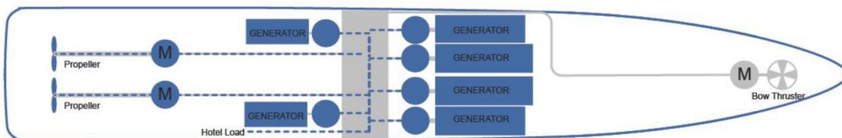
Figure 32: Diesel Electric Typical Configuration (8)
