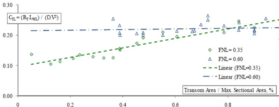
Figure 21: Dependency of resistance (in form of  $C_{TL}$ ) on the immersed transom area at Froude number of 0.35 and 0.60 (40)
