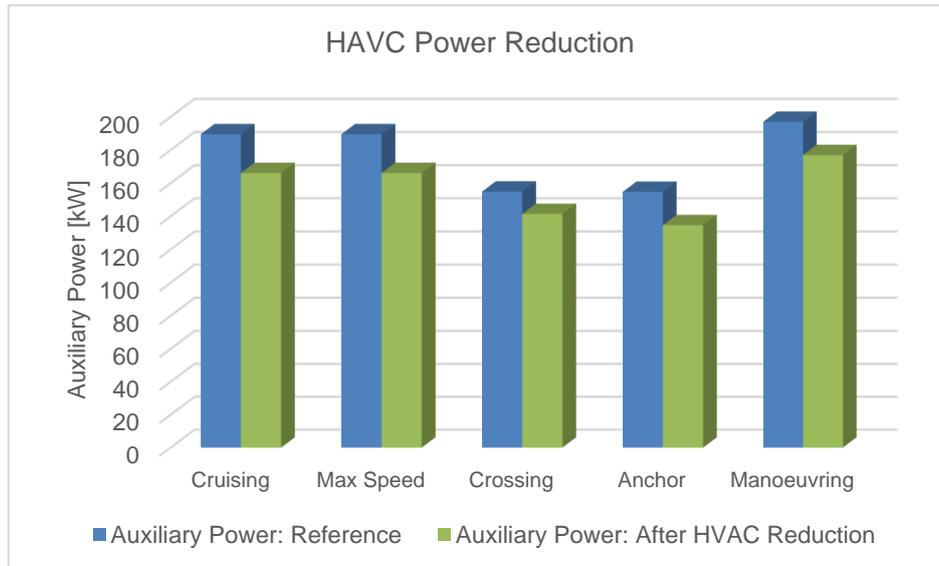
Figure 16: Comparison between Auxiliary power of the reference design and of the new design after HVAC power reduction
