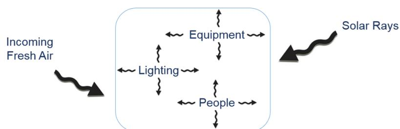
Figure 12: Schematic figure of the heat balance inside a yacht
