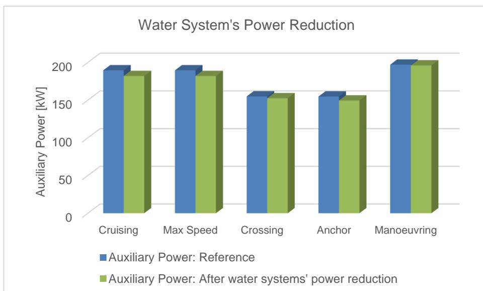
Figure 18: Comparison between auxiliary power of the reference design and of the new design after HVAC, lighting and water systems' power reduction
