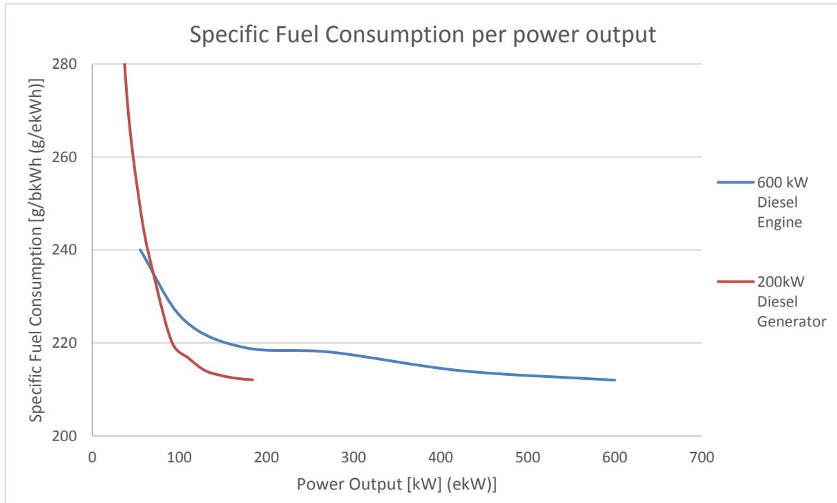
Figure 30: Specific fuel consumption per power output of medium size diesel engine in comparison with smaller generator
