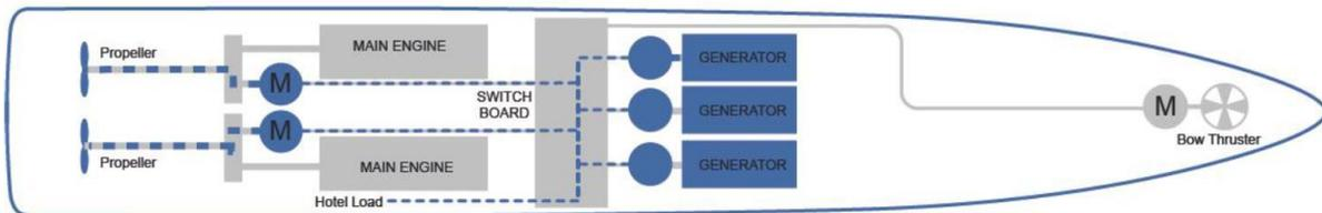
Figure 33: Hybrid propulsion arrangement in slow PTI mode (8)
