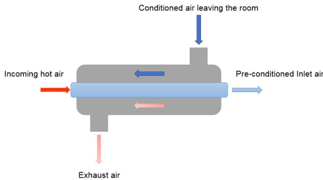
Figure 15: Scheme of a cross flow heat exchanger
