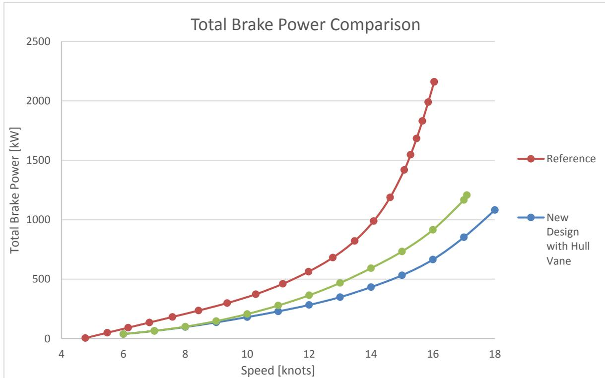
Figure 27: Total brake power demand comparison between the benchmark and the new design with and without the Hull Vane®
