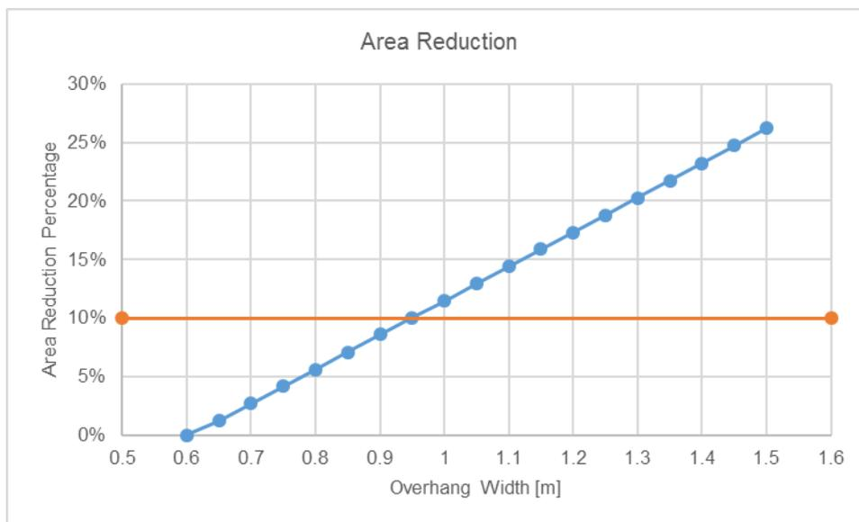
Figure 51: Area reduction percentage due to overhang width on wheelhouse deck
