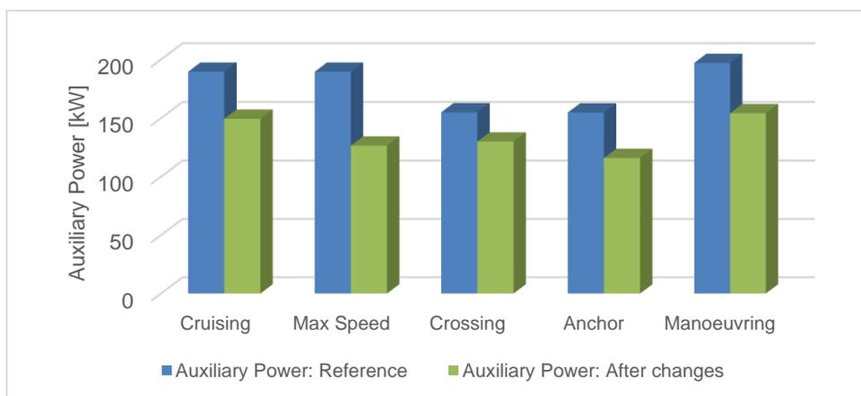
Figure 20: Comparison between auxiliary power of the reference design and of the new design after all changes and introduction of power management affect at maximum speed
