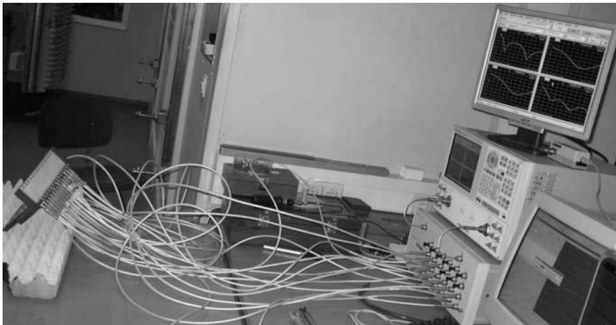
Figure 5.27: Reflection coefficient measurement set-up of the linear array of 15 CPW fed “Eared” antennas.
