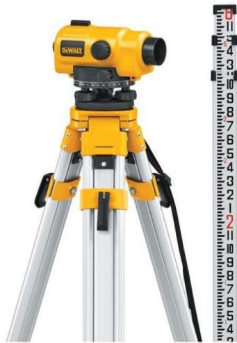
Figure 36 Level, an optical instrument to measure height differences (source:www.gereedschappelijk.nl)
