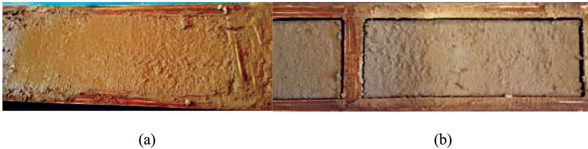
FIGURE 5. Picture of mortar just cast (a) and after five days since pouring (b): volumetric shrinkage of about 18% [26].
