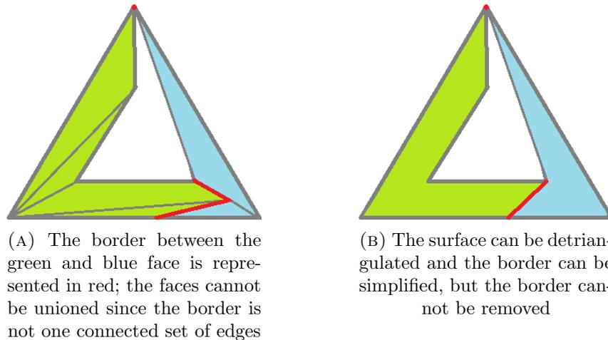
FIGURE 4.17: A coplanar surface before and after detriangulation (without creating holes) and simplification of the border
