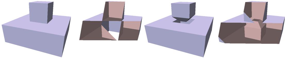
(A) The input geometry consisting of two view- (B) A cross-section of the input to repaired by subtracting (C) The edges are not repaired by union- (D) Instead, the edges are repaired by unioning elements, creating no gaps
