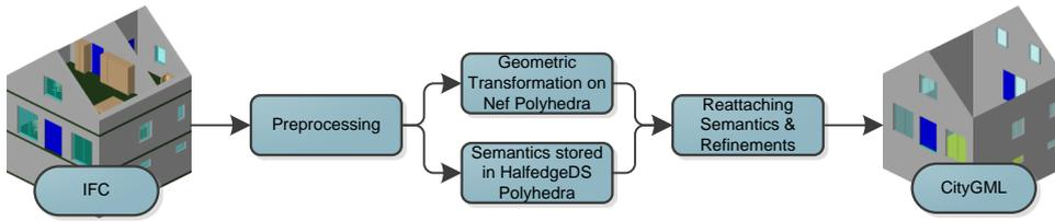
FIGURE 4.5: General workflow diagram for the implementation
