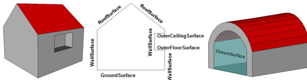
FIGURE 2.7: LoD3 boundary surfaces, no ‘Openings’ (Source: [36])
