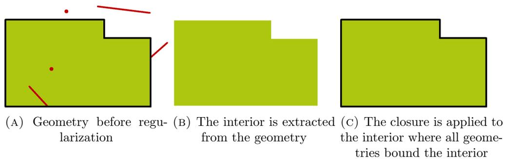
FIGURE 3.18: Regularization is applied to remove dangling geometries
