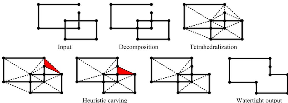
FIGURE 3.13: Heuristic carving a method for repairing geometry (Source: [50])
