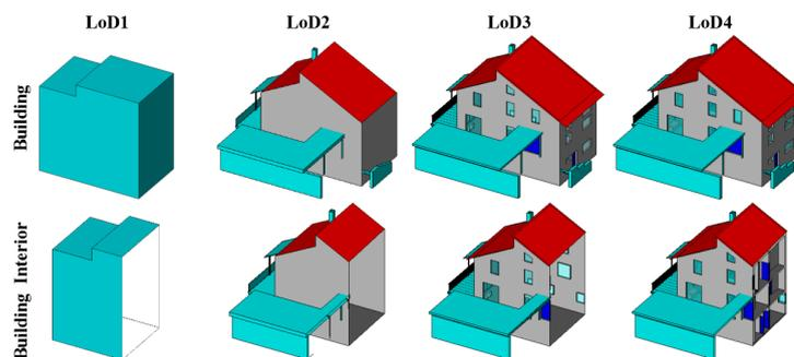
FIGURE 1.2: Building model in LoD1 to LoD4 (Source: [16])
