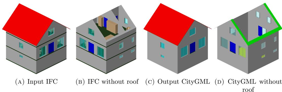
FIGURE 4.32: BIEN-ZENKER Jasmin-Sun input and conversion result
