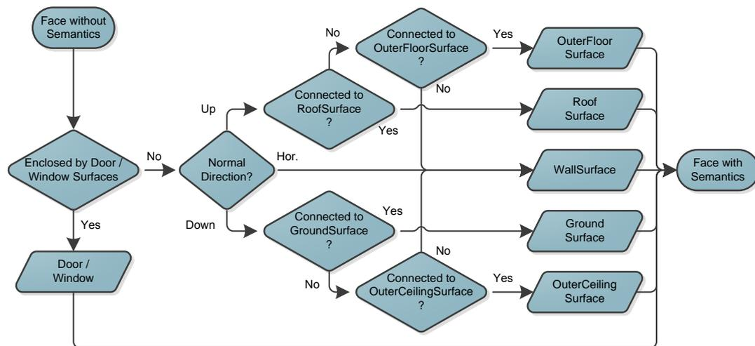
FIGURE 3.23: Workflow diagram for determining the semantics for faces without semantics
