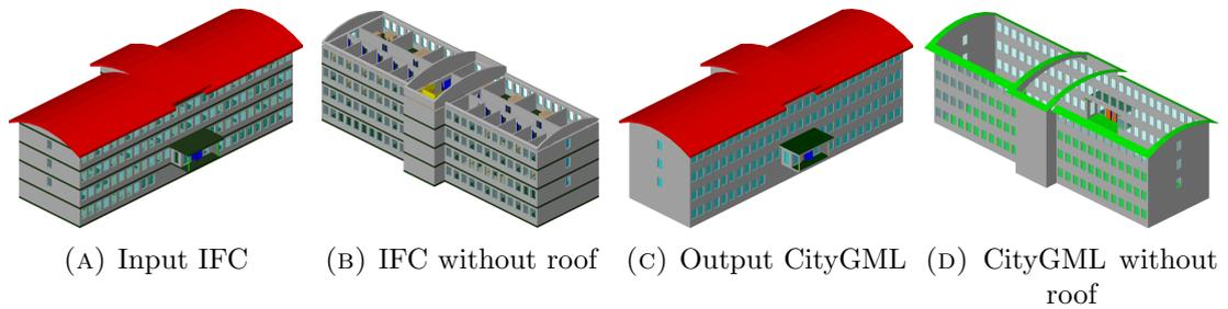
FIGURE 4.33: Office Building input and conversion result
