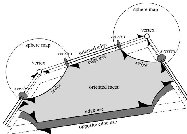
FIGURE 4.3: Two sphere maps, the SNC representation and connectivity of faces and edges for Nef polyhedra (Source: [65])
