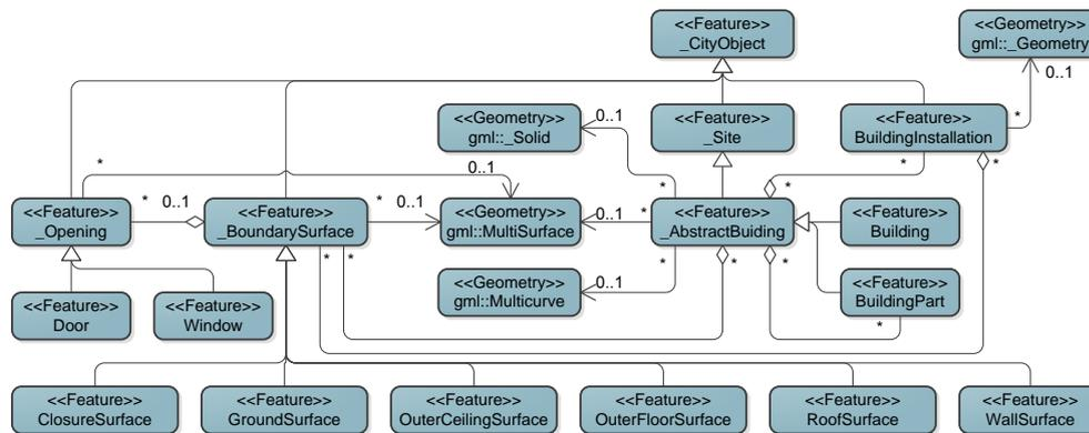
FIGURE 2.6: CityGML UML for LoD3 (Adapted from: [11])
