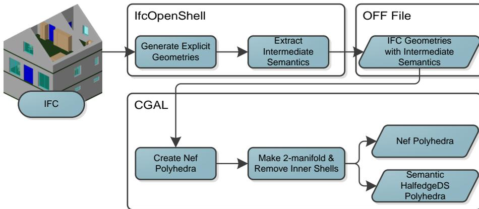
FIGURE 4.6: Flow diagram for the preprocessing stage of the implementation
