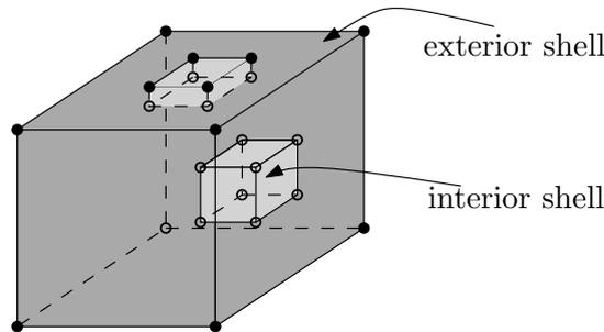
FIGURE 2.10: One solid with one exterior shell and one interior shell, a cavity (Source: [19])
