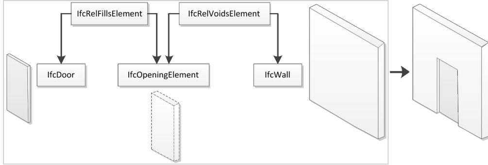
FIGURE 2.5: An example of implicit geometry: the wall is cut by the opening element using the Boolean difference. The door is then placed within the gap in the wall (Adapted from: [5])
