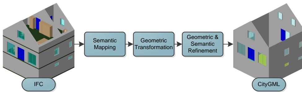
FIGURE 1.4: General workflow diagram of the prototype
