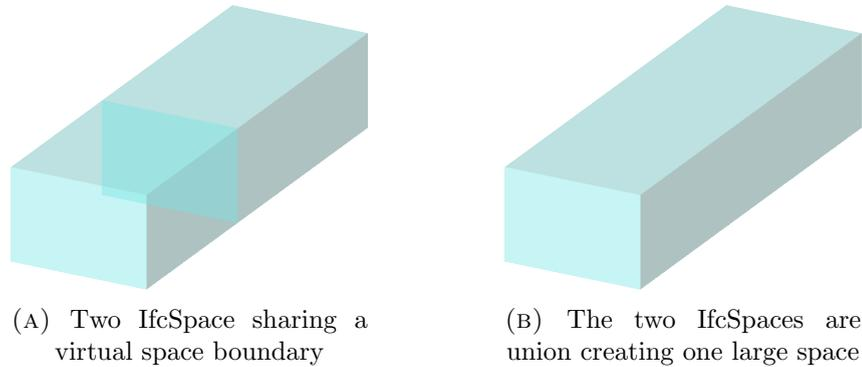
FIGURE 4.21: Connected spaces are union into large spaces
