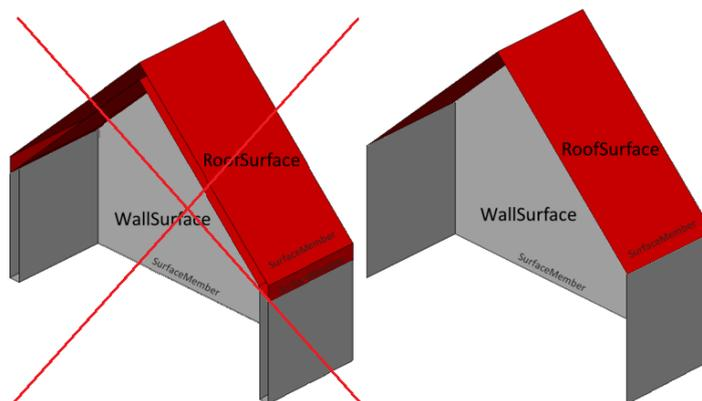
FIGURE 2.9: Only visible surfaces in CityGML (Adapted from: [36])
