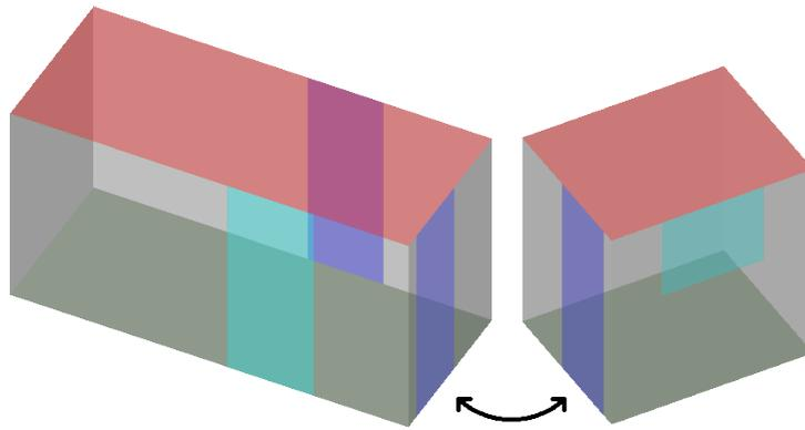
FIGURE 4.50: The Opening surfaces between room should either be linked using XLinks or linked at the semantic level
