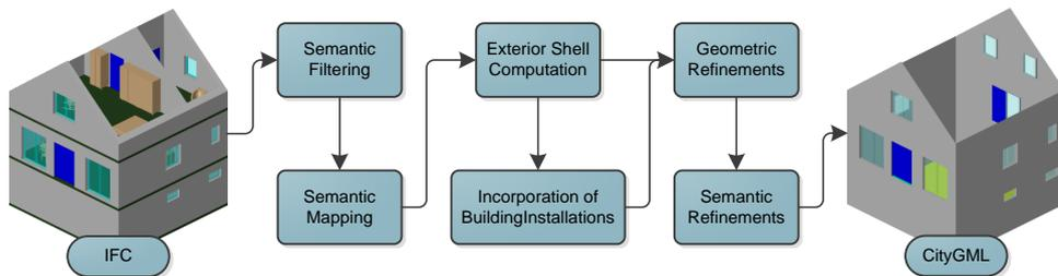
FIGURE 3.1: General workflow diagram of the conversion methodology
