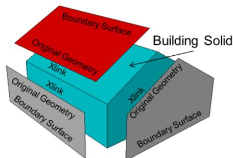
FIGURE 2.8: Linking surfaces and solids using ‘XLinks’ (Source: [36])
