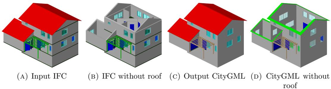
FIGURE 4.31: Niedriha input and conversion result
