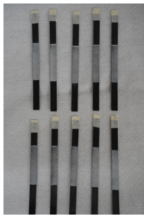
(a) 10 sections of 200mm CFRP tape with a painted speckle pattern applied
