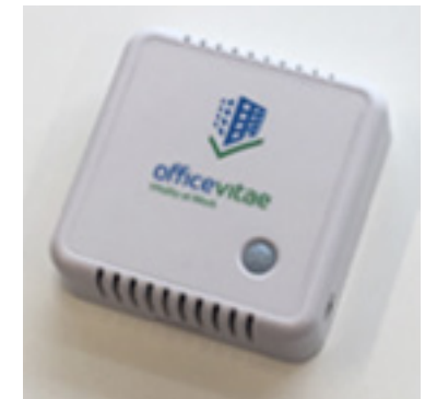
Top: OfficeVitae integrated room sensor.
