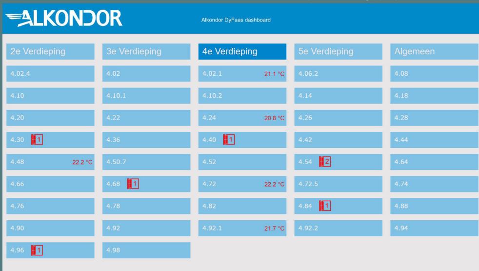
Fig 2. The status of the facade in each office room is reported. For example whether the windows are open or closed, or the sunshading active or inactive. This information can be compared against OfficeVitae's user comfort data to find patterns between negative user behaviour and negative indoor comfort or energy performance results.
