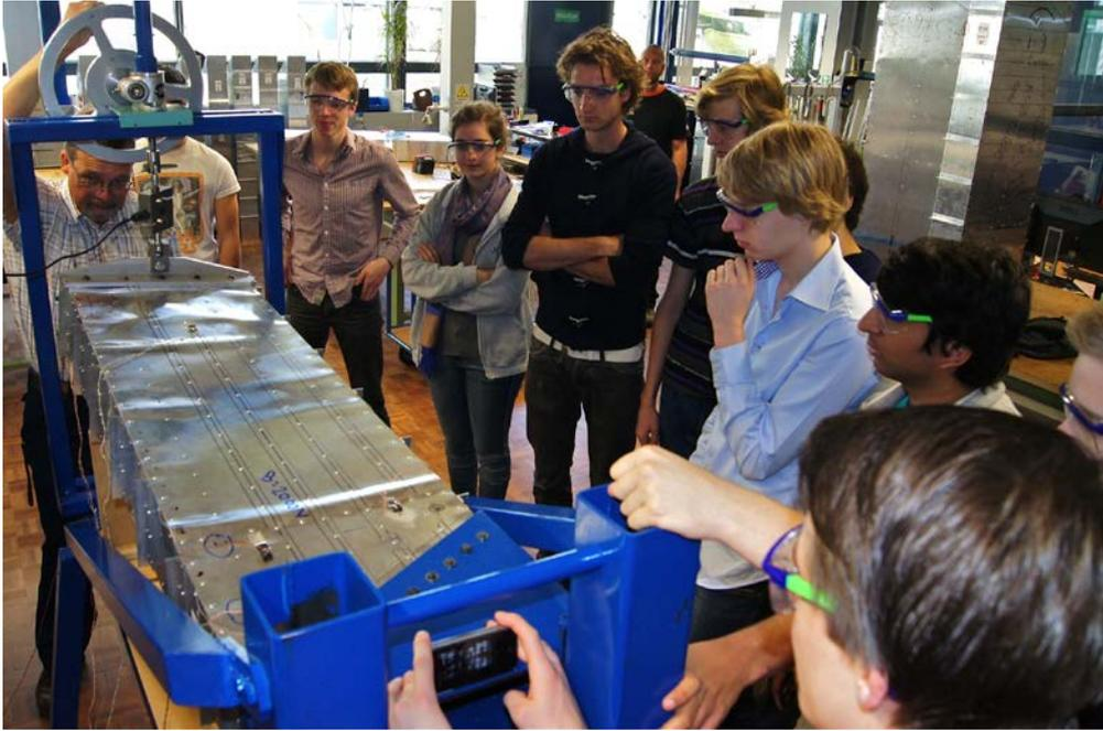
**Figure 4: The wing box in its test rig with buckling clearly visible on the top panel**
