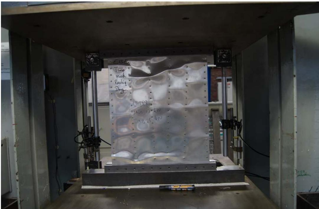
**Figure 5: the redesigned top panel in its test rig**
