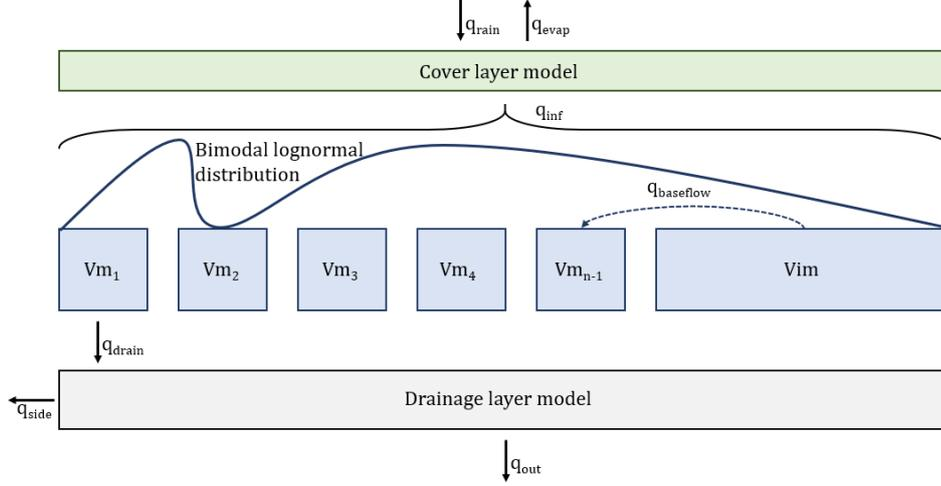
Figure 4.2: The concept of the water balance model with three layers.
