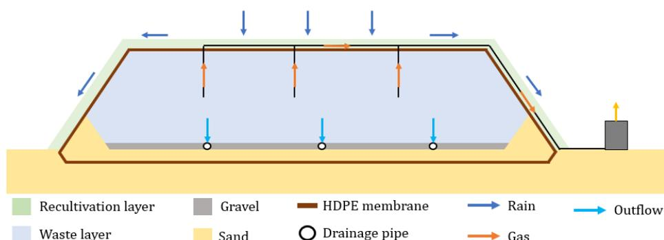
Figure 1.1: A schematisation of the structure of a modern landfill.
