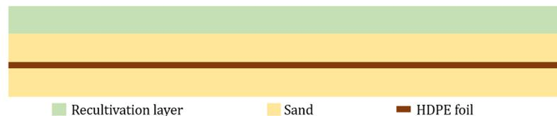
Figure 3.3: The structure of a water resistant cover layer from bottom to top: A sand layer being the foundation for the water resistant layer above it, a sand layer with rain water drainage pipes, a recultivation layer.
