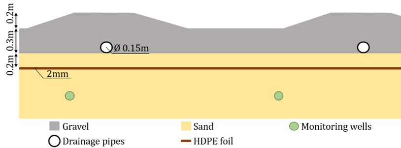
Figure 3.2: The structure of a watertight base layer from bottom to top: A layer of sand below the landfill with monitoring wells inside, the watertight HDPE membrane, a layer of sand and a layer of gravel, with leachate drainage pipes in it.
