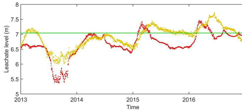
Figure 5.6: The leachate levels of compartment 3 (red) and 4 (yellow) and the dike level (green).
