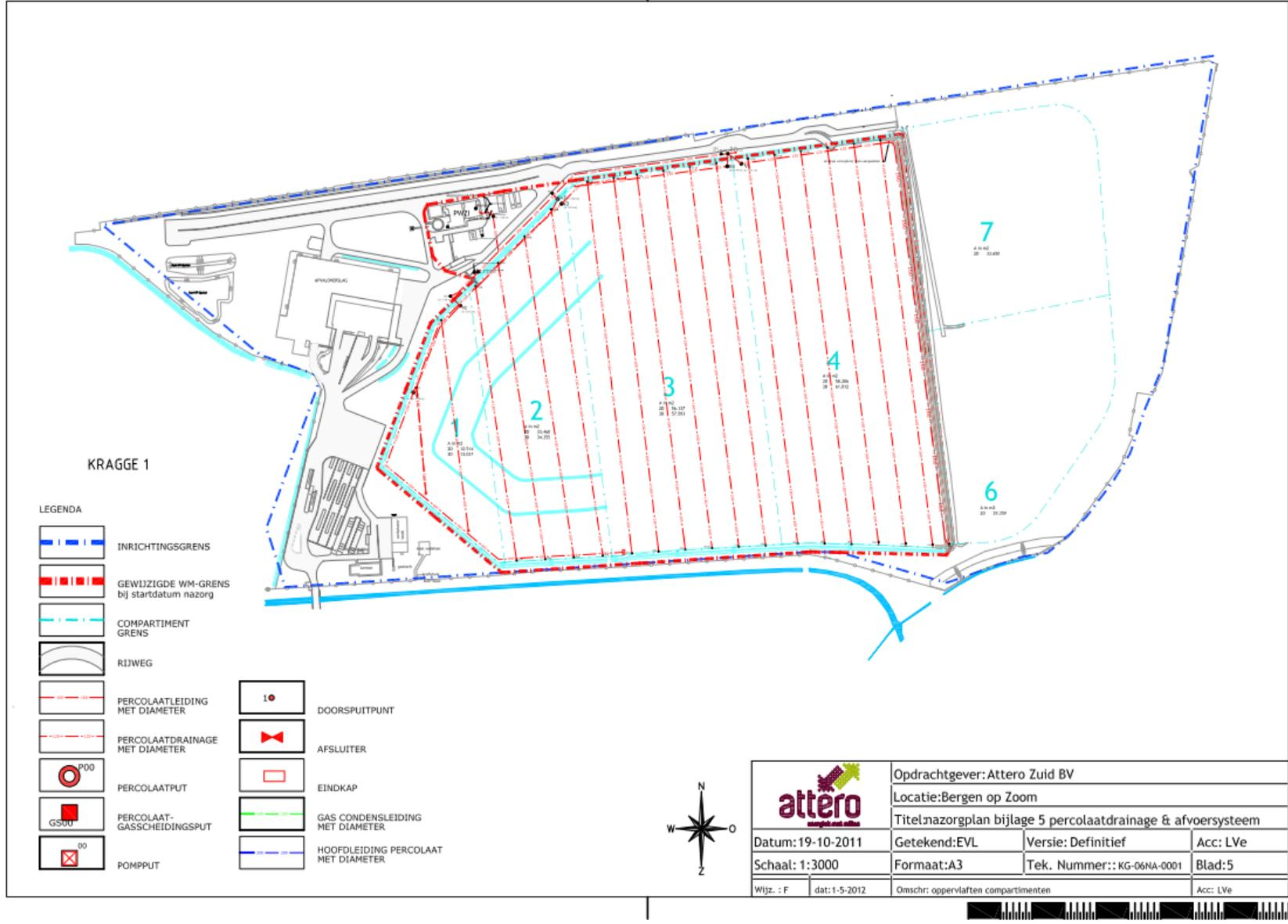
Figure A.1: Drainage system of Landfill De Kragge II.
