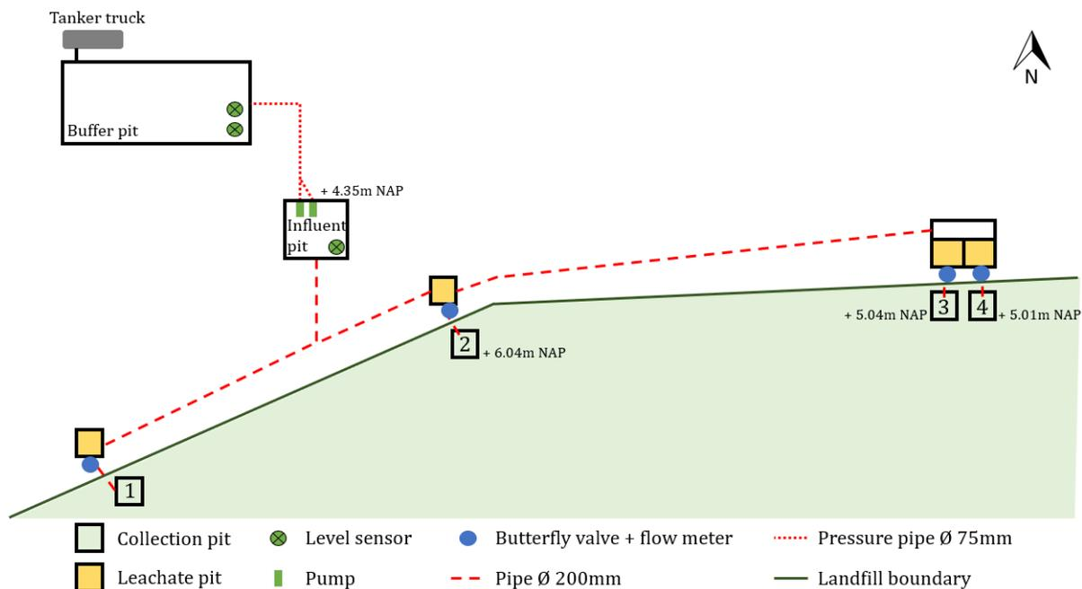
Figure 3.4: A map of the the leachate system at De Kragge II. Leachate flowing from the landfill to the truck passes multiple pits, valves and a flowmeter. Water level measurements are placed in collection pits 3 and 4.
