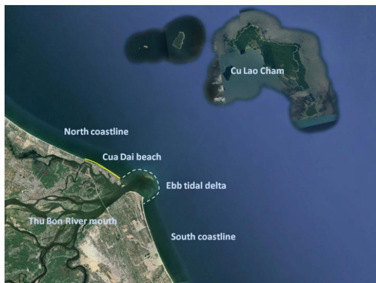
Figure 2.1: Elements of Cua Dai system
