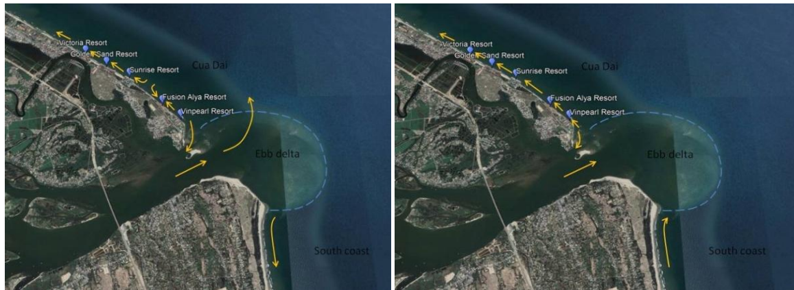
Figure 3.24: Main sediment transport patterns for ENE and SE wave conditions in the second morphological period
