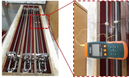
Figure 3.8 Temperature sensor to detect internal temperature variation at the core of the beam specimen during the FT test.
