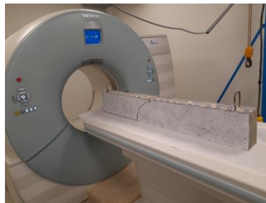
Figure 5.17 CT scanning of the ST-EB specimen.
