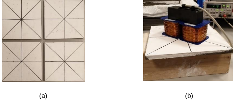
Figure 6.5 Test process to study the effect of white painting: (a) specimens painted in white; (b) inductance measurement.
