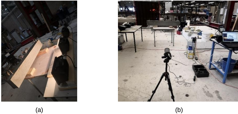
Figure 5.14 IRT test process for one of the hybrid beams: (a) Uniform heating process using three lamps; (b) Data recording during cooling process after removal of the lamps.
