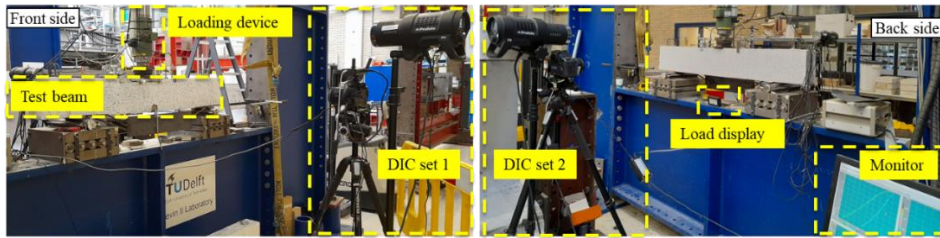
Figure 3.14 Digital image correlation on both sides of the specimens for deformation measurement.
