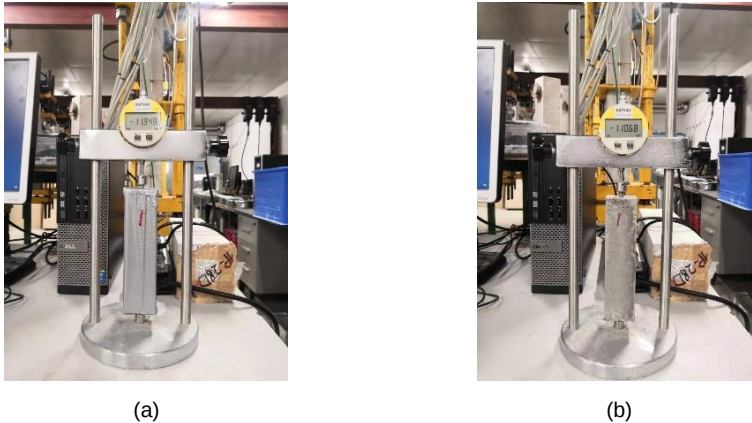
Figure 3.3 Testing set-up for autogenous and total shrinkage measurements on hardened UHPFRC: (a) autogenous shrinkage measurement; (b) total shrinkage measurement.
