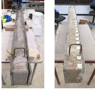
Figure 5.13 Interface debonding for one of the hybrid beams.
