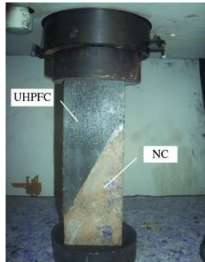
Figure 2.8 Slant shear test set-up for UHPFRC-NC specimen [78].
