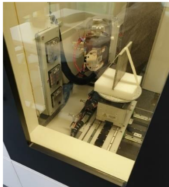
Figure 6.7 CT scanning of UHPFRC plate.
